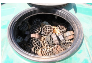
Packing material in a submerged bio-contactor – Note that the shape and size of the packing may vary with different units
