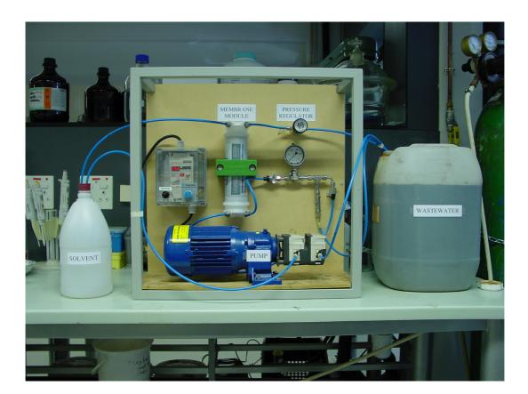
Figure 3.2: Photograph of the pilot-scale membrane extraction system
