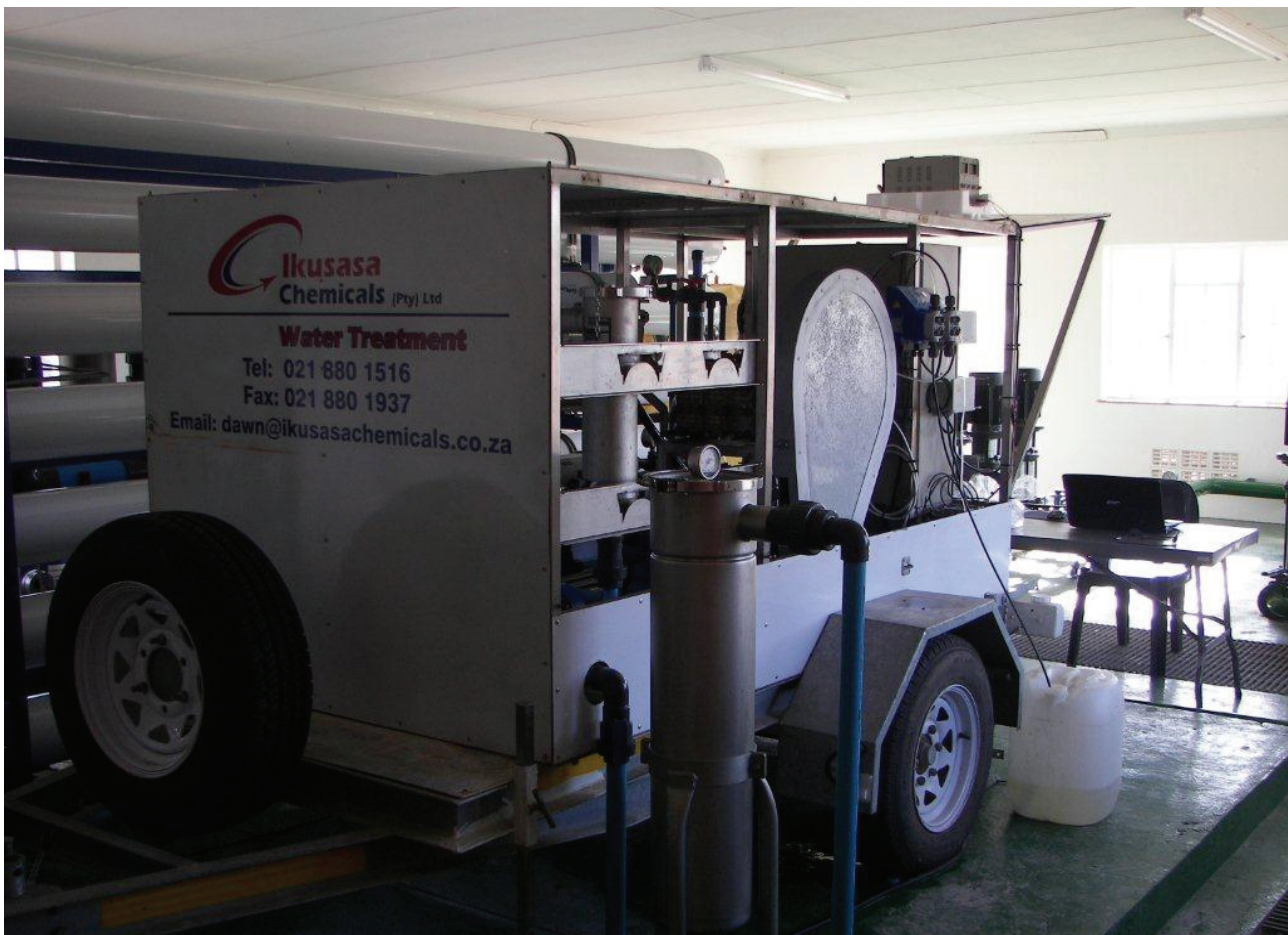
Figure 3.10: Photograph of the RO pilot plant at Bitterfontein (main plant visible at the back)
