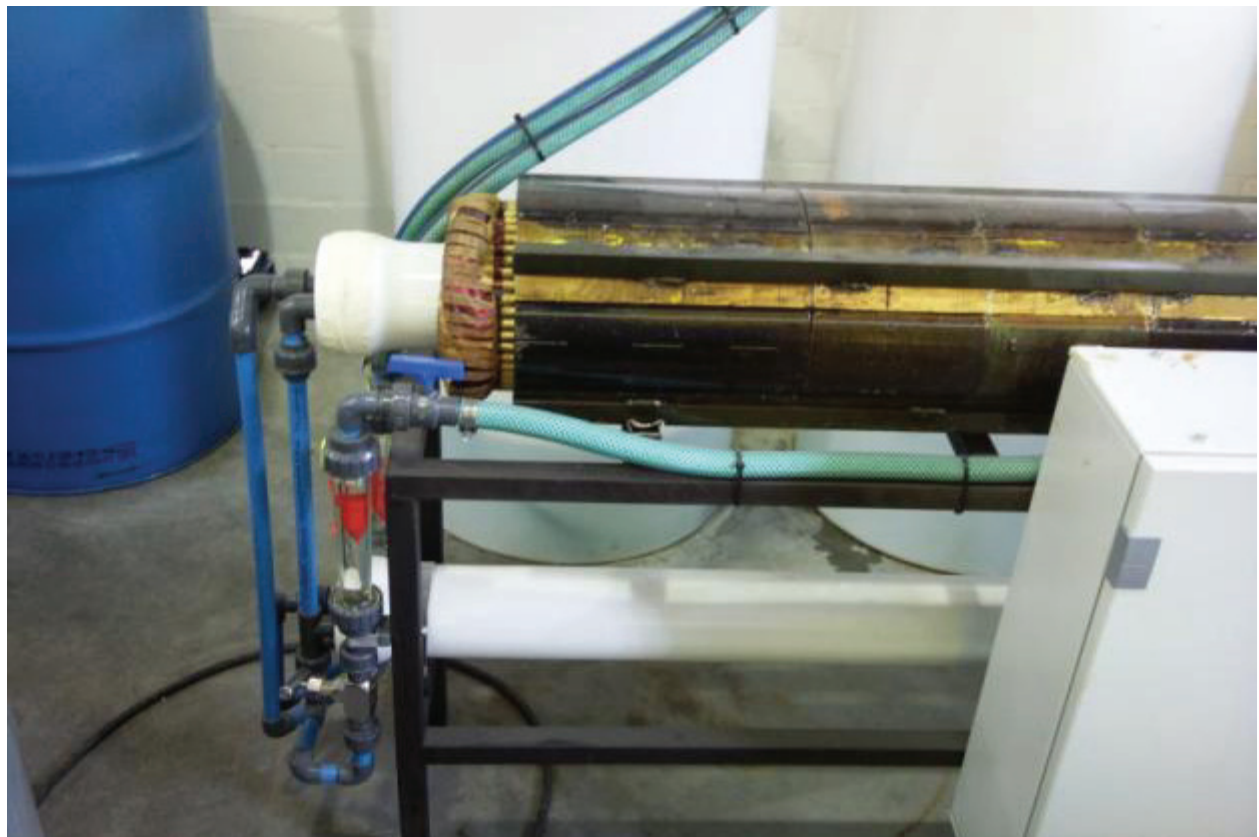
Figure 4.2: Photograph of the stator coil used in the RO plant at Ikusasa factory
