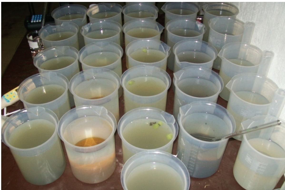
Figure 16: Turbidity reductions by the tested flocculants.
