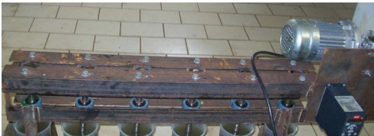
Figure 14: A 6 Place Jar stirrer with VSD for speed control
