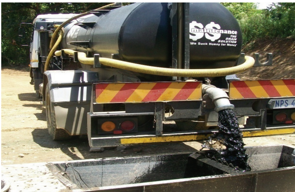
Figure 10: Sewage being trucked in to the Melville WWTWs
