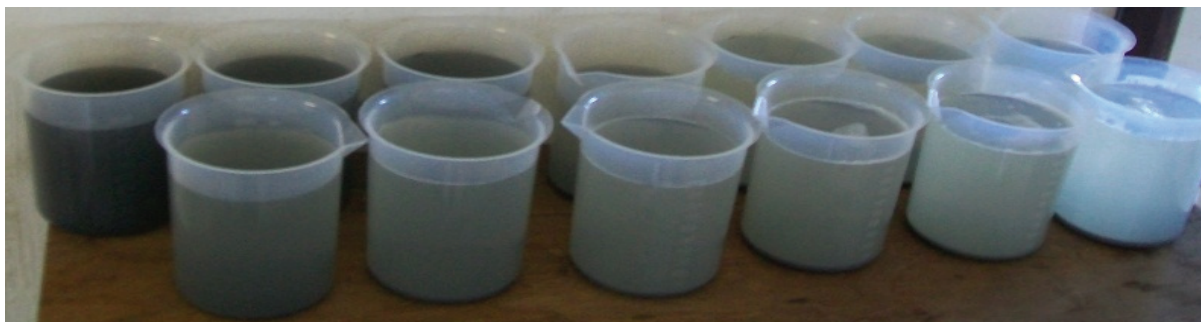
Figure 15: Settled water from Moringa flocculation (in the back) and Ferric (in the front).
