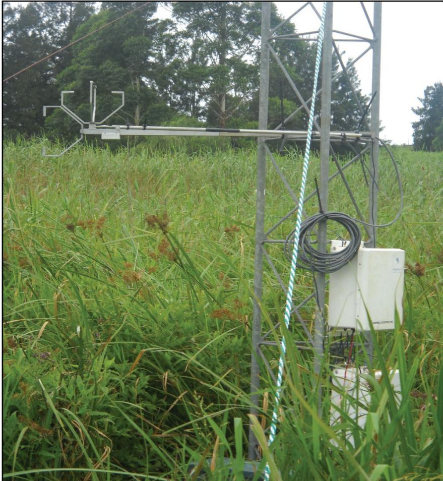
Figure 4.2. An Applied Technologies, Inc. (ATI) sonic anemometer mounted on a lattice mast above the sedge.
