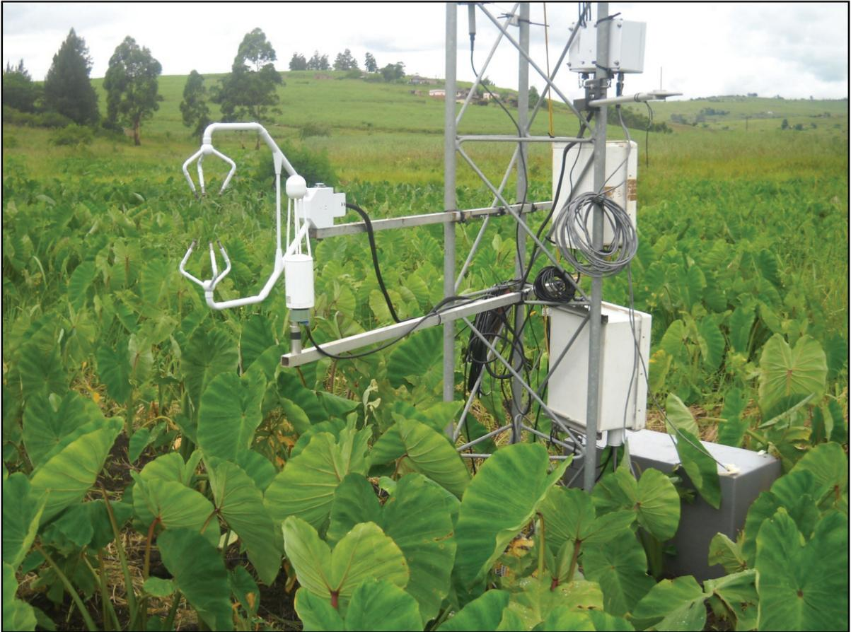
Figure 4.1. An extended open path (CSAT 3) eddy covariance system installed on a lattice mast above the madumbe canopy.
