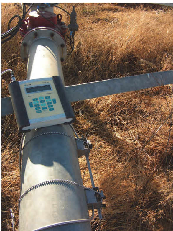
Figure 22 Portable acoustic measuring devices for pipes (left) and canals (right)
