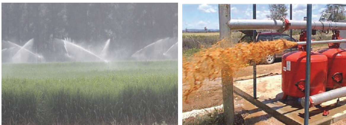
Figure 7 In-field losses such as spray evaporation and backwash water affect efficiency
