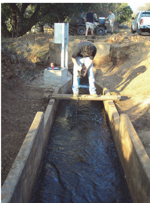
Figure 22 Portable acoustic measuring devices for pipes (left) and canals (right)
