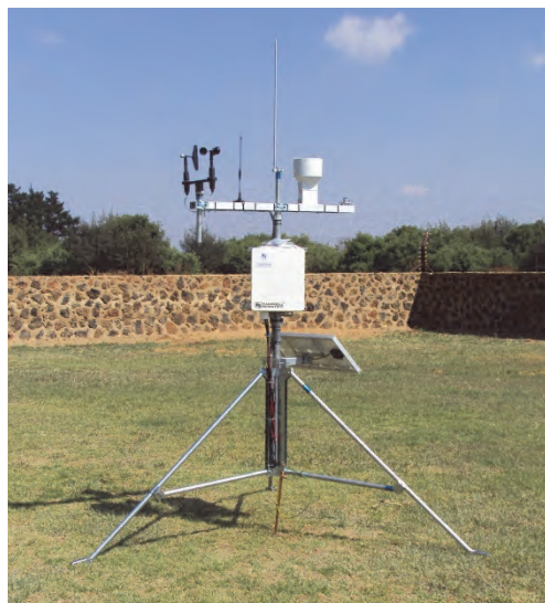
Figure 24 Example of an automatic weather station for climatic data collection
