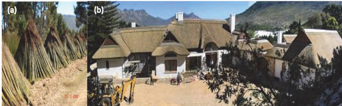
Figure 6: Thamnochortus insignis cut in the growing season and not sun-dried for at least 7 days before bundling & (b) Finished product, thatched guest lodge.
