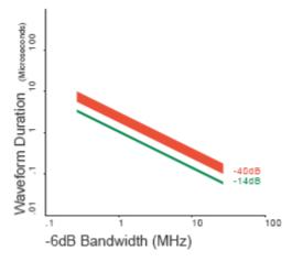
Figure 6 - Waveform duration to bandwidth
