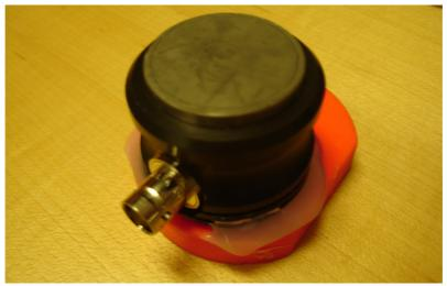
Figure 25 - Shear wave transducer
