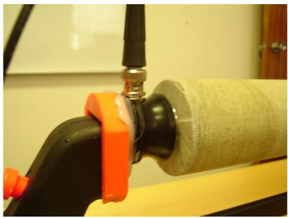
Figure 23 - Transducer fitting
