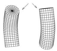
Figure 8 - Flexural class mode (Zadler et al., 2004).
