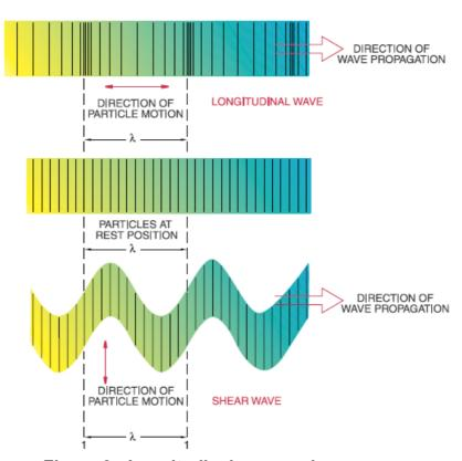
Figure 3 - Longitudinal versus shear waves
