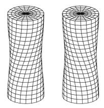
Figure 9 - Torsional class mode (Zadler et al., 2004).
