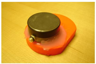
Figure 26 - Compressional wave transducer
