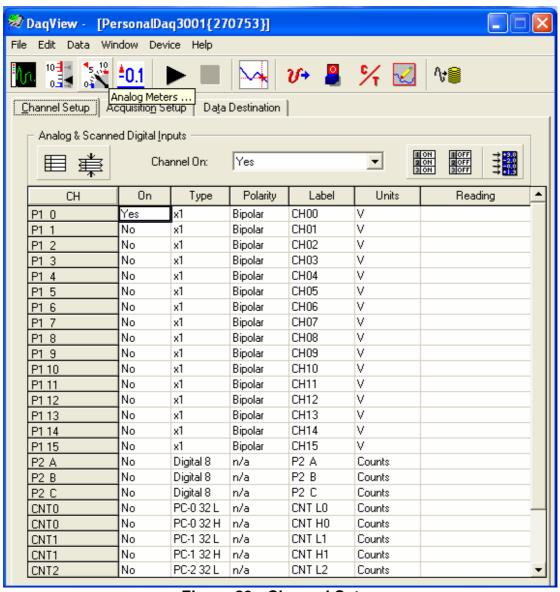
Figure 29 - Channel Setup
