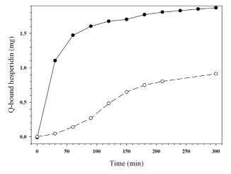
**Figure 2.3:** The adsorption of the model flavonoid hesperidin to two food-grade Amberlite<sup>®</sup> resins was tested. ( $\circ$ ) XAD4 displayed slower adsorption kinetics and lower load capacity than (•) XAD7HP. The XAD7HP adsorbed nearly all the hesperidin in solution and was able to bind even more once placed in a fresh solution, giving it a load capacity of more than twice that of XAD4.
