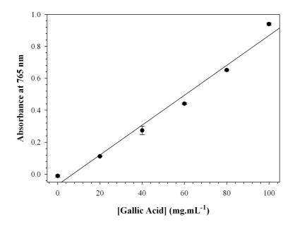
**Figure A3:** Gallic acid standard curve for total phenol determination shows a linear response in the range of 0-100 mg/L gallic acid. Gallic acid is a typical plant polyphenol that can be used for estimating total phenol content of plant extracts expressed as gallic acid equivalents (GAE).
