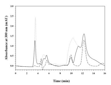
**Figure 2.4:** HPLC analysis profiles of samples from the Amberlite<sup>®</sup> XAD7HP batch adsorption process. (—) Represents the chromatogram of the flavonoid-rich solution prior to the solid-phase recovery study. (…) Represents the chromatogram of the flavonoid-rich solution retained after the adsorption process. The chromatogram represented by (– –) is from elution step where ethanol was used to remove flavonoids from the resin.
