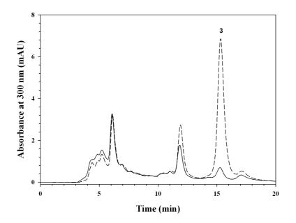
**Figure 2.6:** Typical HPLC chromatograms of (—) water and (– –) methanol extracts of orange pulp. Hesperidin (3) elutes at approximately 15.5 min. Other major peaks are observed at approximately 6 and 12 min respectively.
