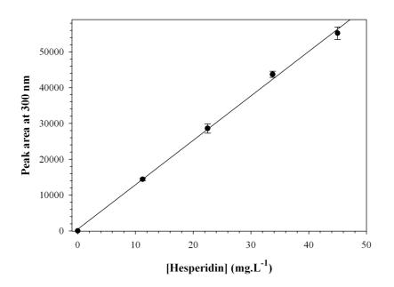
**Figure A2:** HPLC hesperidin standard curve shows a linear response in the range of 0-45 mg/L. The upper concentration is also close to the saturation point in a water solution.
