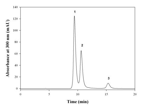
**Figure 2.2:** The HPLC method allowed separation of (1) *p*-coumaric acid, (2) ferulic acid and (3) hesperidin and would also resolve naringin and narirutin from hesperidin.
