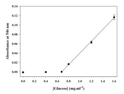
**Figure A1:** Glucose standard curve with DNS assay shows a linear response in the range of 0.7-1.6 mg/mL glucose. The lack of linearity in the lower range is the result of oxygen in the sample, destroying the glucose under alkaline conditions.
