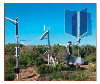
The Whirly enables the collection of fog even during near windless conditions.
