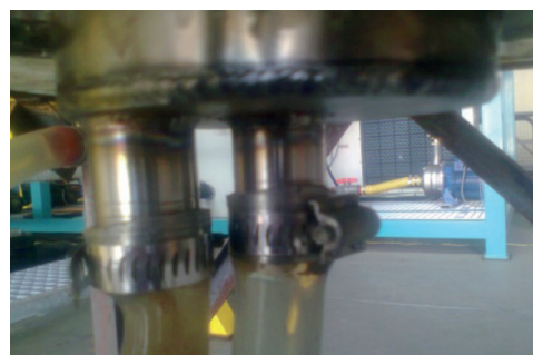
Figure 3 Feed water inlet and outlet for the gravitation HybridICE filter
