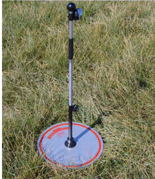
Figure 9: The Ellinbank rising plate meter used in the trial to measure the available dry matter.
