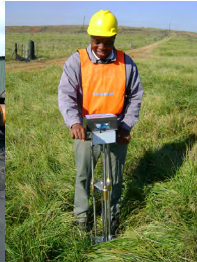
Figure 16: The handheld penetrometer used during the trial to measure the compaction on the pivot.
