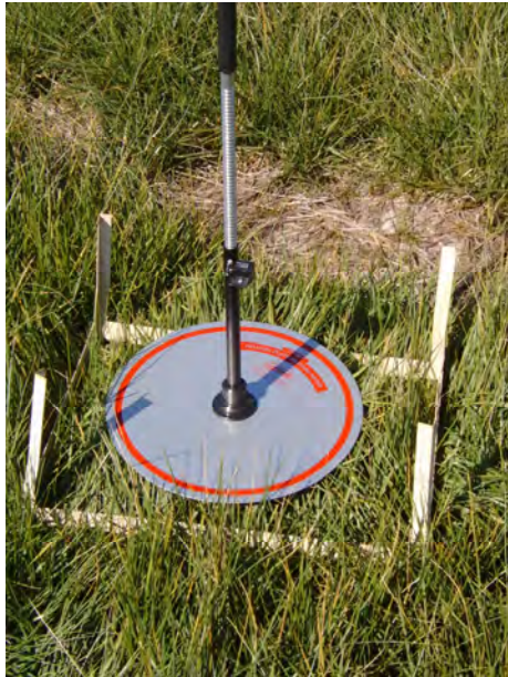
Figure 10: Calibrating the Ellinbank rising plate meter by measuring the pasture height in the quadrant and then clipping the utilizable dry material in the quadrant (Figure 11) and weighing it.
