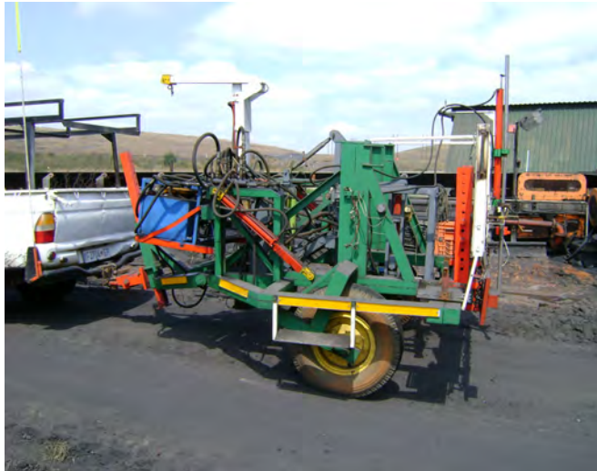
Figure 15: The hydraulic penetrometer used during the trial to measure the compaction on the pivot.
