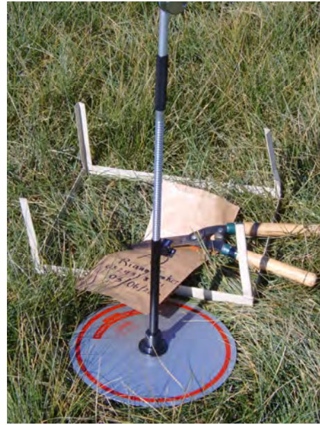
Figure 11: Calibrating the Ellinbank rising plate meter, using the following equipment by measuring the pasture height in the quadrant and then clipping the utilizable dry material in the quadrant and weighing it.
