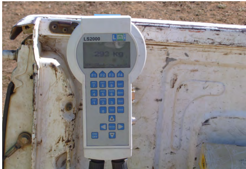
Figure 7: The LS2000 electronic scale which was linked to the scale showed in Figure 6, to accurately obtain the animal weights.
