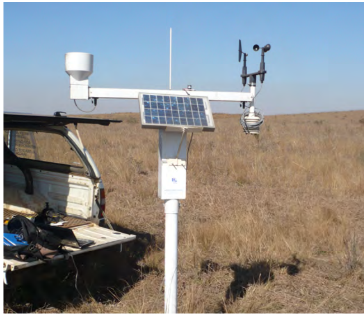
Figure 3: One of the two weather stations used to capture climatic data.
