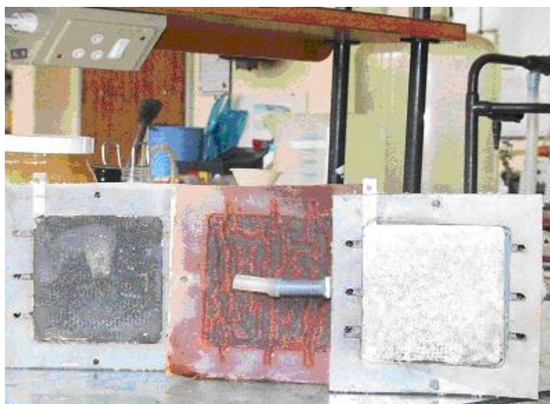
Figure 2.3.(2): Electrolytic cell for dissociation of water on laboratory scale (electrodes on sides and membrane in centre)
