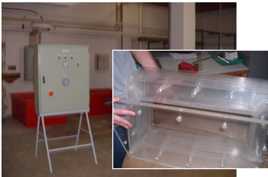
Figure 2.3.(3): The electrochemical cell and power supply unit built on pilot plant scale for dissociation of water
