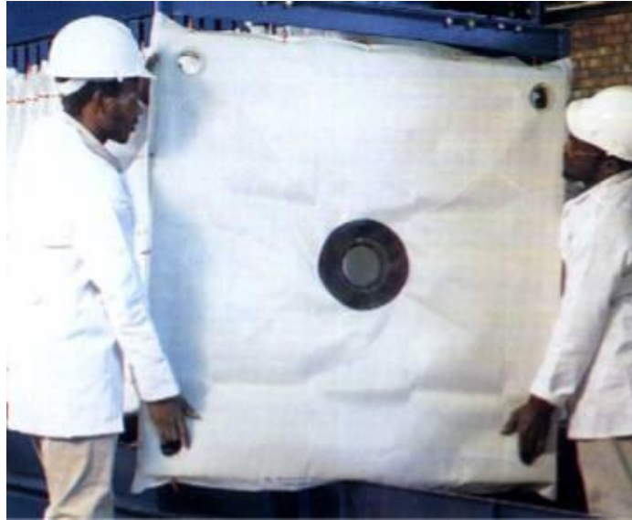
Figure 25 - Filter Cloth on Filter Press Plate
