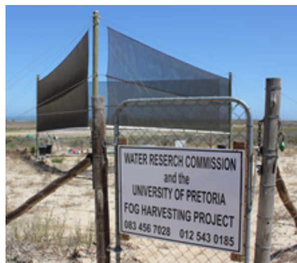
The triangular fog water collection system.
