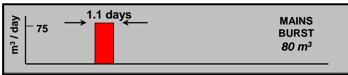
Figure 2.3 : Typical duration and losses from a mains burst
