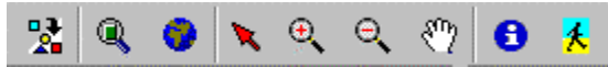
Figure 7.7: Toolbar buttons (properties, layer extent, full extent, pointer, zoom in, zoom out, pan, information, photograph)
