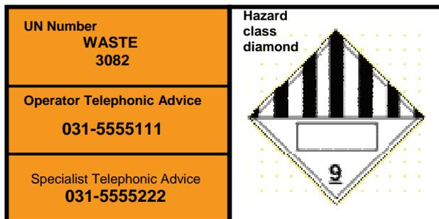
The vehicle carrying the wastes must display three of these placards: One on either side of the vehicle and one at the back. A truck and trailer combination with a waste container on the truck and containers on the trailer must display six placards in total.
