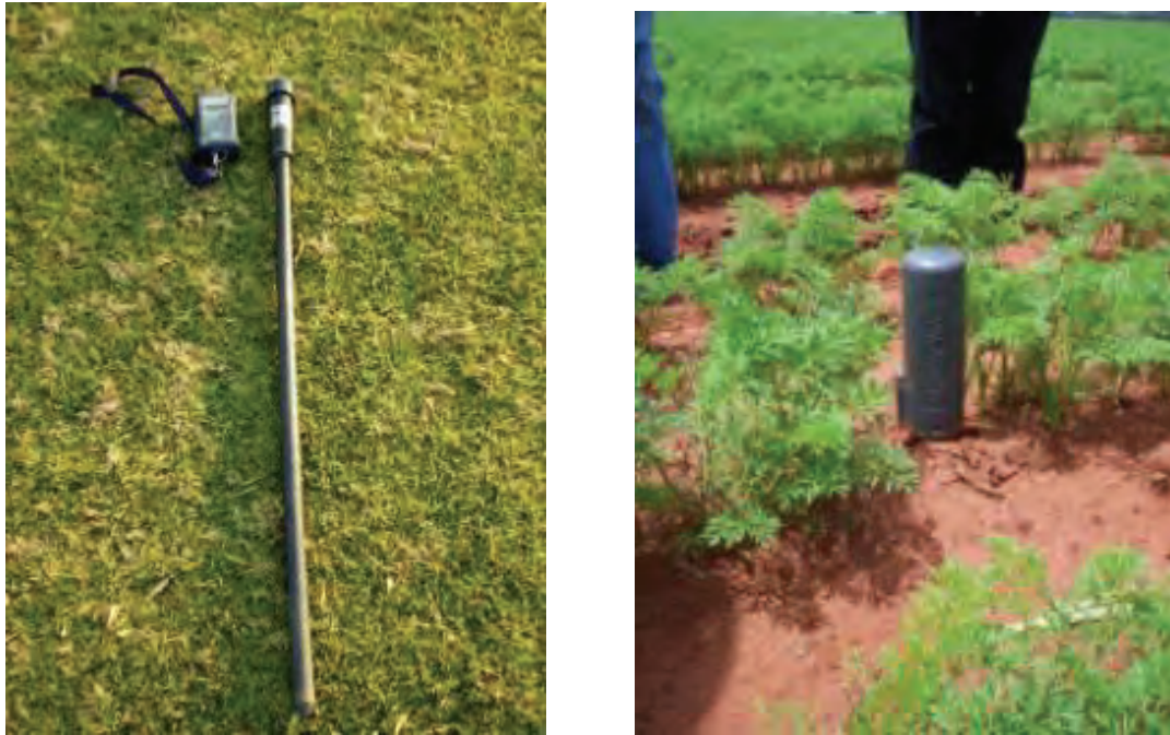
Figure 9: Examples of the capacitance probes that were used to monitor soil water content
