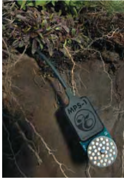
Figure 59: Illustration of the new Dielectric MPS-1 Water Potential Sensor (Decagon, 2008).
