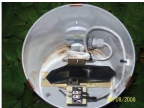
Figure 10: Tipping bucket rain gauge used to monitor irrigation amounts for the centre pivots.
