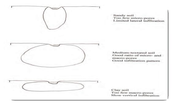
Figure 4: Water infiltration from shallow (non-ridged) furrow in different soils
