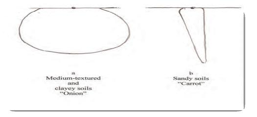
Figure 3. Water infiltration under drip irrigation
