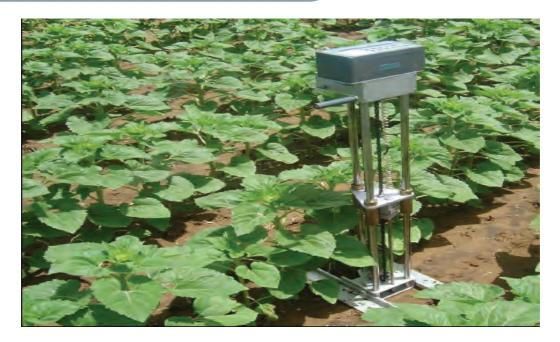
Figure 2. Penetrometer used for determination of soil compaction
