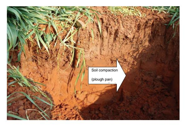
Figure 3. Plough pan soil compaction (Source: D Haarhoff)
