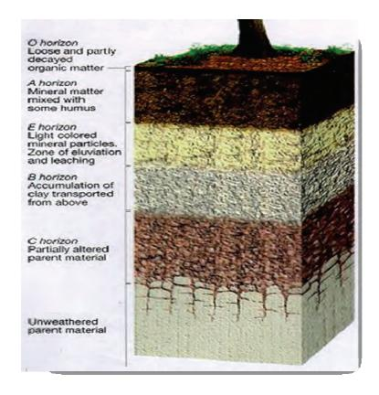
Figure 3. Example of a diagnostic soil profile with various soil horizons
