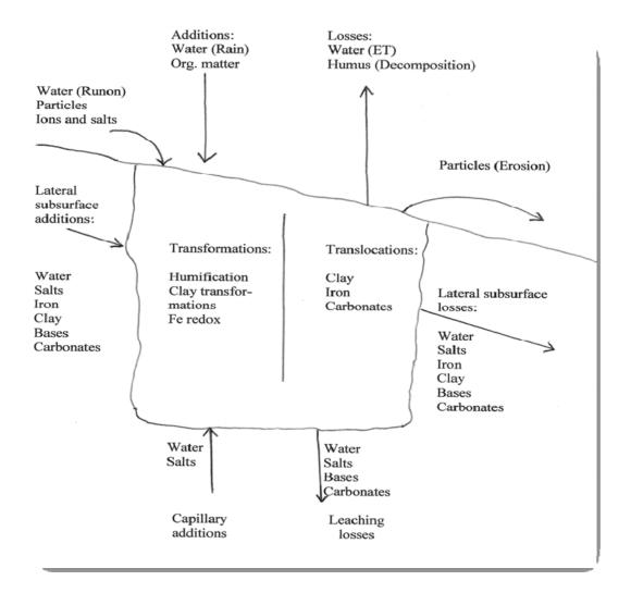
Figure 1. Schematic illustration of soil forming
