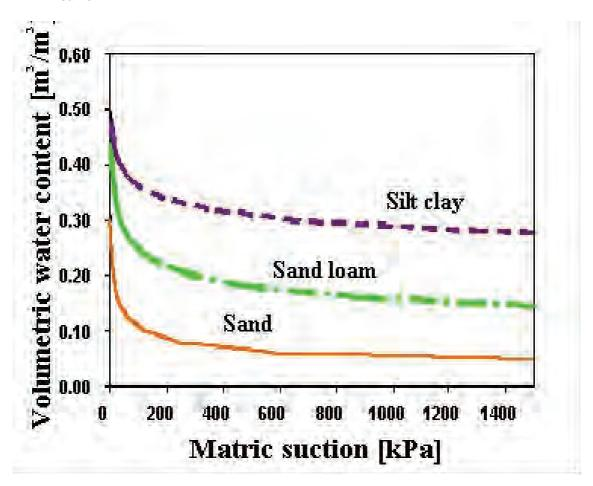
Figure 2. Soil water retention curve for different soil types
