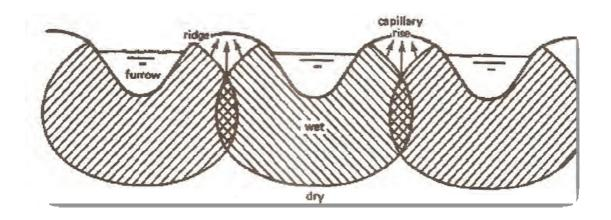
Figure 5. Ideal wetting pattern in deep furrow irrigation with ridge<sup>2</sup>
