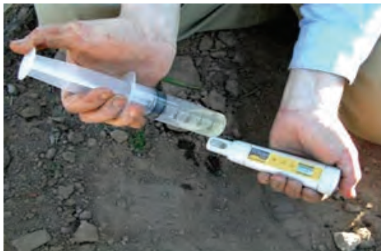
Figure 2. Pocket size pH meter
