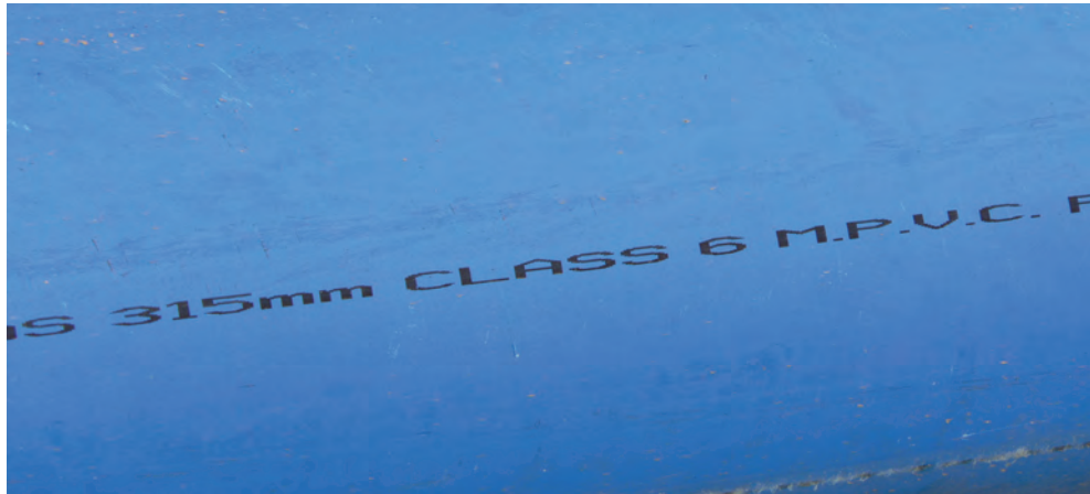
Figure 31. Script on PVC pipe – 315 mm (outside diameter) class 6 (pressure capacity of 6 Bar)
