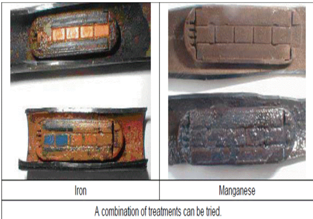
Figure 4. Filter rings blocked by sediments due to high manganese and organic content 8)
