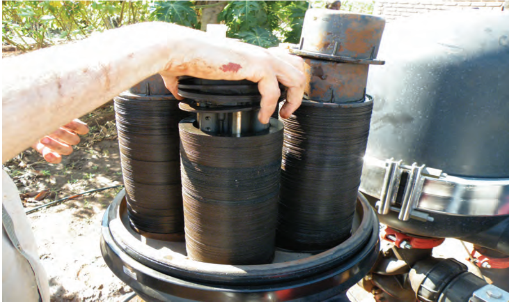
Figure 26. Disc elements of filter unit (100 micron filtration size)
