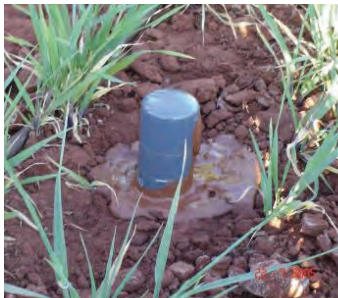
Figure 8. C Probe installed 6)
