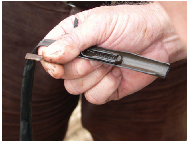
Figure 17. Cut open drip pipe
