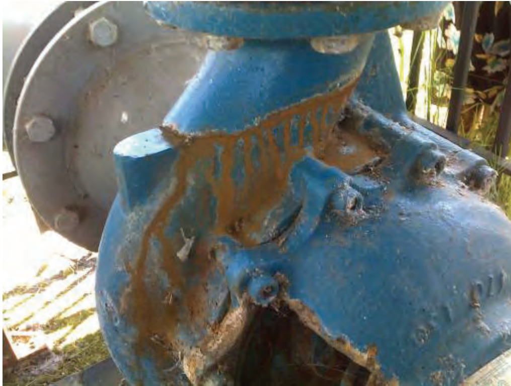
Figure 35: Cracked pump casing
