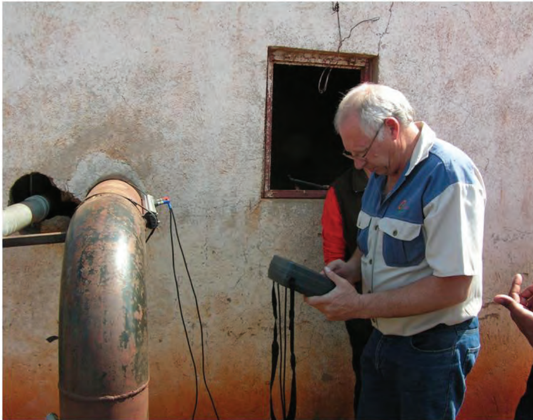
Figure 29: Using a clamp-on ultrasonic meter to evaluate mechanical meters at the Orange-Riet Scheme
