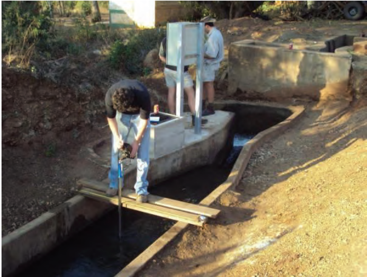
Figure 23: Using the FlowTracker at the inlet of the secondary canal.
