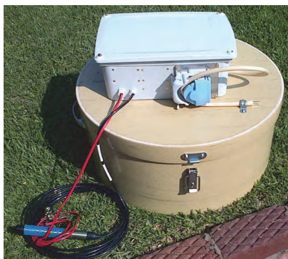
Figure 4.3: ALCO 20-bottle sequential sampler built by the Centre for Water Resources Research at the University of KwaZulu-Natal.
