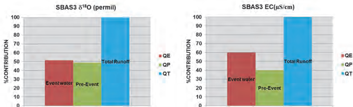
Figure 6.21: Percentage contribution of event and pre-event water to total runoff using \delta^{18}\text{O} and EC as tracers for the event of 20 February 2013 at Southern Basalts study site.
