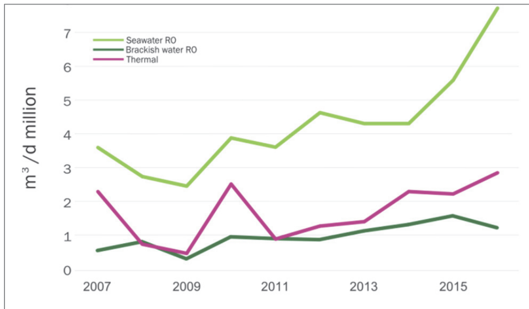
Figure 2.7: Thermal versus membrane technology by annual contracted capacity (GWI, 2011)
