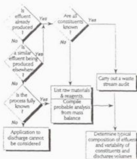
Figure 10 Flow diagram showing the procedure to determine the composition and variability of effluent quality
