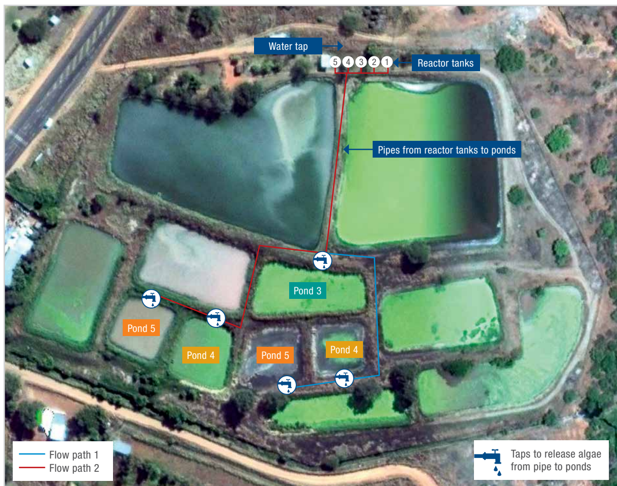
Figure 10: Layout of the ponds at the Motetema Wastewater Treatment Works, indicating the piping from the reactor tanks and the ponds to be dosed
