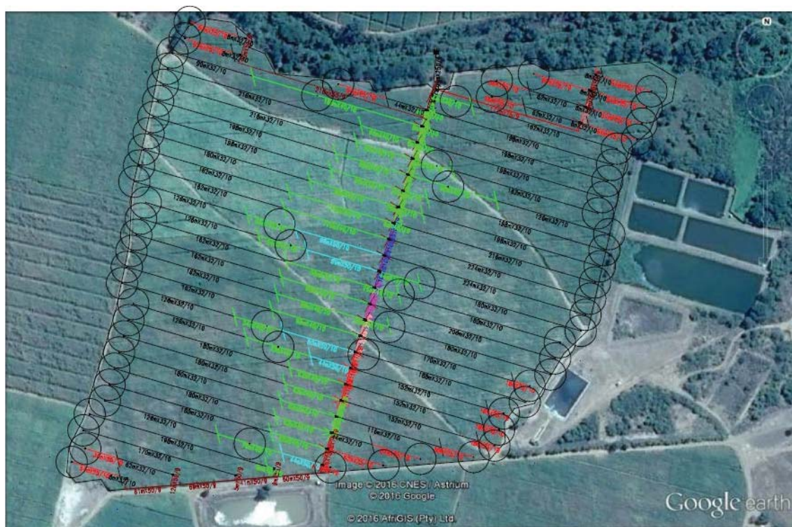
Figure 5. 6: Lay-out of the sprinkler irrigation system
