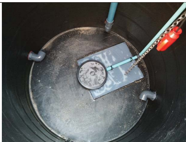
inside of bioreactor - sparger and level probe
