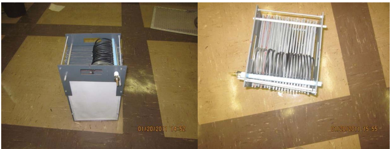
Figure 4: Final membrane pack showing side view (left) and top view (right)
