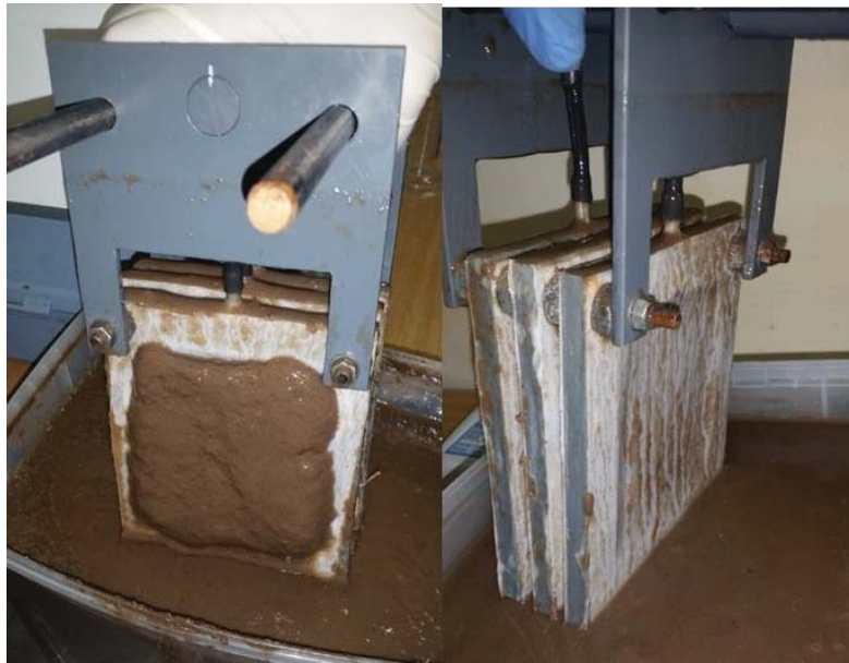
Figure 46: Membranes after no-scour runs (left) and continuous air scour (right)
