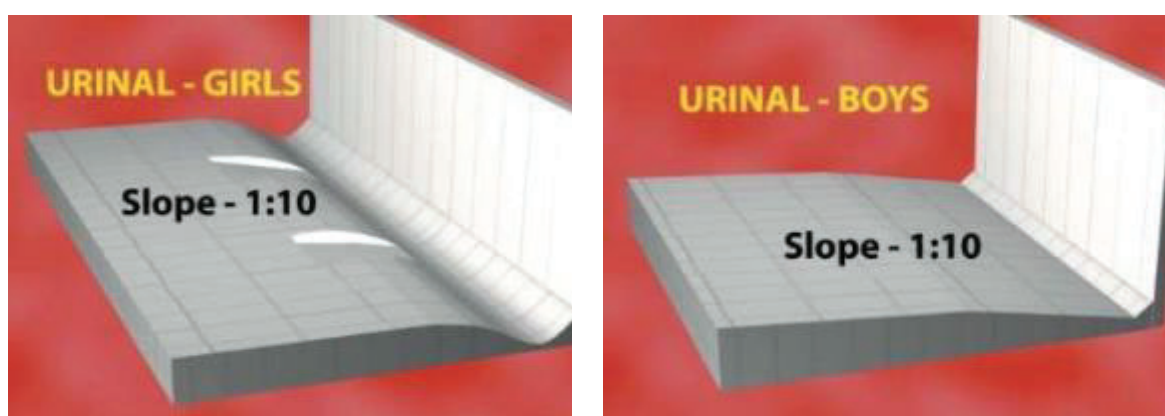
Figure 20: Designs for girls' and boys' urinals recommended by the Government of India
