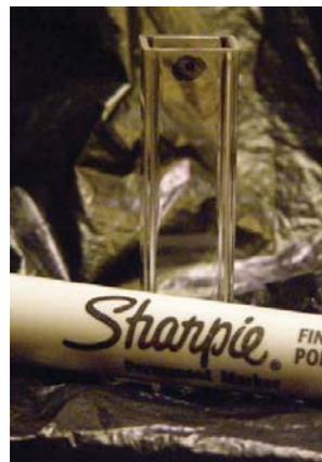
**Fig D3.2: Disposable polymethacrylate cuvette**   **Fig D3.3: Cuvette labeled for positioning**
