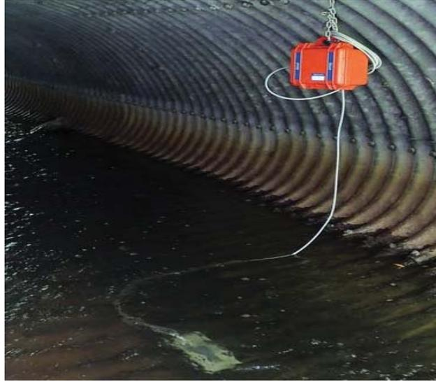
**Figure 4-5: Greyline MantaRay Portable Area Velocity Flow Meter**
