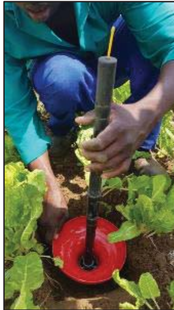
Figure 4-10: Installation of wetting front detectors (Stevens & Stirzaker, 2010) within the root zone of winter vegetable crops at the study schools.
