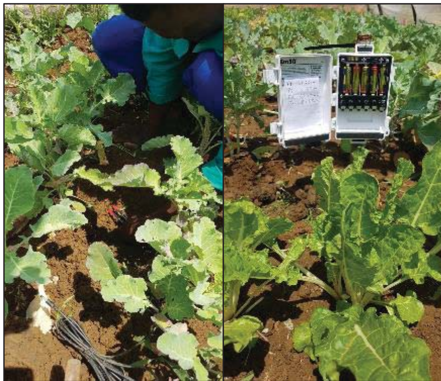
Figure 4-9: 10-HS automatic soil water sensors installed within the root zone of winter vegetable crops at the study schools.
