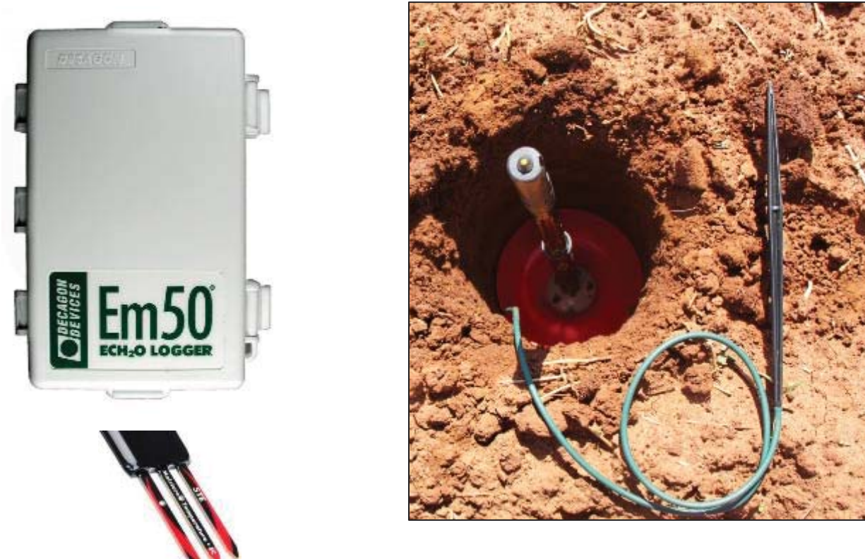
Figure 3-5: Illustration of wetting front detector (WFD) and ECH2O 5TE soil moisture sensor.
