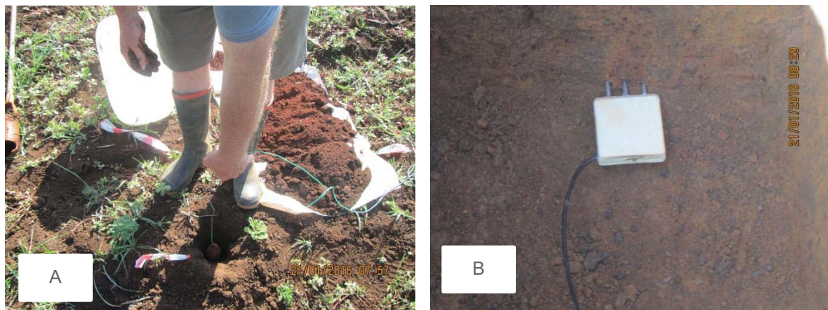
Photograph 5.5 Installation of Watermark sensors (A) and TDR sensors (B) at OSCA, Empangeni.
