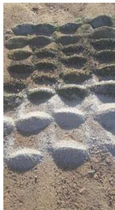
Figure 12 (Right): Core samples taken during the drilling process. These pictures were sent to Mr Vonk to determine whether drilling should continue or stop, based on the structure and consistency of these samples.
