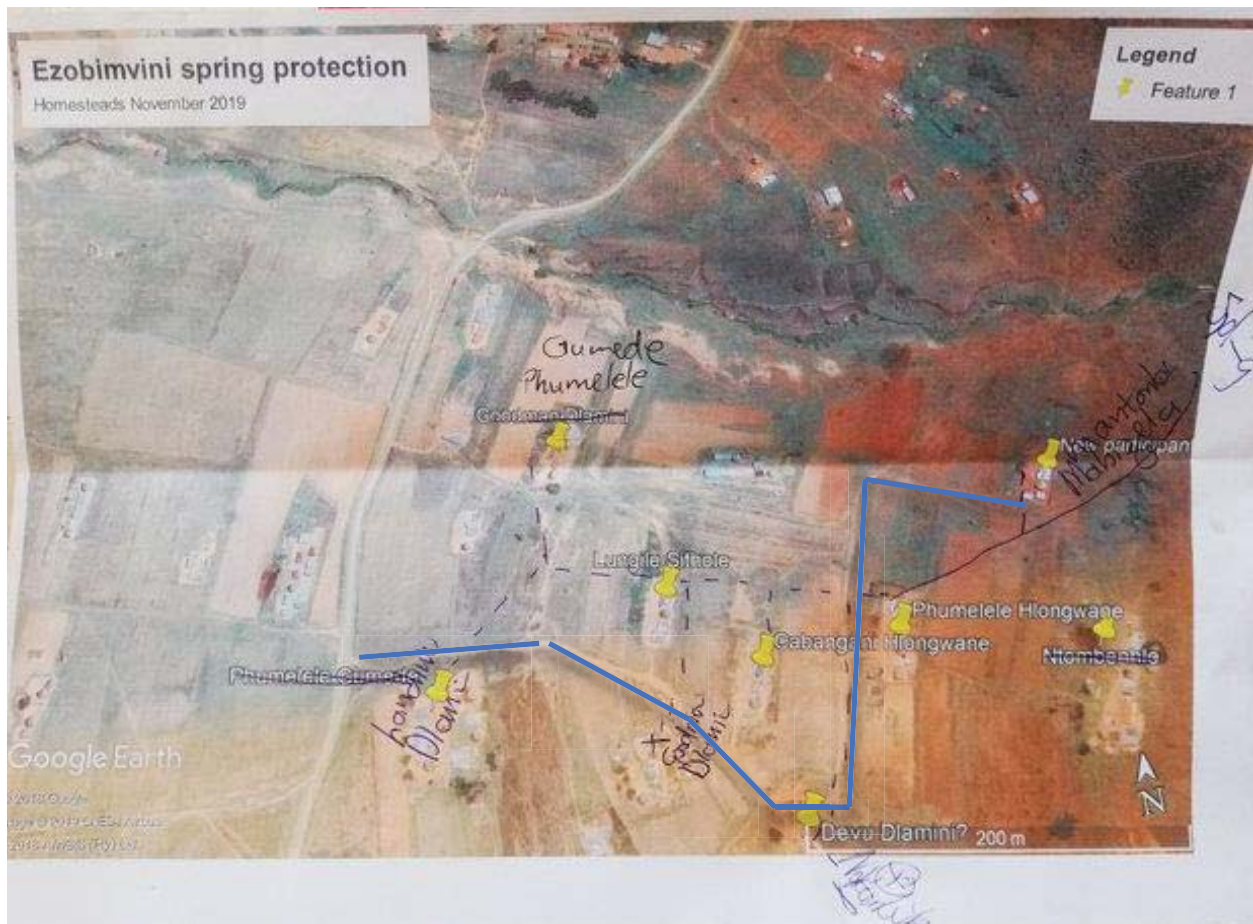
Figure 6: Creating a Google Earth map from GPS coordinates using cell phones is not very accurate, so a correction was made. The blue line indicates the main feeder pipe to participants' homesteads running along the small road to Phumelele Hlongwane's homestead.
