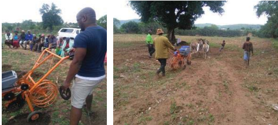
Figure 2. Left: Introducing the Knapick planter to the learning group and demonstrating the changing of seed plates. Right: The oxen-drawn planter has been hitched to a team of donkeys for planting.
