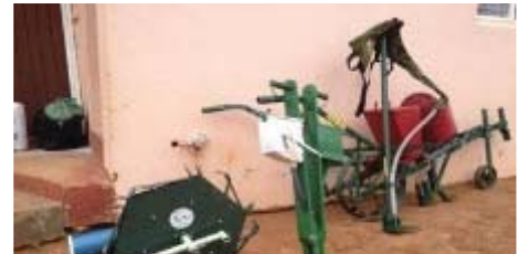
Different planters; Mbli (hoe-type hand), Haraka (Wheel), Matracca (jab) and animal drawn planters, (Knapik – below)
