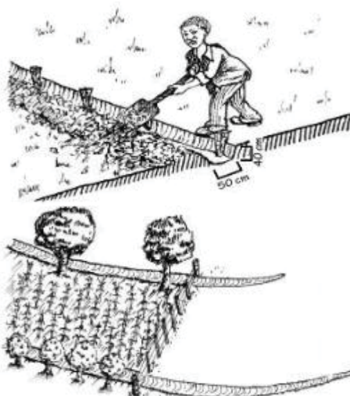
Constructing a swale and a view of two swales indicating the flow of water
