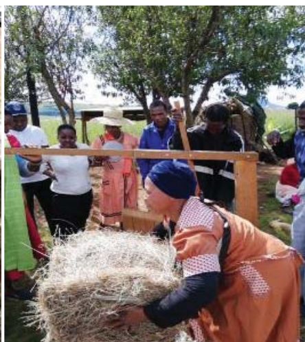
Hand operated baler, with a bale of veld grass made with this baler
