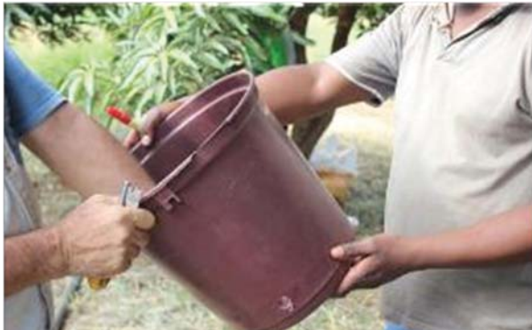
A small hole is made at the bottom of the 20 L bucket to connect the elbow connector and the down pipe
