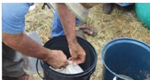
Sand placed in a closed muslin bag on-top of the gravel, to avoid sand being washed into the dripper lines
