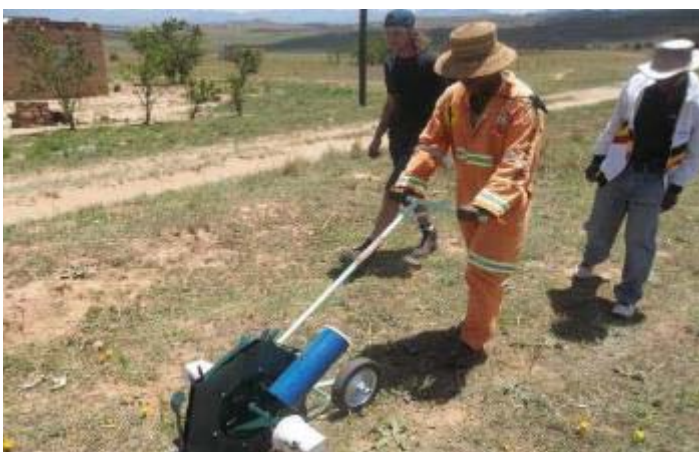
Using a Haraka wheel planter – this planter can “plant” a range of different seeds, but does not allow for fertilizer placement at the same time
