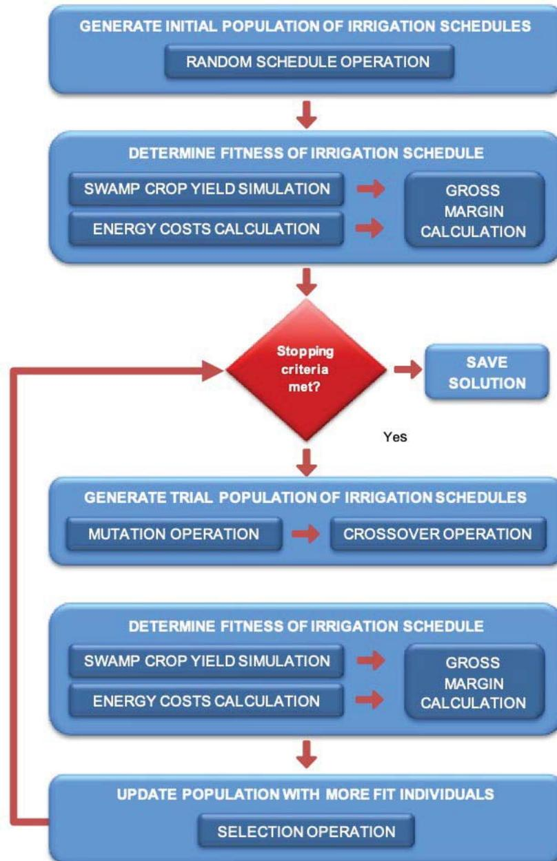
Figure 6.1 Flow chart of differential evolution optimisation procedure.
