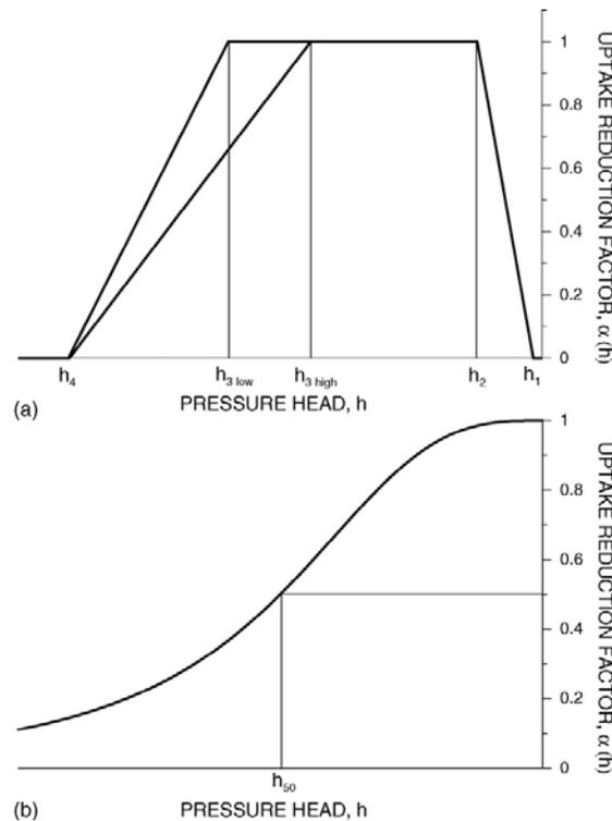
**Figure 4.4** Piecewise linear (a) and alternative S-shaped (b) water-stress uptake reduction functions of Feddes et al. (1978) and van Genuchten (1987) as described in Skaggs et al. (2006).
