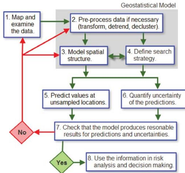
**Figure 4.2** Generalised workflow for geostatistical studies as recommended by the geostatistical analyst toolkit of the ArcGIS 10.4 software suit (Esri).
