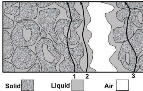
**Figure 4.5** Snapshot of a schematic illustration of the three conductance pathways for the apparent soil electrical conductivity measurements (obtained from Corwin and Scudiero, 2016, modified from Rhoades et al., 1989). Pathway 1 = solid-liquid conductance, Pathway 2 = liquid conductance and Pathway 3 = solid conductance.
