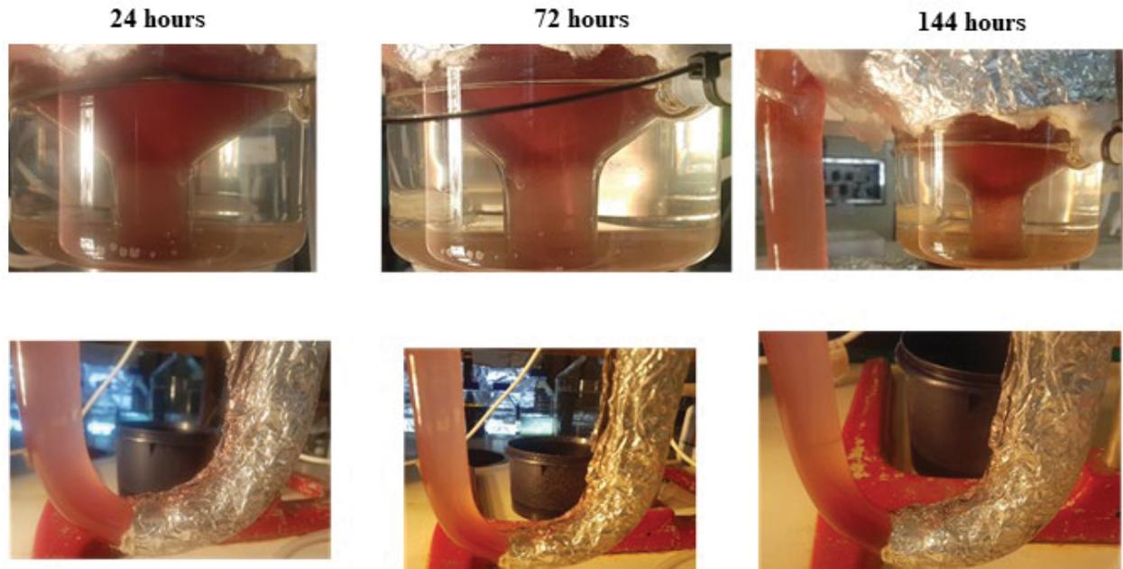
Figure 32 : Photograph of cooling and down-comer sections of the TPBR showing regions of deep purple coloration signifying biomass settling.
