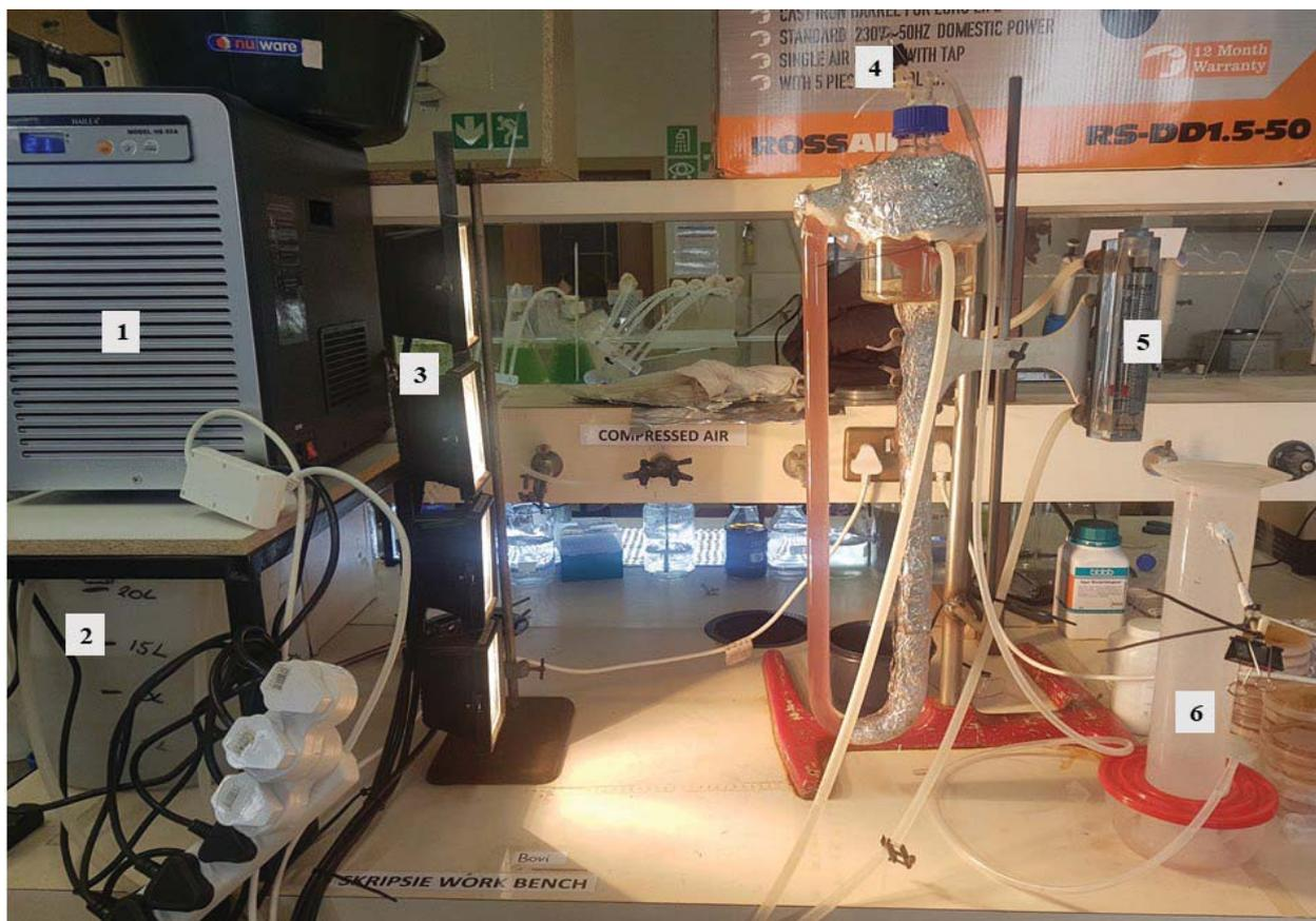
Figure 24: Photograph of the TPBR during biological hydrogen production with the annotated number (1-6) corresponding to water chiller, reservoir, halogen light panel, sample port, water flowmeter and hydrogen collection unit respectively.
