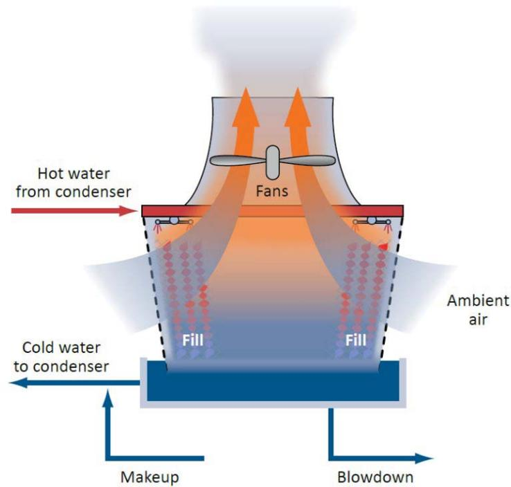
Figure 3: Water flow in a wet cooling tower (Bushart, 2014)
