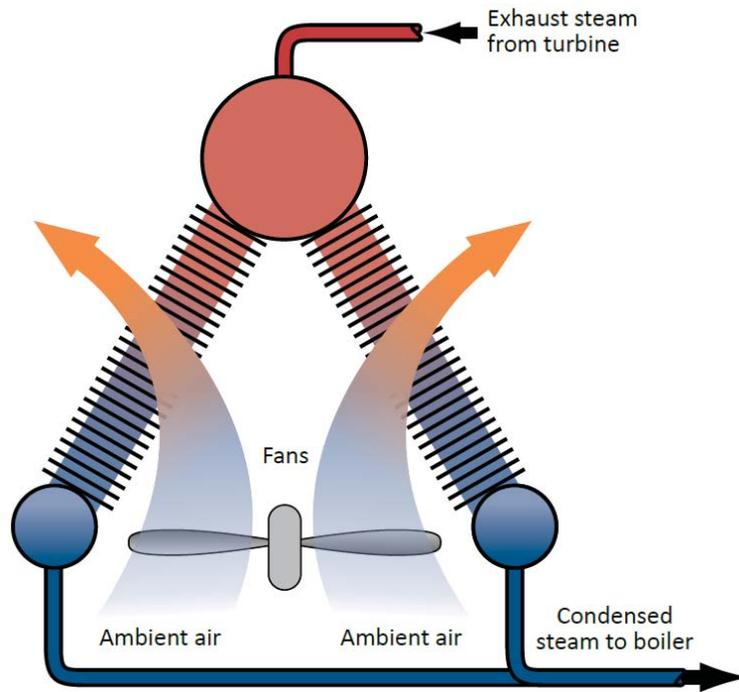
Figure 4: Direct dry cooling (Bushart, 2014)
