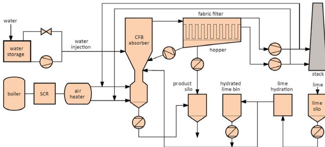
Figure 26: CFB scrubber system at Dry Fork power plant
