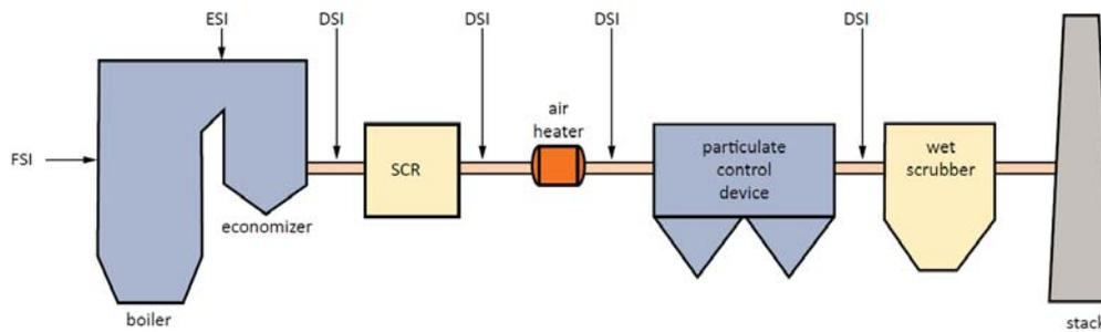
Figure 28: Possible sorbent injection locations
