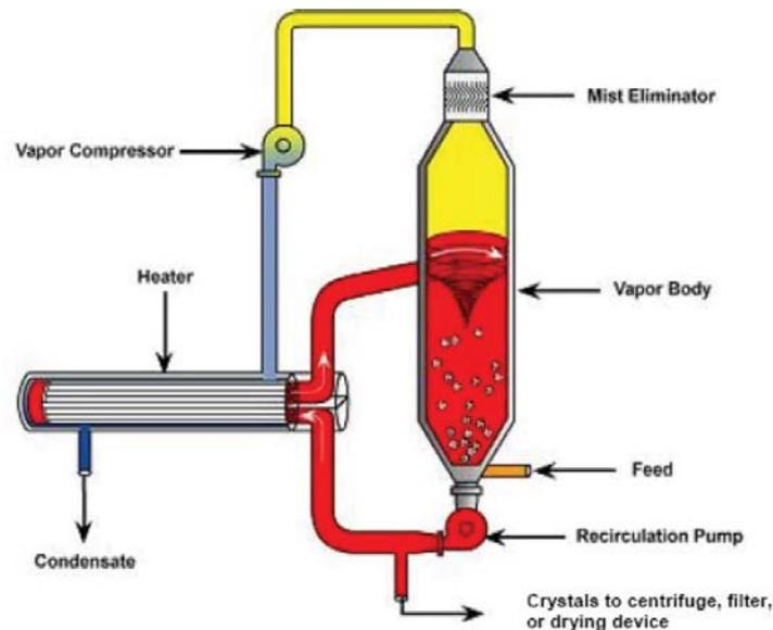
Figure 33: Crystallizer Schematic
