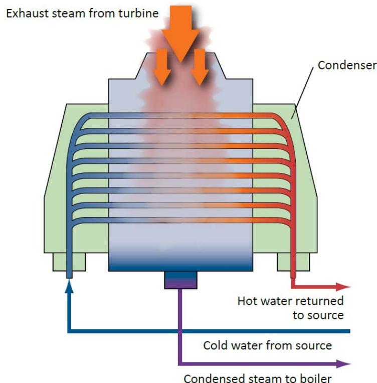
Figure 2: Water flow in once through cooling (Bushart, 2014)
