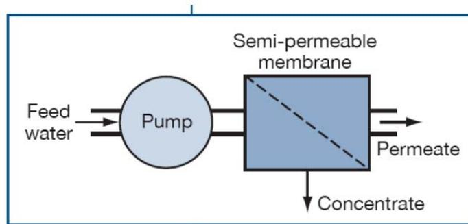
Figure 31: Reverse osmosis system schematic
