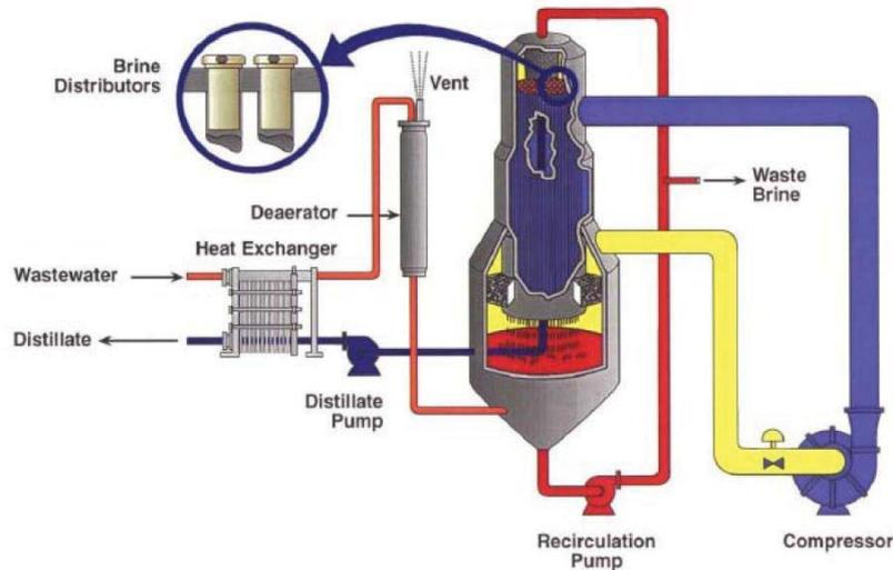
Figure 32: Vapor compression falling film evaporator schematic
