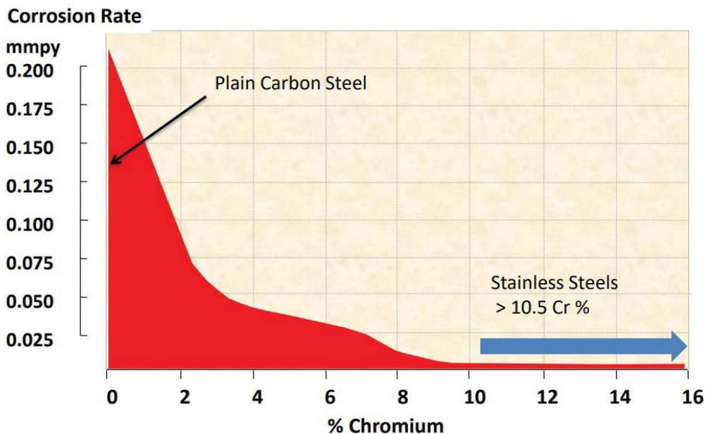
**Figure 3: Corrosion Rate of Carbon Steel and Stainless Steel**
