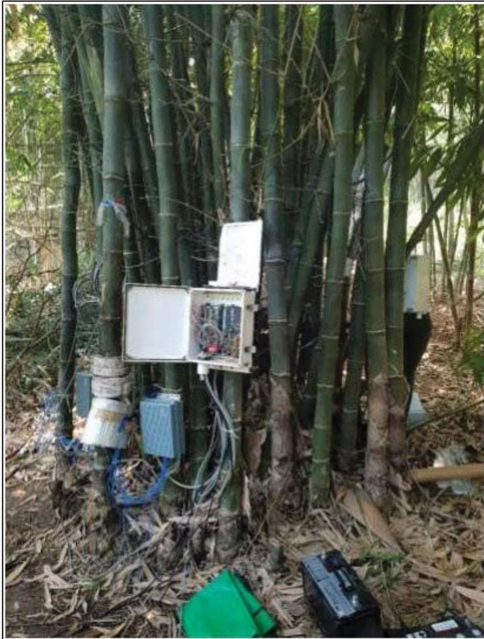
**Plate 4-7: HPV installation in the balcooa clump at Shooter's Hill**
