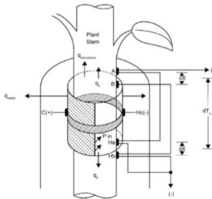
**Figure 2-11: Schematic diagram of the former stem flow sensor (Lascano et al., 2016)**
