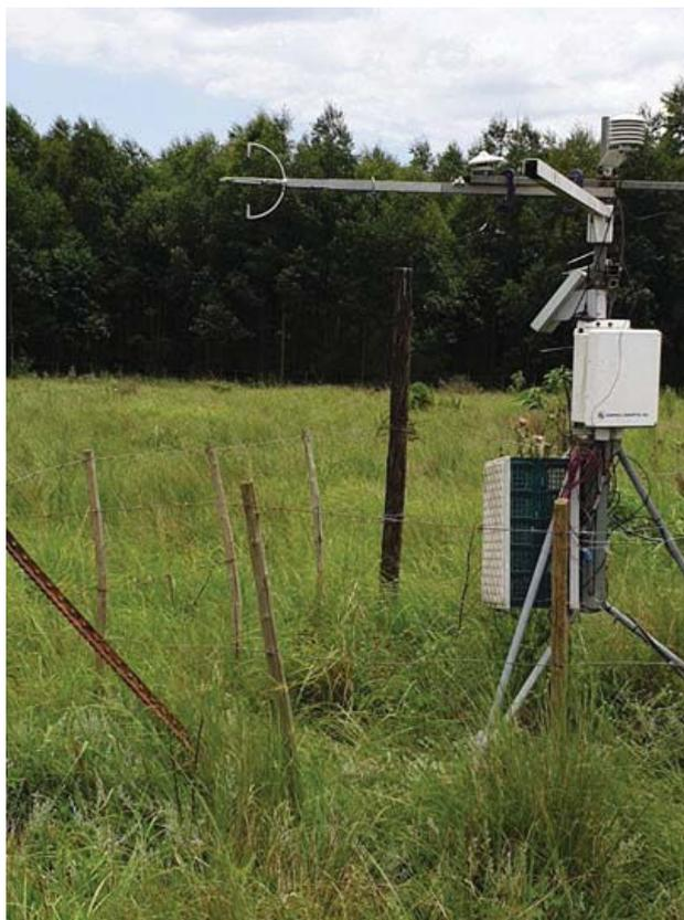
**Plate 5-7: Sonic anemometer and weather station**
