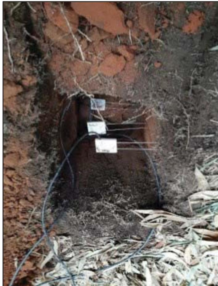
**Plate 4-2: Installed soil water probes (CS 616) for measuring soil water**
