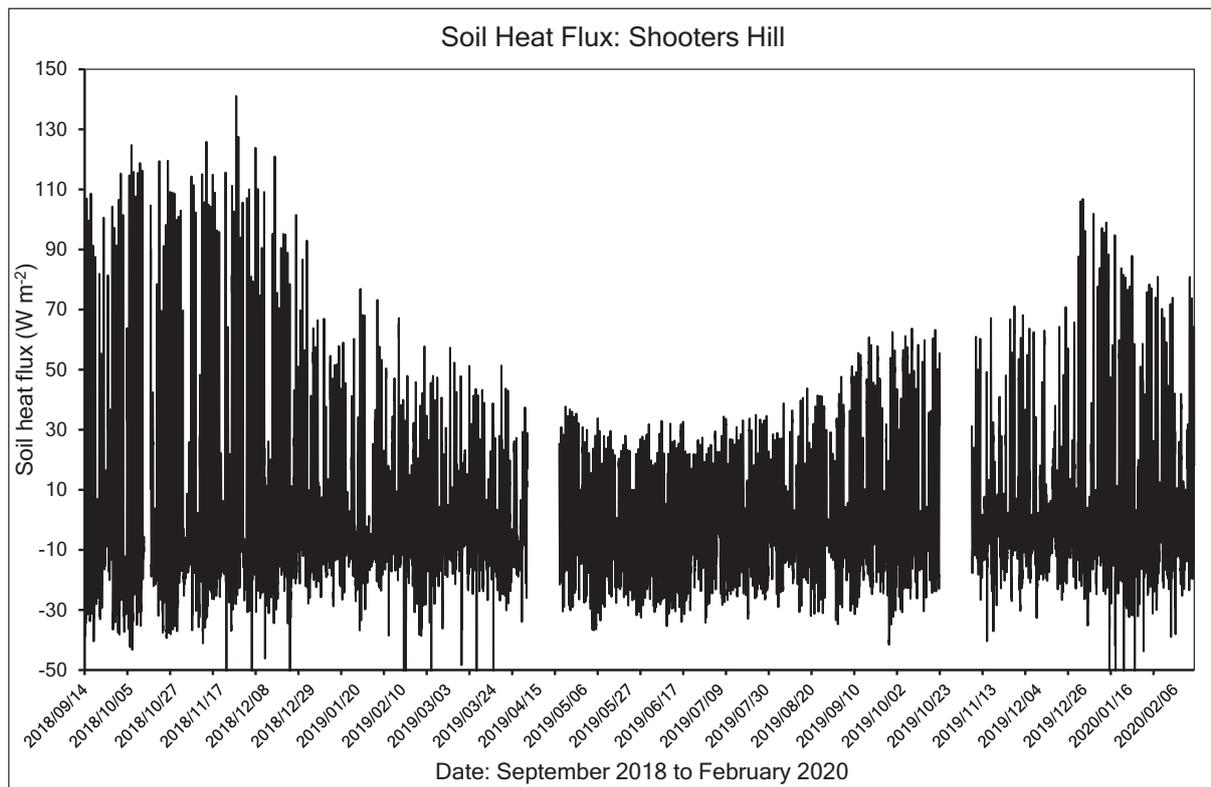
**Figure 5-47: Soil heat flux measured every 30 minutes at Shooter’s Hill grassland site from September 2018 to February 2020**
