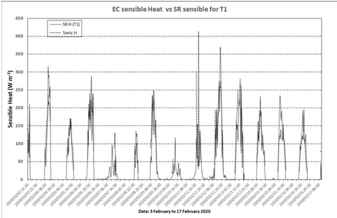
**Figure 5-42: The diurnal trends in the EC sonic and SR sensible heat flux at Shooter's Hill**
