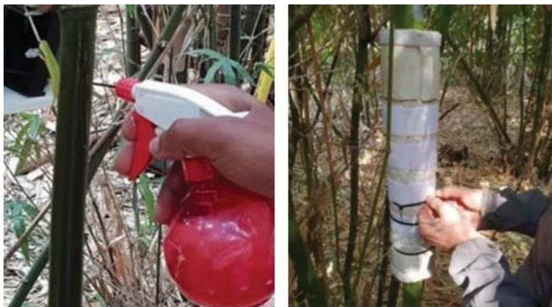
**Plate 4-12: Preparation and installation of the Dynamax collars**
