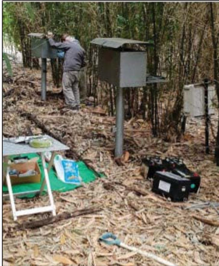
**Plate 4-8: Safe boxes for batteries (grey boxes) and the logger enclosure (white box) in the beema site**
