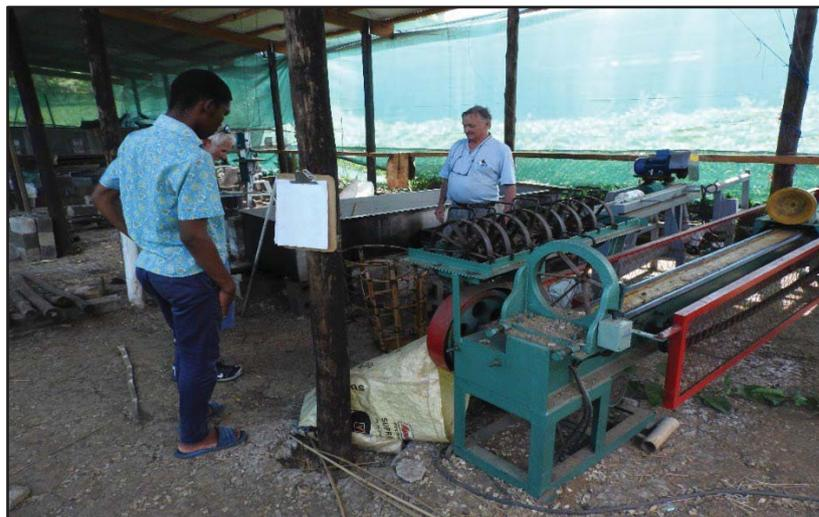
**Plate 3-3: Mechanical saw for splitting bamboo poles**
