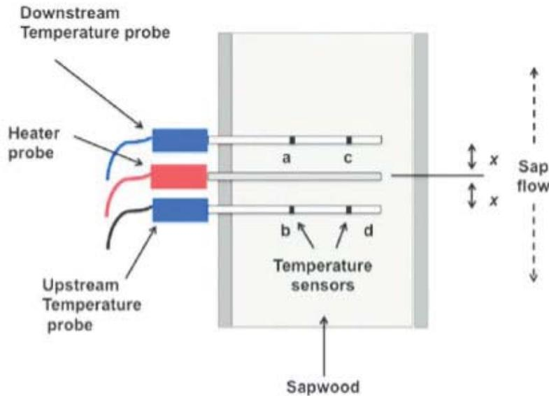
**Figure 2-13: Schematic diagram of the heat ratio method (Bayona-Rodriguez & Romero, 2016)**
