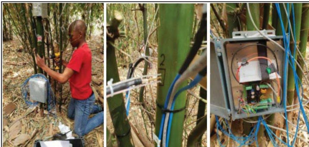
**Plate 4-6 Heater probes connected to a data logger and multiplexer**
