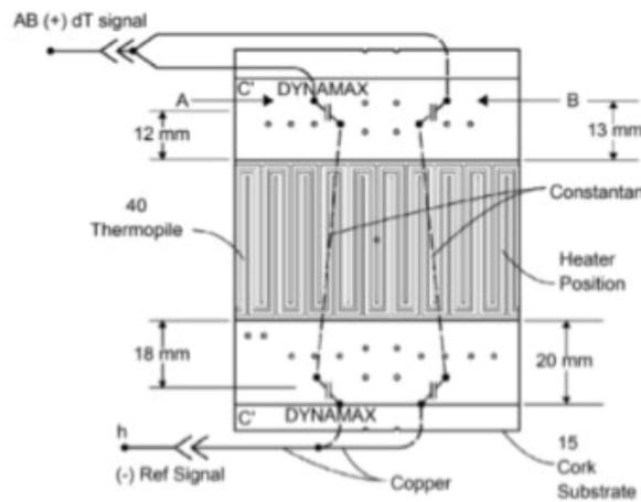
**Figure 2-12: Schematic diagram of EXO-Skin™ Sap flow Model SGEX-13 (Dynamax Inc., Houston, TX) (Lascano et al., 2016)**
