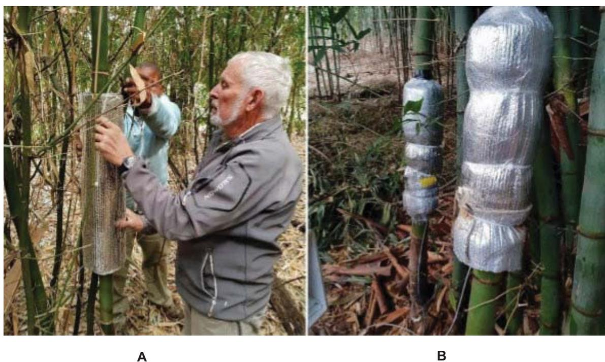
**Plate 4-13: A) Securing the sensor; and B) Completed Dynamax collar installation**
