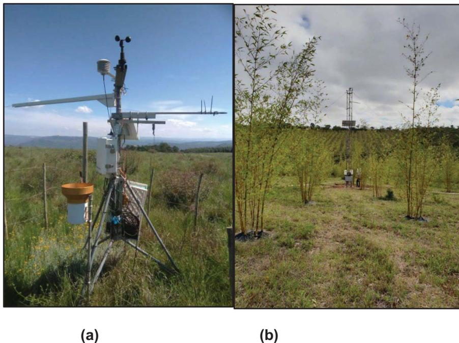
**Plate 4-1: Automatic weather station at the grassland site KwaZulu-Natal (a) and the 9 m lattice mast with the AWS in the Eastern Cape (b)**
