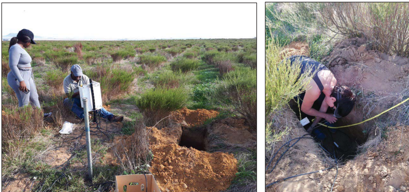
Figure 23. Installation of soil moisture sensors to monitor the volumetric soil water content in the root zone of the rooibos crop
