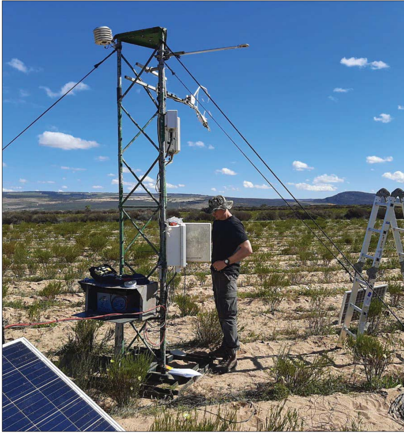
Figure 21. Installation of open path eddy covariance and surface renewal systems in rooibos.
