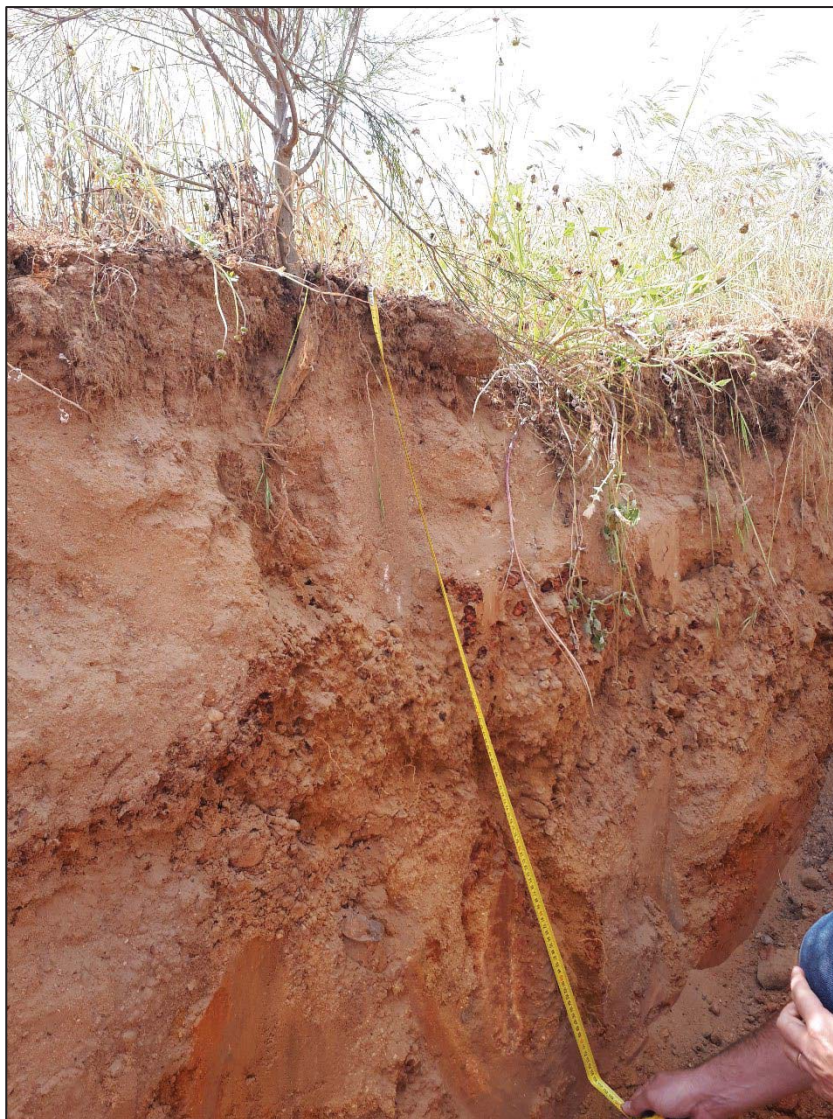
Figure 25. Soil profile for characterizing the soils at the Porterville study site
