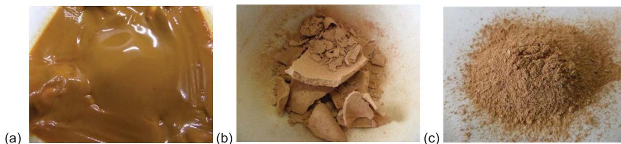
Figure 5.6. Light brown precipitate (pH 7): (a) Filtered (25°C) (b) Dried (180°C for 1 h) (c) Ground with pestle and mortar after drying
