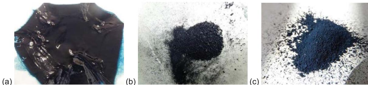
Figure 5.13. Light blue precipitates (pH 3): (a) Filtered (25°C) (b) Dried (180°C for 1 h) (c) Ground with pestle and mortar after drying
