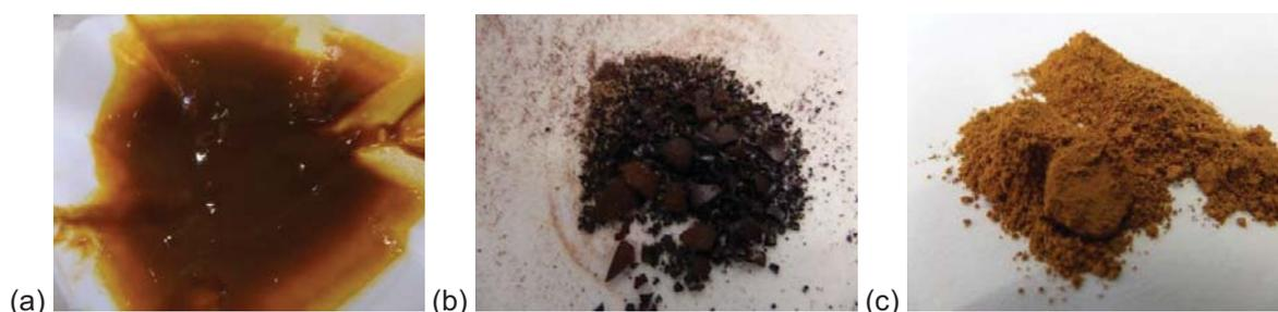
Figure 5.26. Reddish-brown precipitate (pH 5): (a) Filtered (25°C) (b) Dried (180°C for 1 h) (c) Ground with pestle and mortar after drying
