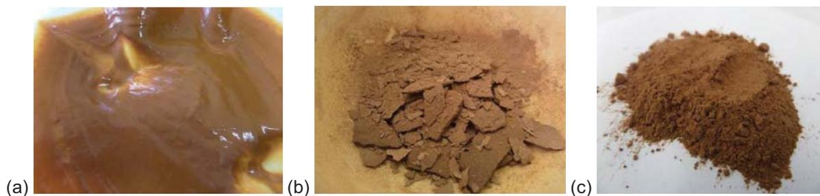
Figure 5.25. Brown precipitate (pH 9): (a) Filtered (25°C) (b) Dried (180°C for 1 h) (c) Ground with pestle and mortar after drying
