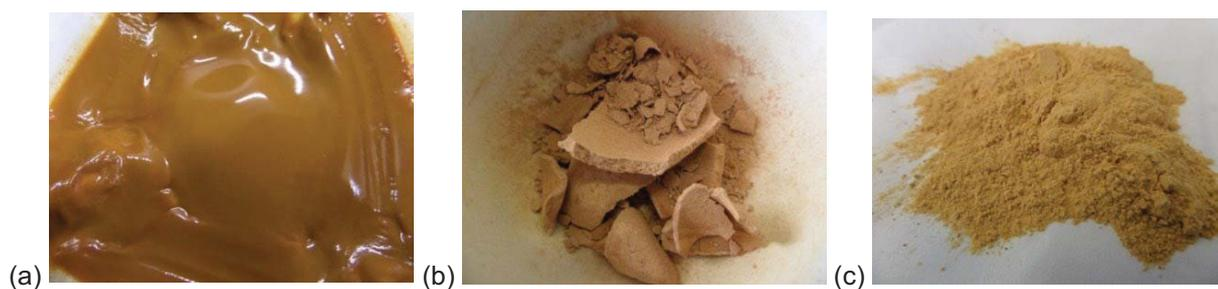
Figure 5.23. Light brown precipitate (pH 7): (a) Filtered (25°C) (b) Dried (180°C for 1 h) (c) Ground with pestle and mortar after drying
