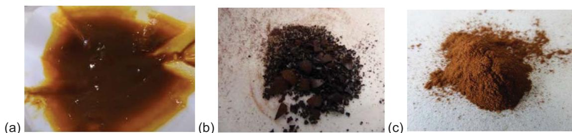
Figure 5.9. Reddish-brown precipitate (pH 5): (a) Filtered (25°C) (b) Dried (180°C for 1 h) (c) Ground with pestle and mortar after drying
