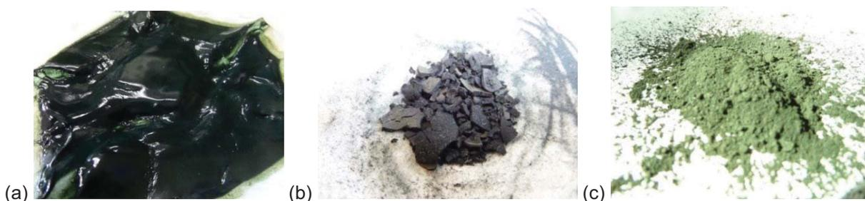
Figure 5.15. Green precipitate (pH 7): (a) Filtered (25°C) (b) Dried (180°C for 1 h) (c) Ground with pestle and mortar after drying
