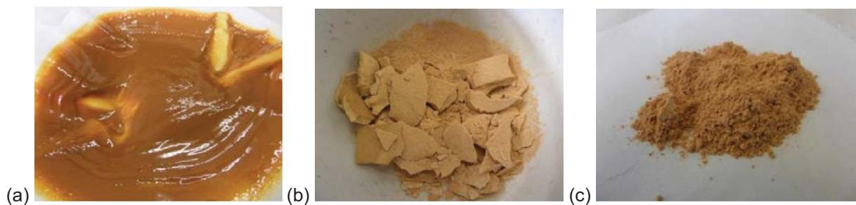
Figure 5.22. Yellow-brown precipitate (pH 6): (a) Filtered (25°C) (b) Dried (180°C for 1 h) (c) Ground with pestle and mortar after drying
