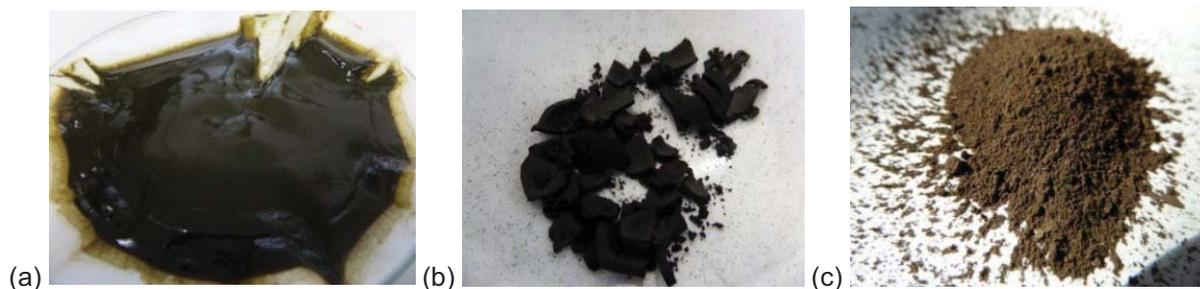
Figure 5.16. Brown precipitate (pH 9): (a) Filtered (25°C) (b) Dried (180°C for 1 h) (c) Ground with pestle and mortar after drying
