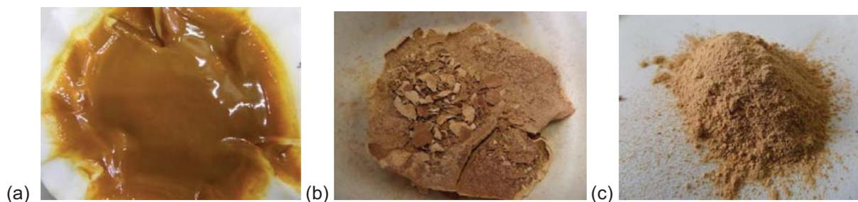
Figure 5.5. Brown precipitate (pH 6): (a) Filtered (25°C) (b) Dried (180°C for 1 h) (c) Ground with pestle and mortar after drying
