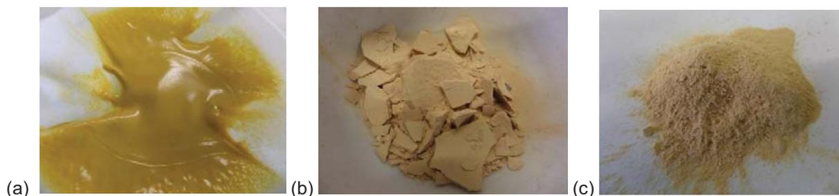
Figure 5.2. Yellow precipitates (pH 3): (a) Filtered (25°C) (b) Dried (180°C for 1 h) (c) Ground with pestle and mortar after drying
