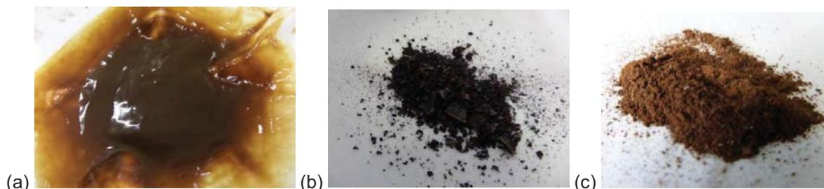
Figure 5.10. Brown precipitate (pH 7): (a) Filtered (25°C) (b) Dried (180°C for 1 h) (c) Ground with pestle and mortar after drying
