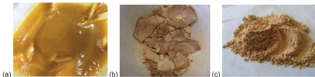
Figure 5.20. Yellow-brown precipitates (pH 4): (a) Filtered (25°C) (b) Dried (180°C for 1 h) (c) Ground with pestle and mortar after drying
