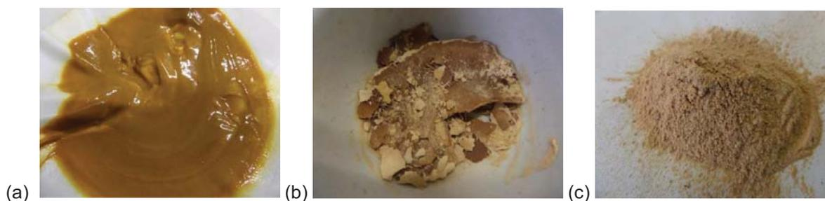
Figure 5.4. Yellow-brown precipitate (pH 5): (a) Filtered (25°C) (b) Dried (180°C for 1 h) (c) Ground with pestle and mortar after drying
