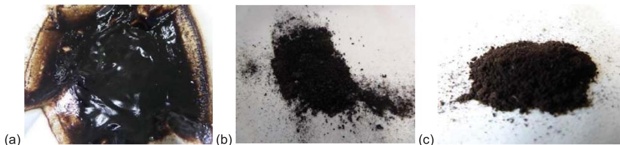
Figure 5.11. Black precipitate (pH 9): (a) Filtered precipitates (25°C) (b) Dried (180°C for 1 h) (c) Ground with pestle and mortar after drying.
