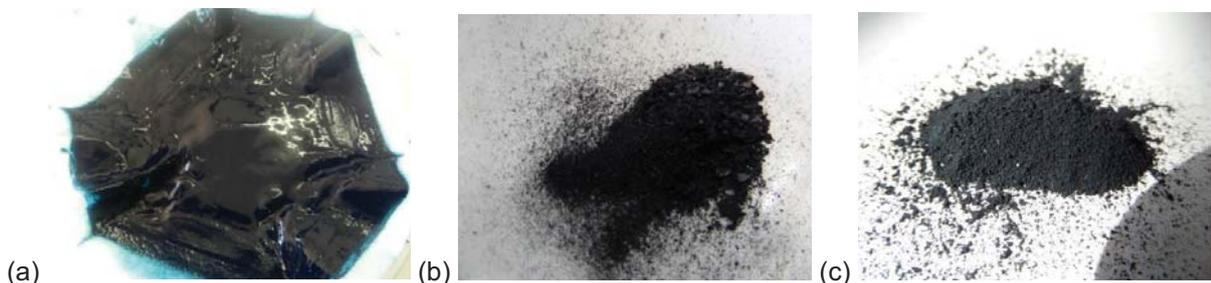
Figure 5.14. Dark blue precipitates (pH 5): (a) Filtered (25°C) (b) Dried (180°C for 1 h) (c) Ground with pestle and mortar after drying
