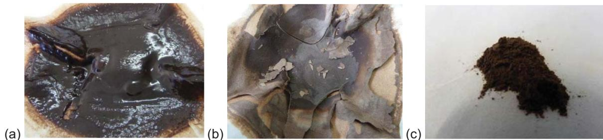
Figure 5.28. Brown-black precipitate (pH 9): (a) Filtered precipitates (25°C) (b) Dried (180°C for 1 h) (c) Ground with pestle and mortar after drying.
