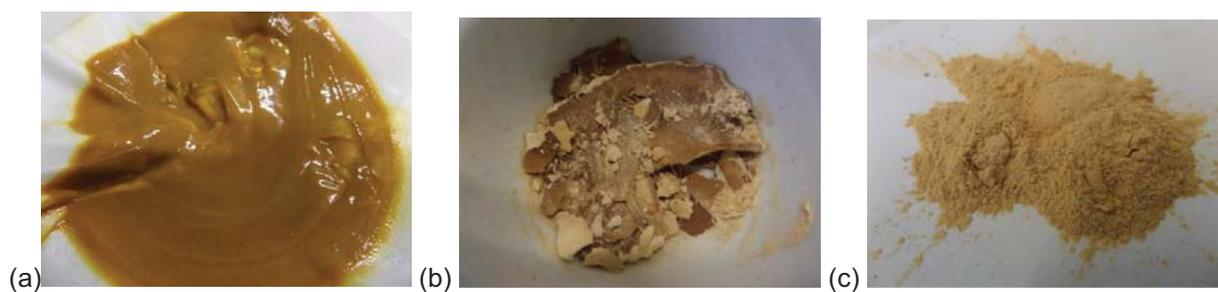
Figure 5.21. Yellow-brown precipitate (pH 5): (a) Filtered (25°C) (b) Dried (180°C for 1 h) (c) Ground with pestle and mortar after drying
