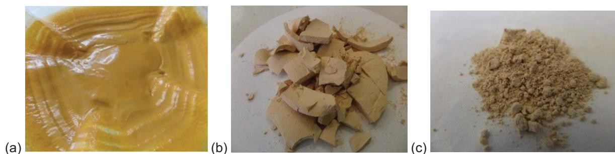
Figure 5.19. Yellow precipitates (pH 3): (a) Filtered (25°C) (b) Dried in oven (180°C) (c) Sample grinded with pestle and mortar after it was dried
