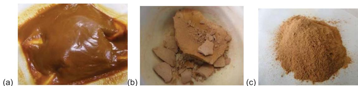
Figure 5.7. Reddish-brown precipitate (pH 8): (a) Filtered (25°C) (b) Dried (180°C for 1 h) (c) Ground with pestle and mortar after drying
