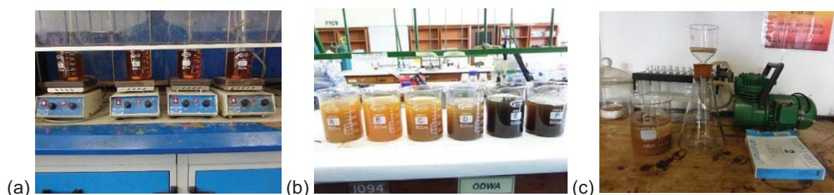
Figure 3.8. (a) Eight beakers stirred for 48 h to allow oxygen circulation in the reactions. (b) The pH values for precipitation increase from the extreme right beaker to the extreme left (i.e. pH 3 to 9). (c) Vacuum system used to filter the samples.
