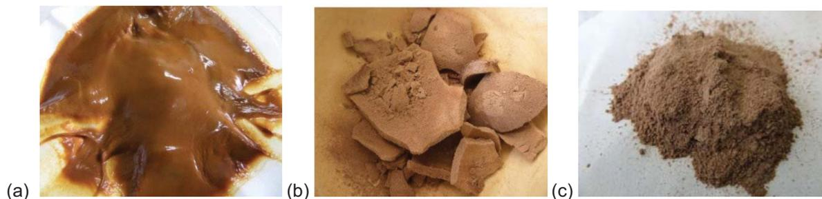
Figure 5.8. Brown precipitate (pH 9): (a) Filtered (25°C) (b) Dried (180°C for 1 h) (c) Ground with pestle and mortar after drying
