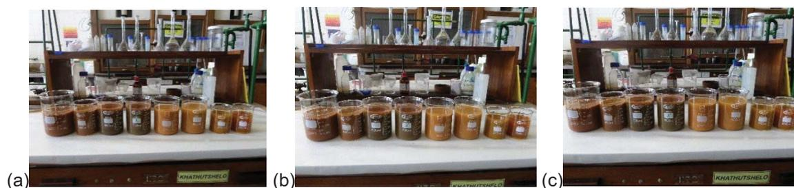
Figure 3.9. pH adjustment with (a) NaOH (b) MgCO<sub>3</sub> (c) CaCO<sub>3</sub> with precipitates formed in AMD after stirring for 48 h at 25°C
