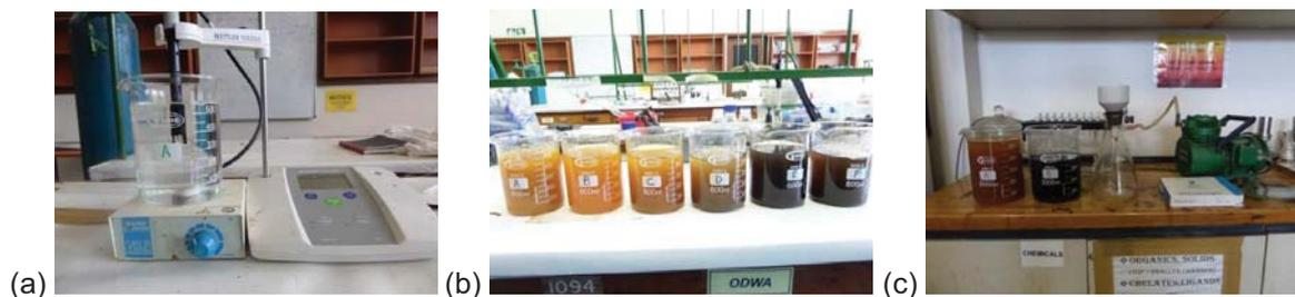
Figure 3.6. (a) pH adjustment with NaOH in initial solutions (b) precipitates formed in solutions after stirring for 48 h at  $25^\circ\text{C}$  (c) vacuum system used to filter precipitates.
