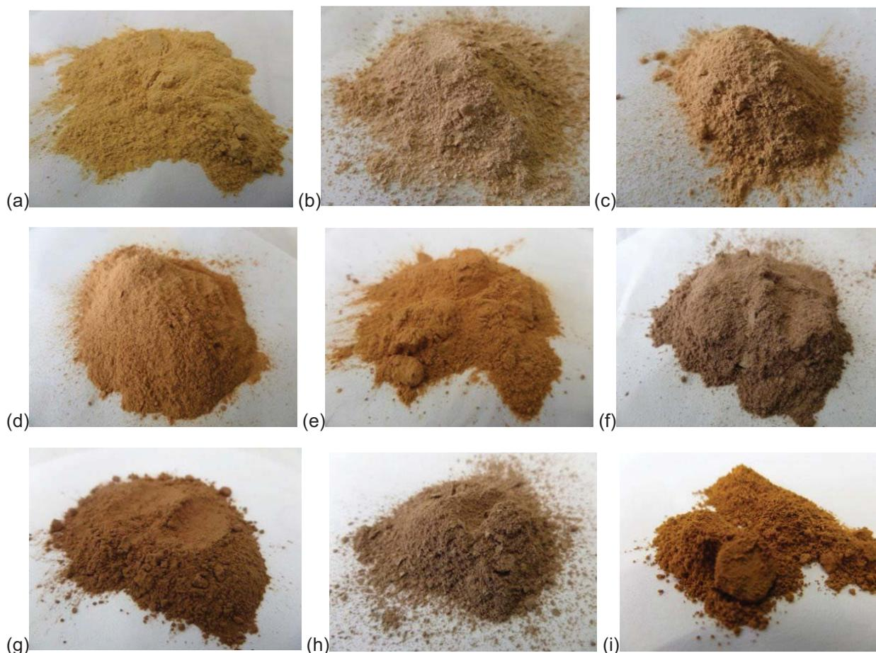
Figure 5.31. Precipitates using  $\text{CaCO}_3$  (pH 3-9): (a) to (i) Dried ( $180^\circ\text{C}$  for 1 h), ground with pestle and mortar after drying.
