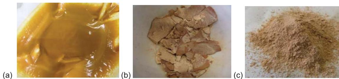
Figure 5.3. Yellow-brown precipitates (pH 4): (a) Filtered (25°C) (b) Dried (180°C for 1 h) (c) Ground with pestle and mortar after drying
