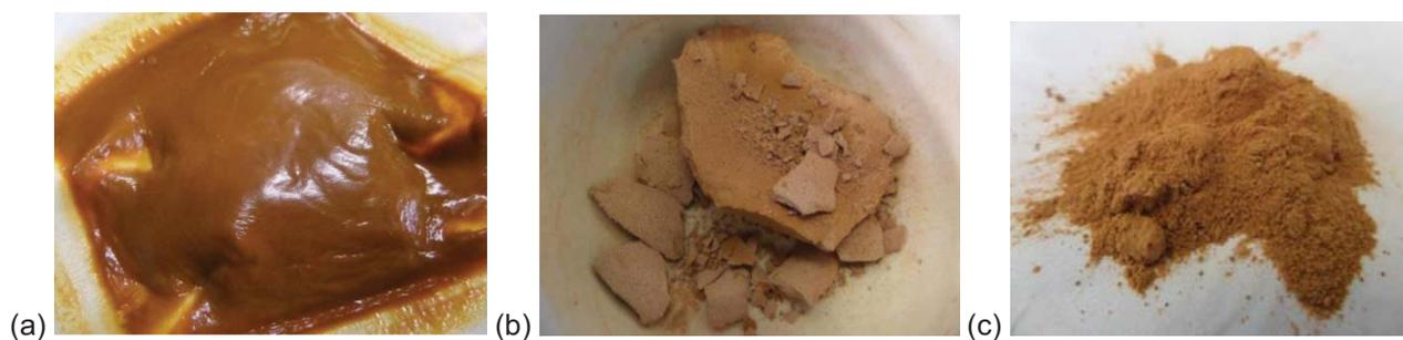
Figure 5.24. Reddish-brown precipitate (pH 8): (a) Filtered (25°C) (b) Dried (180°C for 1 h) (c) Ground with pestle and mortar after drying
