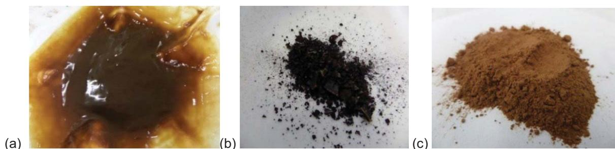
Figure 5.27. Brown precipitate (pH 7): (a) Filtered (25°C) (b) Dried (180°C for 1 h) (c) Ground with pestle and mortar after drying
