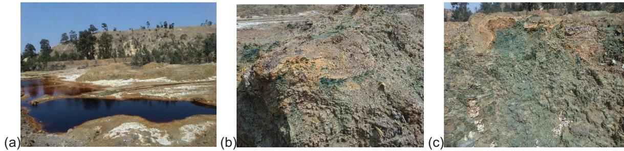
Figure 2.2. Gold recovery from tailings (a) AMD generated in the Central Rand basin (b) and (c) ferrocyanide containing water at pH 9 that mixed with AMD in the stream at pH 2.5, resulting in the formation of Prussian blue.
