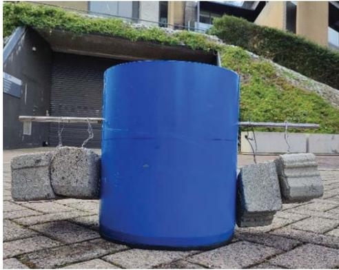
(a) Mod-ASTM C1781 test apparatus
