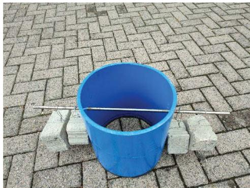
(a) Mod-ASTM C1781 test apparatus
