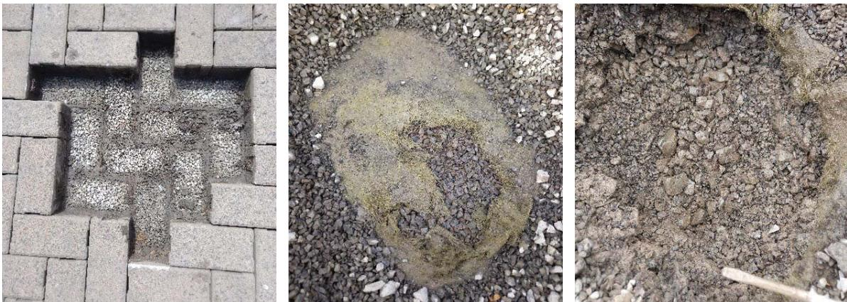
(a) Sediment outline      (b) Damaged geotextile      (c) Muddy film aggregates
