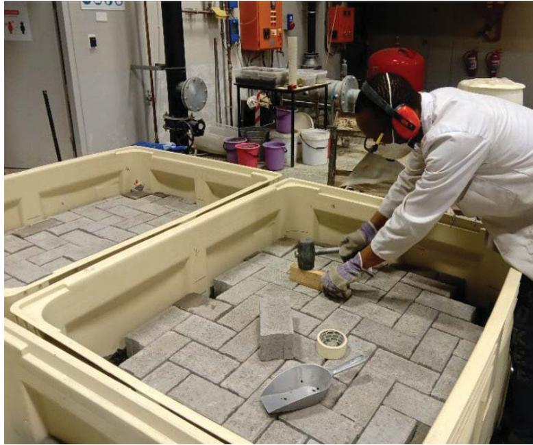
**Figure 5-5: Pavers being installed in the experimental cells**
