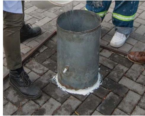
(b) ASTM C1781 test apparatus
