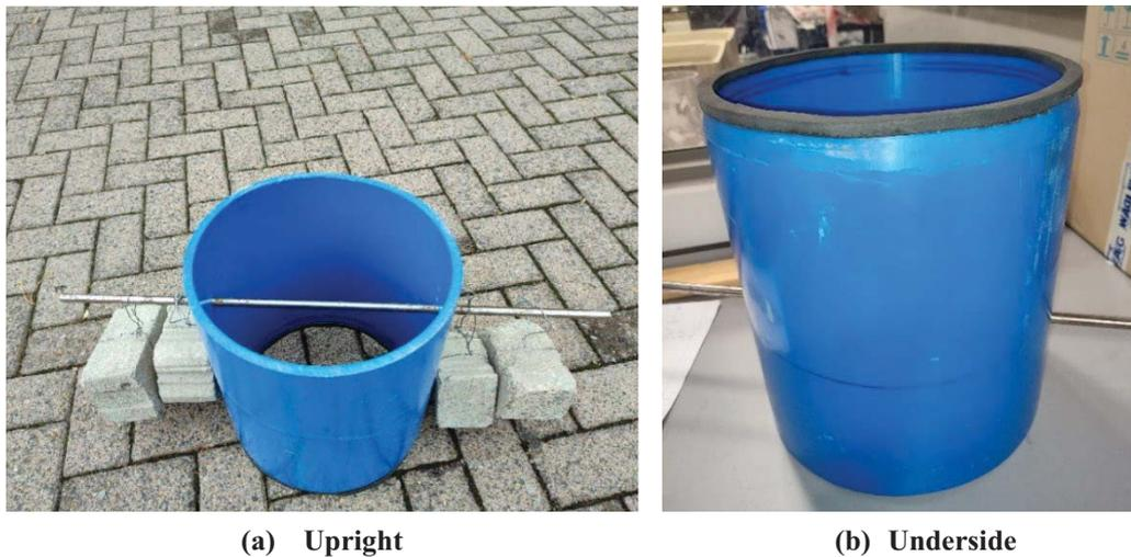
**Figure A-1: Mod-ASTM apparatus**
