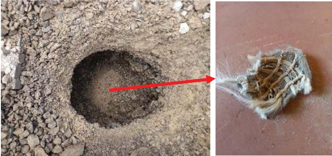
**Figure E-6: Damaged bottom geotextile**
