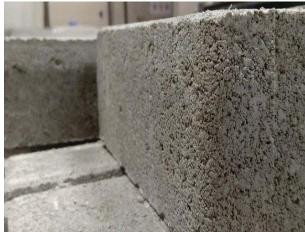
(b) Permaflow ® chamfered side
