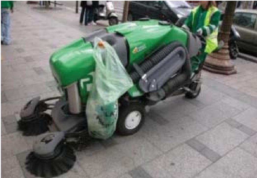
Figure 2-27: Mechanical street sweeper (NCDEQ, 2020)
