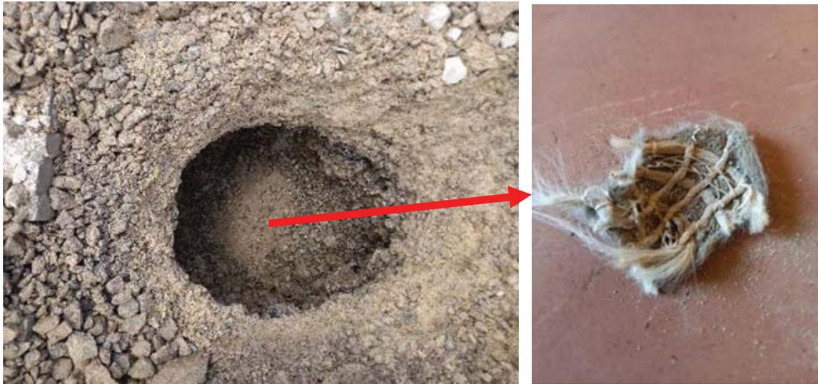
**Figure E-6: Damaged bottom geotextile**
