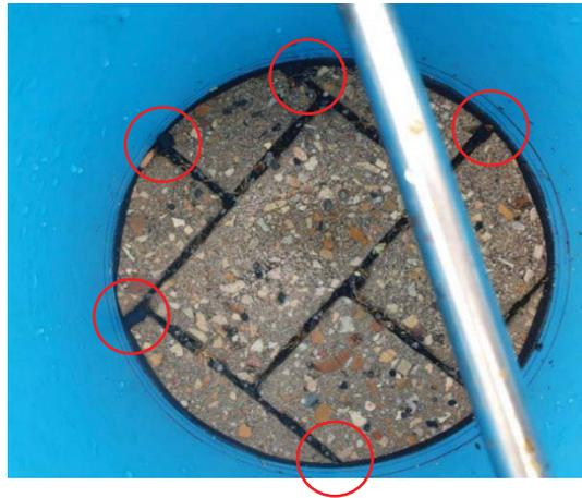
**Figure A-2: Neoprene pieces plugging the joints in Mod-ASTM**
