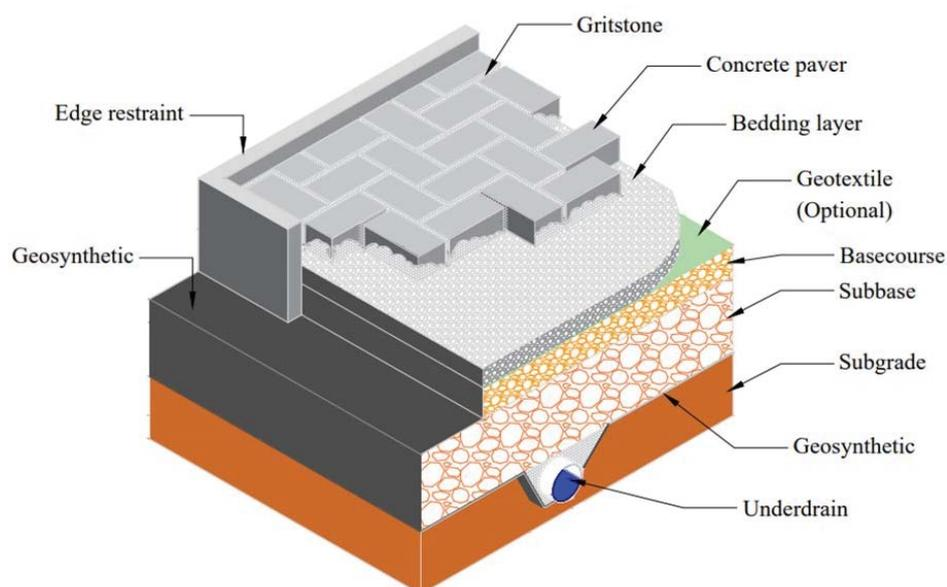
**Figure 1: Typical PICP section (After ICPI, 2020)**
