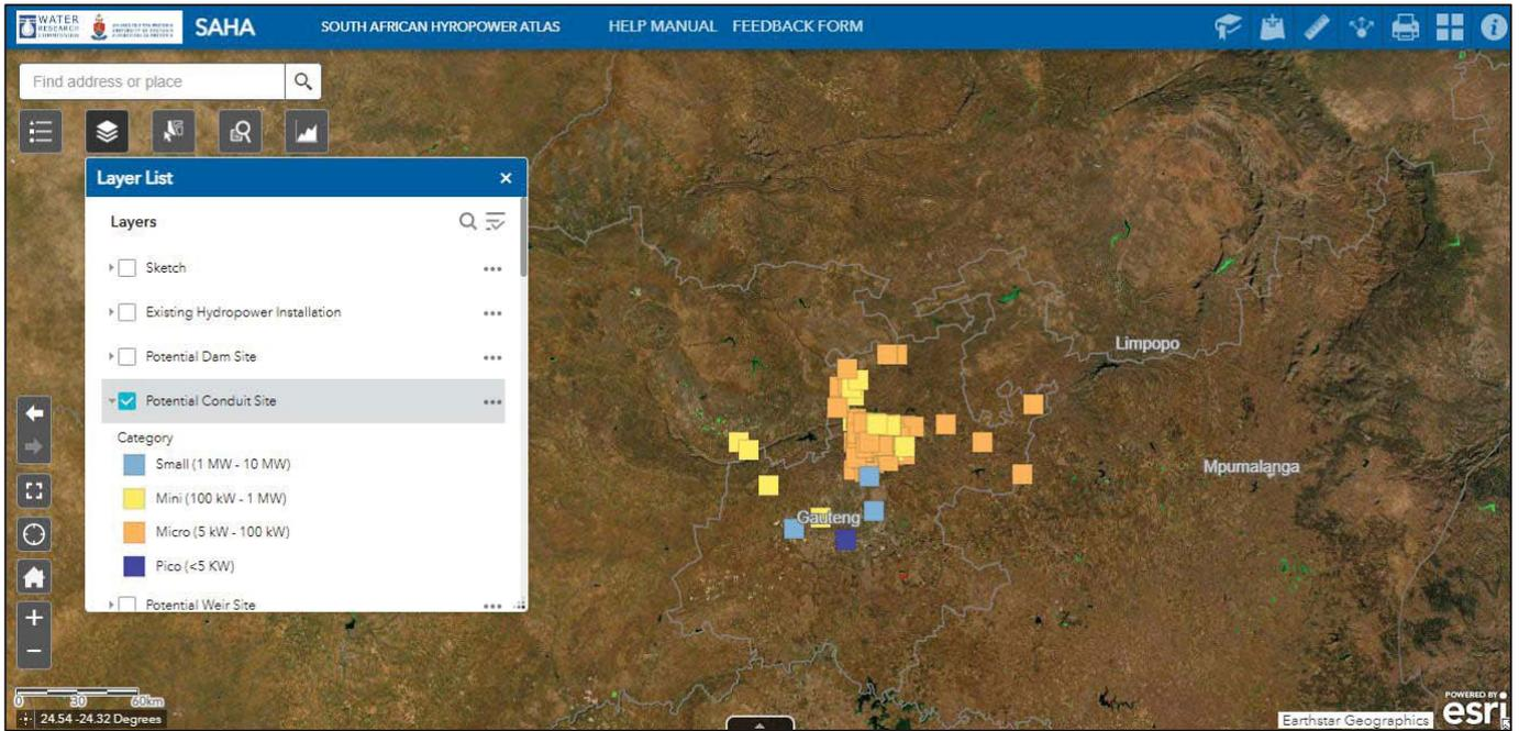
Figure 6-2: Conduit hydropower potential layer
