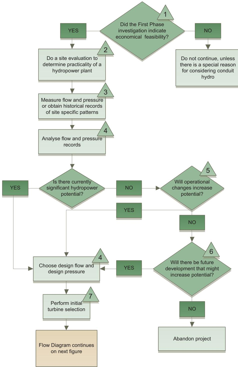
Figure 5-14: Phase 2 flow diagram Part A
