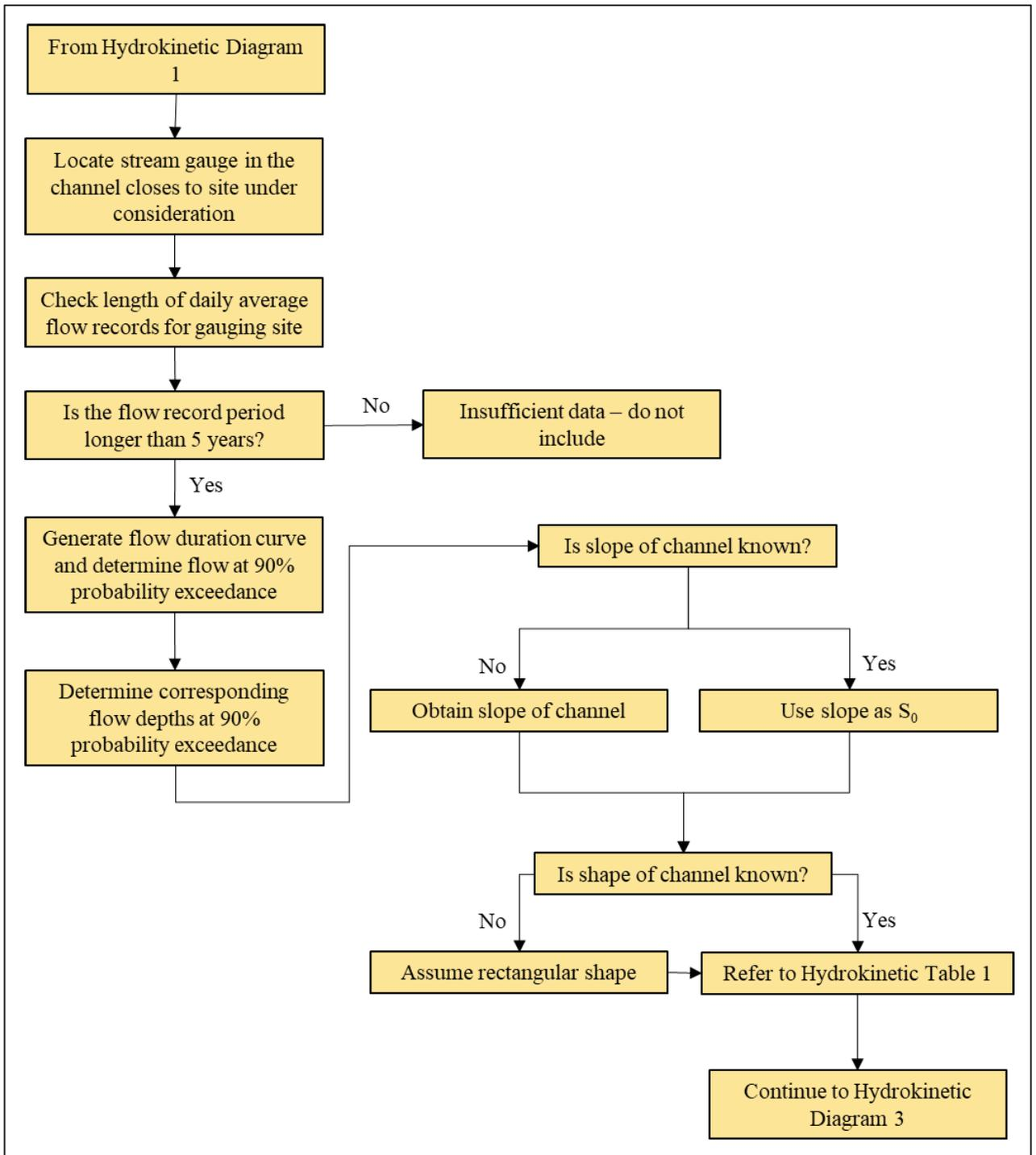
Figure 3-4: Hydrokinetic evaluation diagram 2
