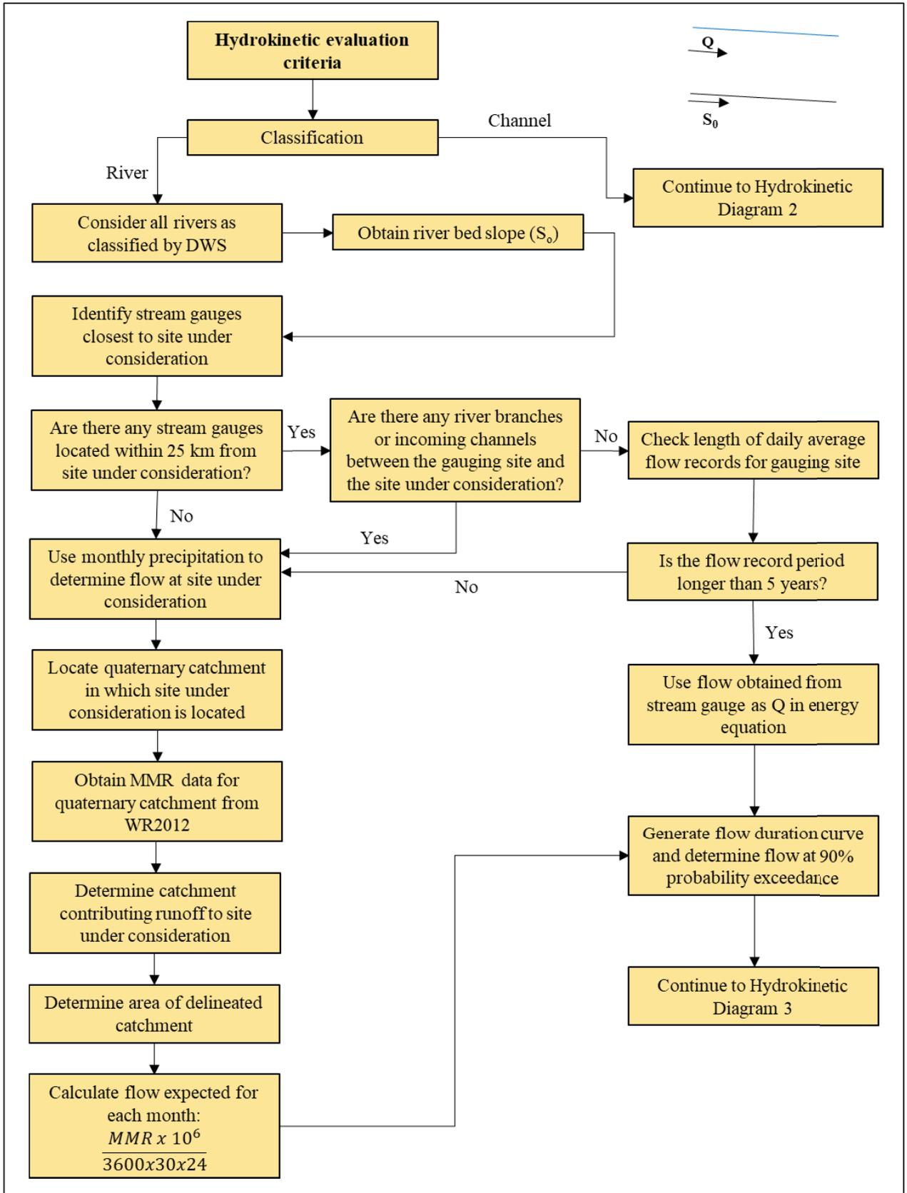
Figure 3-3: Hydrokinetic evaluation diagram 1
