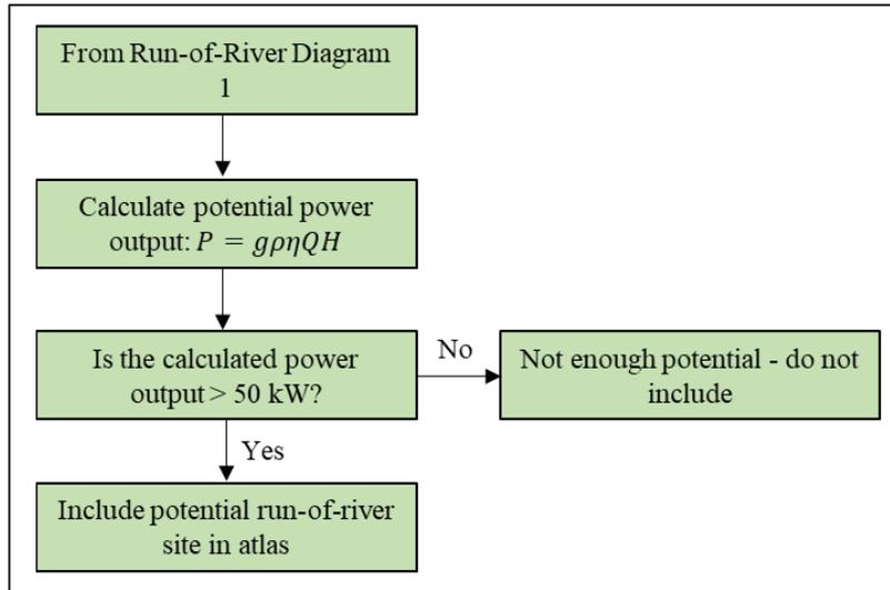
Figure 3-7: Run-of-river evaluation diagram 2
