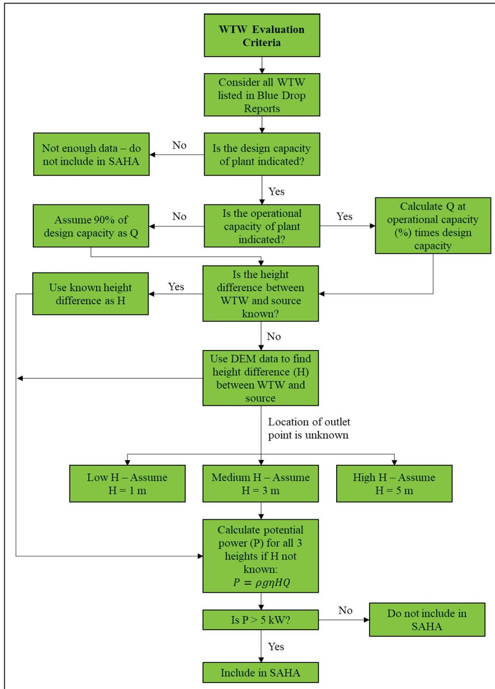
Figure 3-12: WTW evaluation diagram
