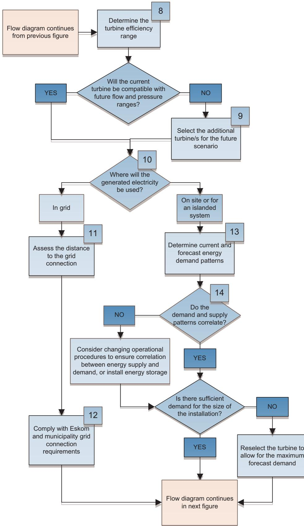
Figure 5-17: Phase 3 flow diagram Part B
