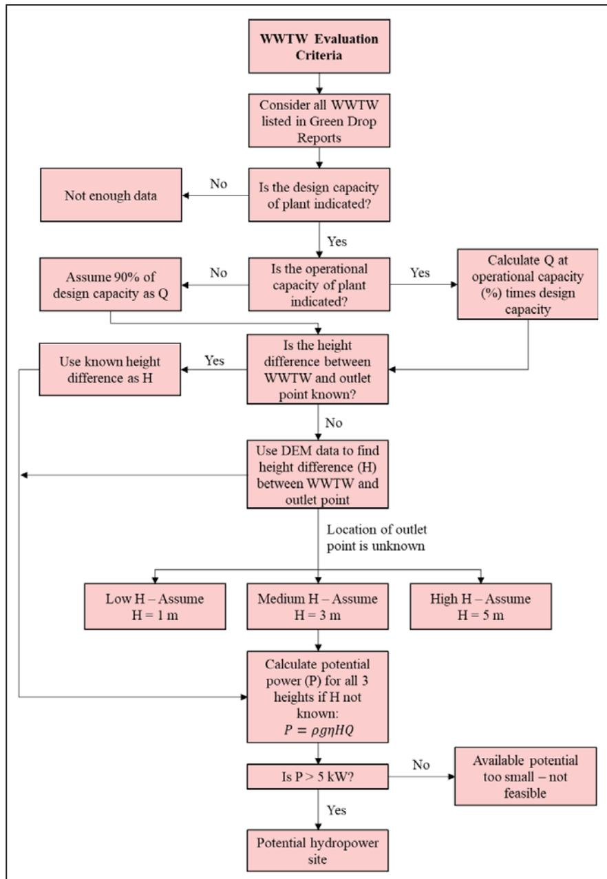
Figure 3-11: Diagrammatic depiction of WWTW evaluation framework
