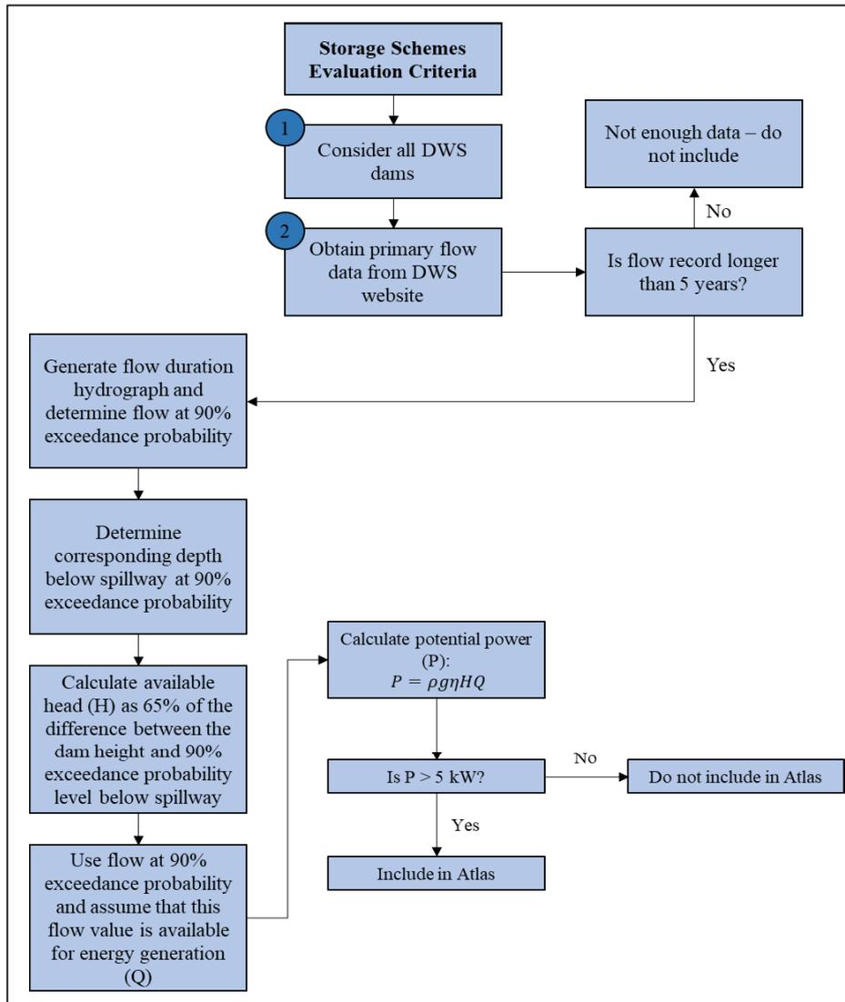
Figure 3-9: Storage scheme evaluation diagram
