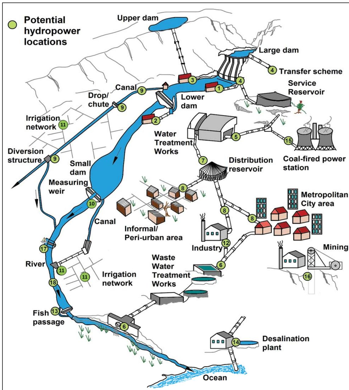
Figure 2-1: Locations of electricity generation potential (Adapted from Loots *et al.* (2015))
