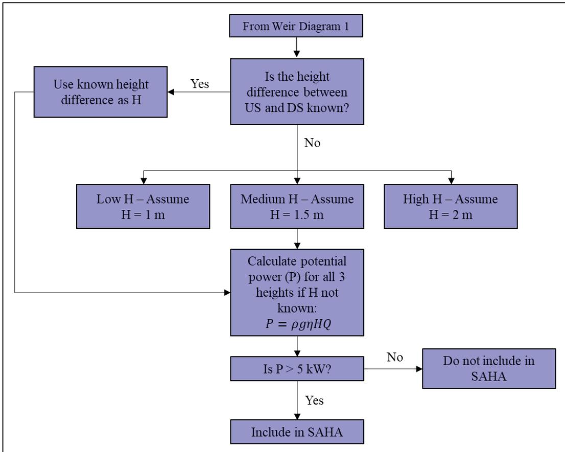
Figure 3-14: Weir evaluation diagram 2
