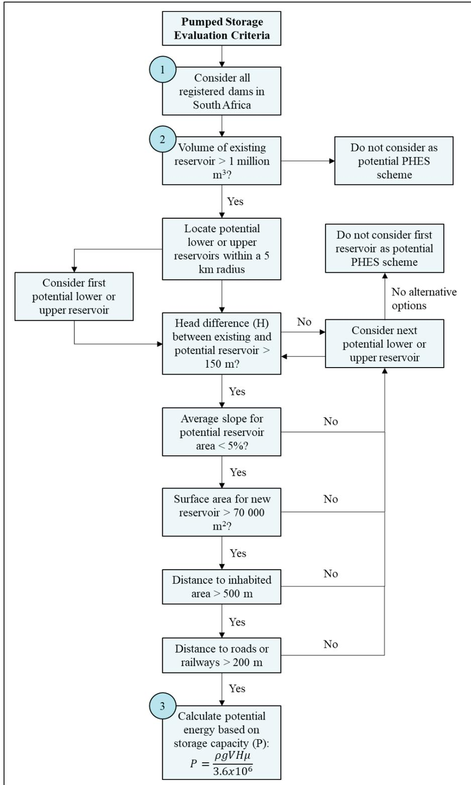
Figure 3-10: Pumped storage evaluation diagram
