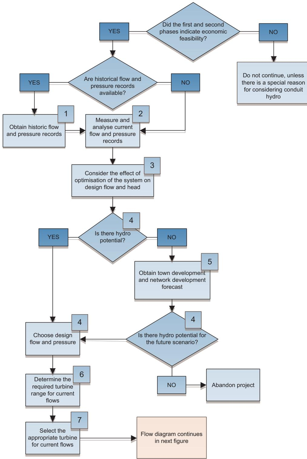
Figure 5-16: Phase 3 flow diagram Part A
