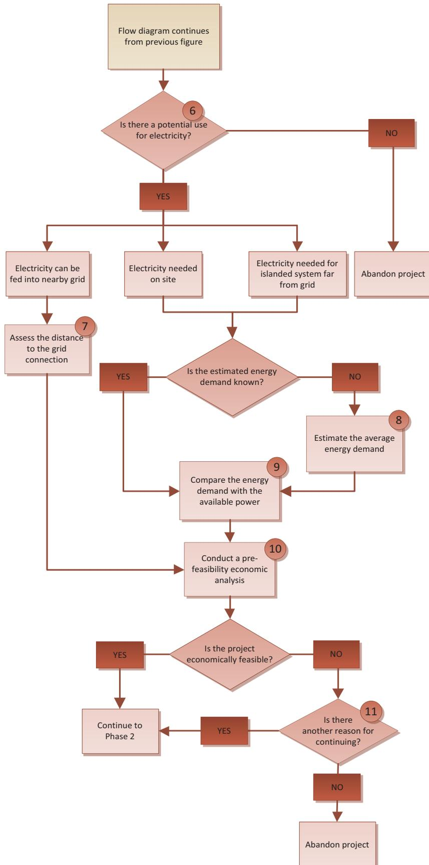
Figure 5-13: Phase 1 flow diagram Part B
