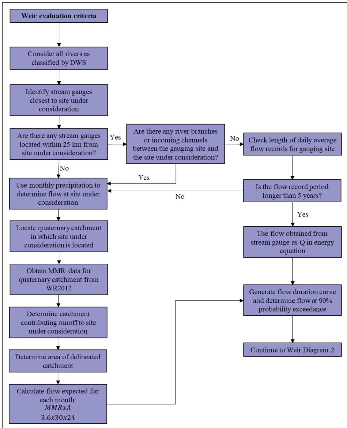
Figure 3-13: Weir evaluation diagram 1
