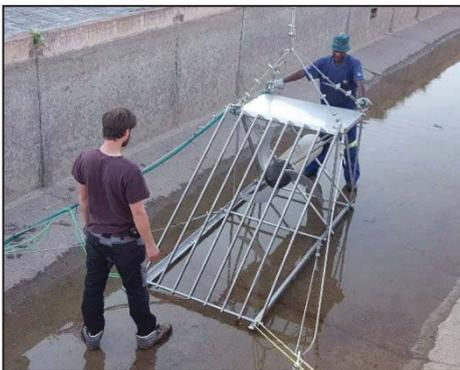
Hydrokinetic turbines in rivers and canals are referred to as zero head installations as energy is generated from kinetic energy in the flowing water.
