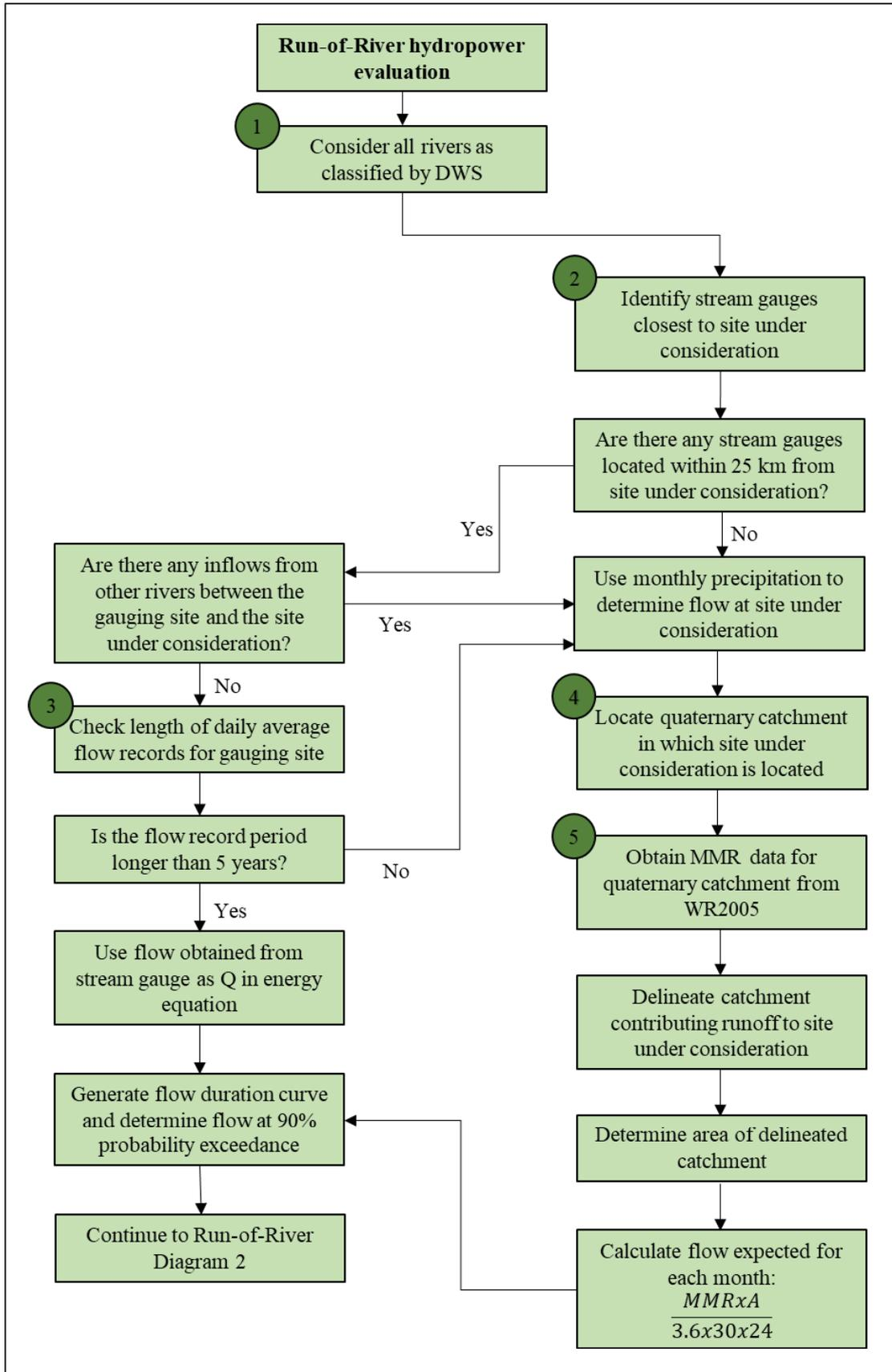
Figure 3-6: Run-of-river evaluation diagram 1
