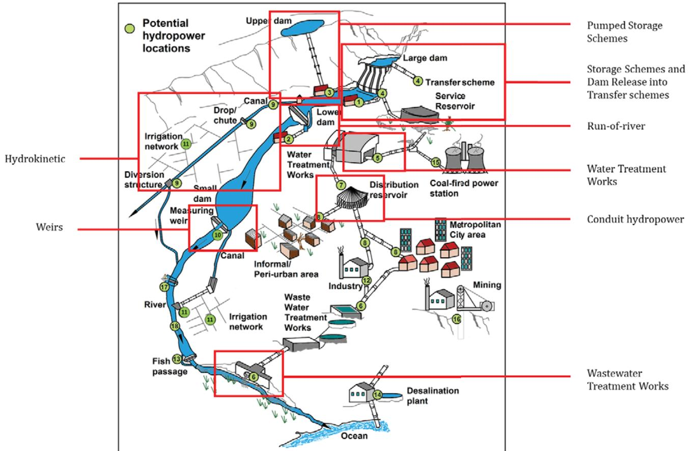
Figure 2-4: Hydropower types included in SAHA
