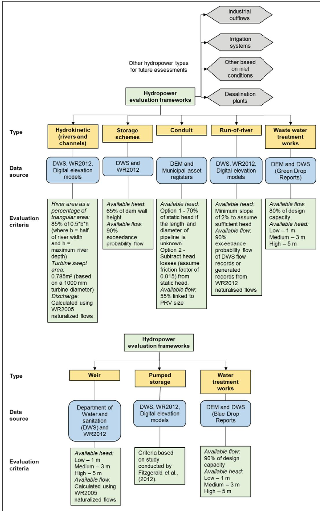
Figure ii: Summary of identified data sources and selected criteria for hydropower evaluation
