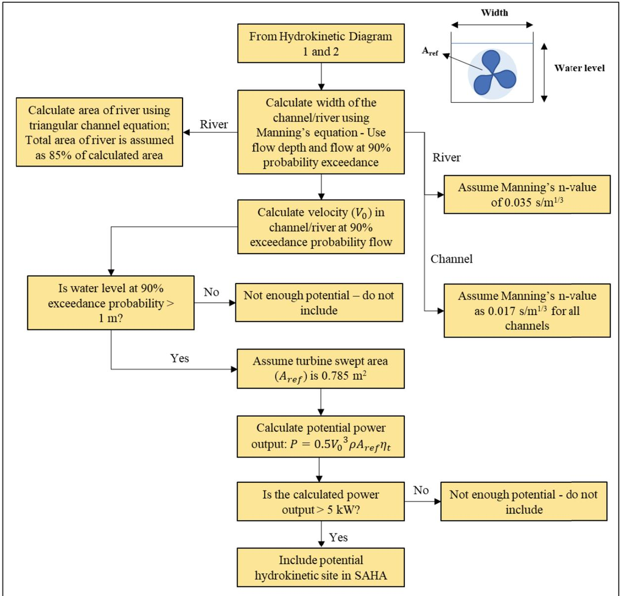
Figure 3-5: Hydrokinetic evaluation diagram 3
