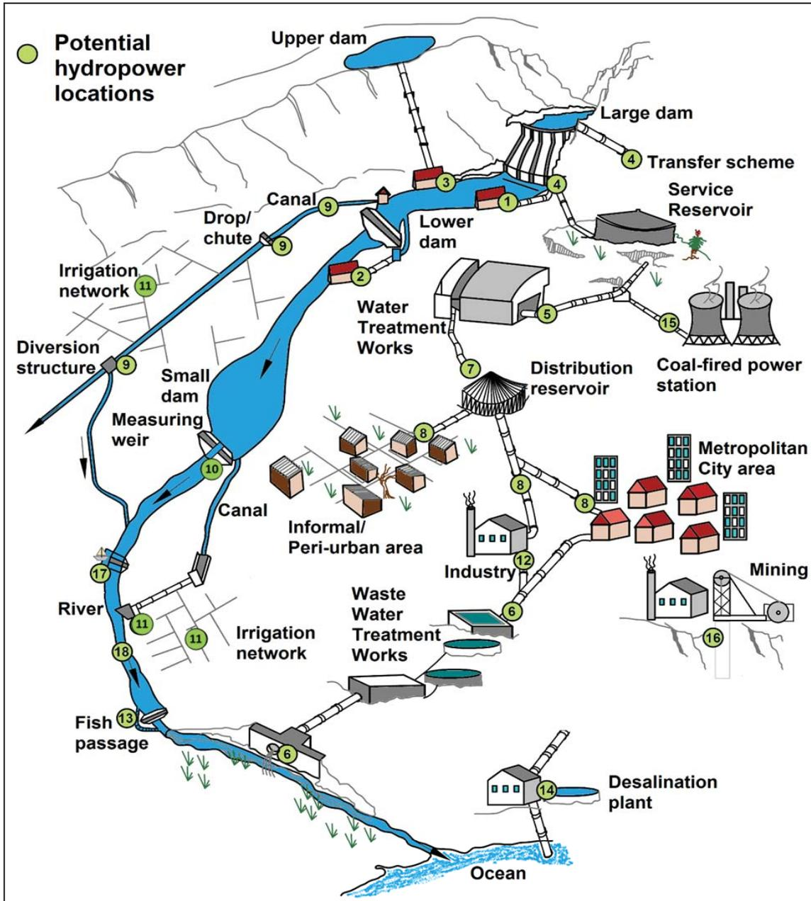
Figure i: Locations of electricity generation potential (Adapted from Loots *et al.* (2015))
