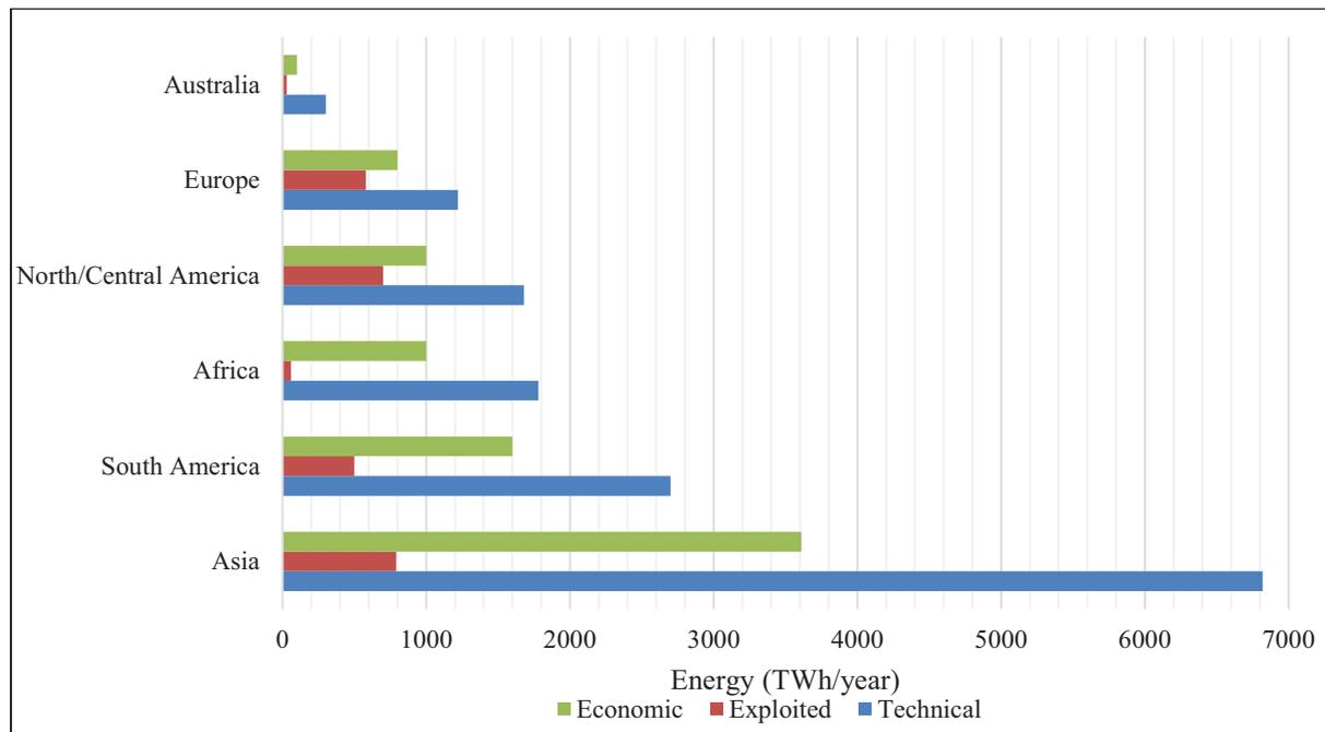
Figure 2-2: World hydropower potential (adapted from Pérez-Sánchez *et al.* (2017))
