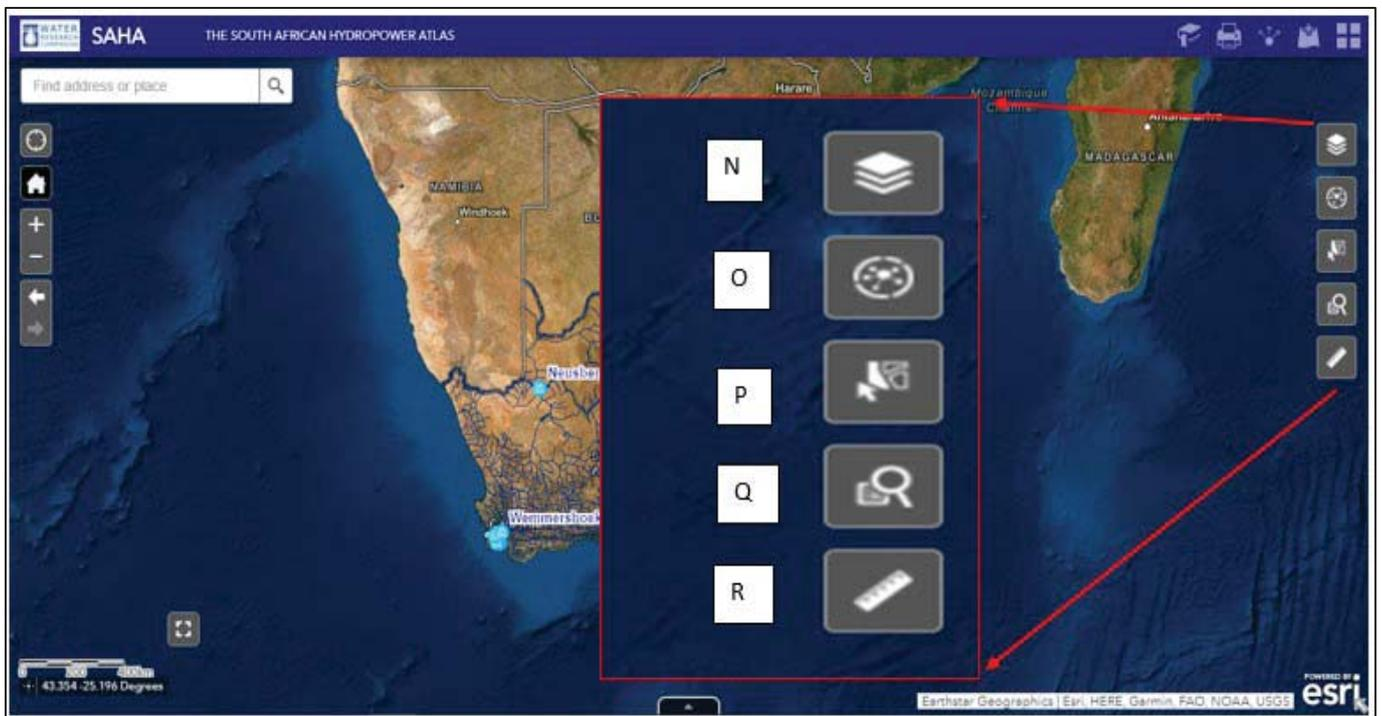
Figure 4-8: Data Layer list (N), The Analysis (O), Select (P), Query (Q), Measurement tool (R)
