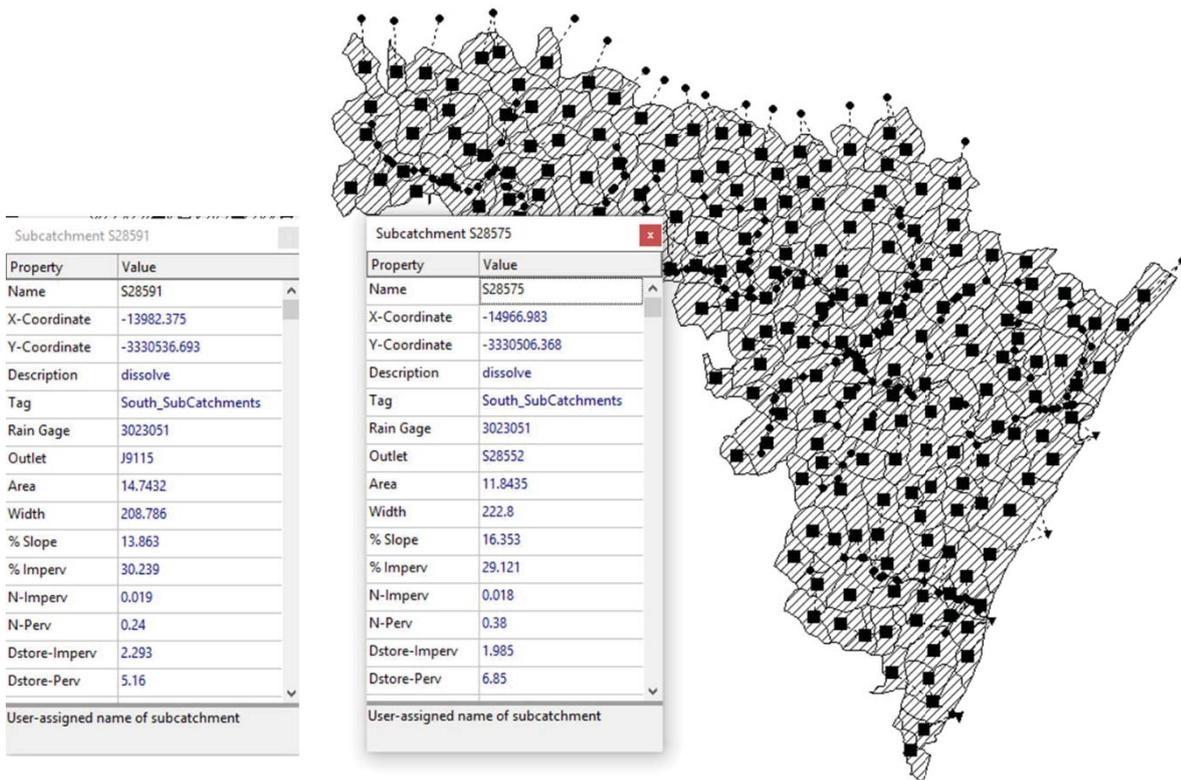
Figure 2.5. Sub-catchment properties and outlets in SWMM
