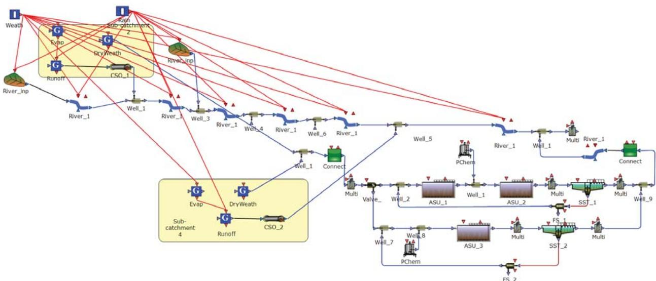
Figure 2.9. WEST layout for integrated model including the river sections in sub-catchments 1-4. Sub-catchments 2 and 4 are populated and have associated dry weather and run-off generators while sub-catchments 1 and 3 are unpopulated and represented by river inputs only.
