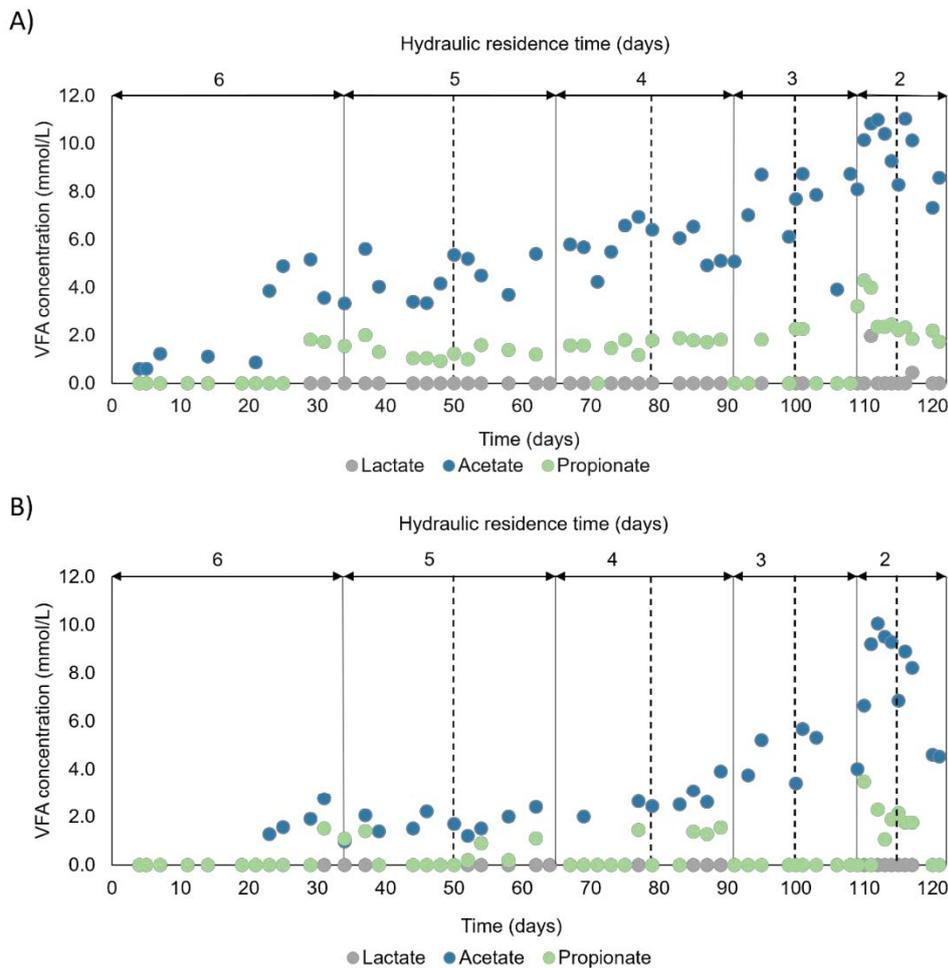
Figure 4-9: Effect of HRT on volatile fatty acid concentration profile measured over time showing A) primary reactor and B) secondary reactor. Solid and dotted vertical lines define FSB harvesting regime.
