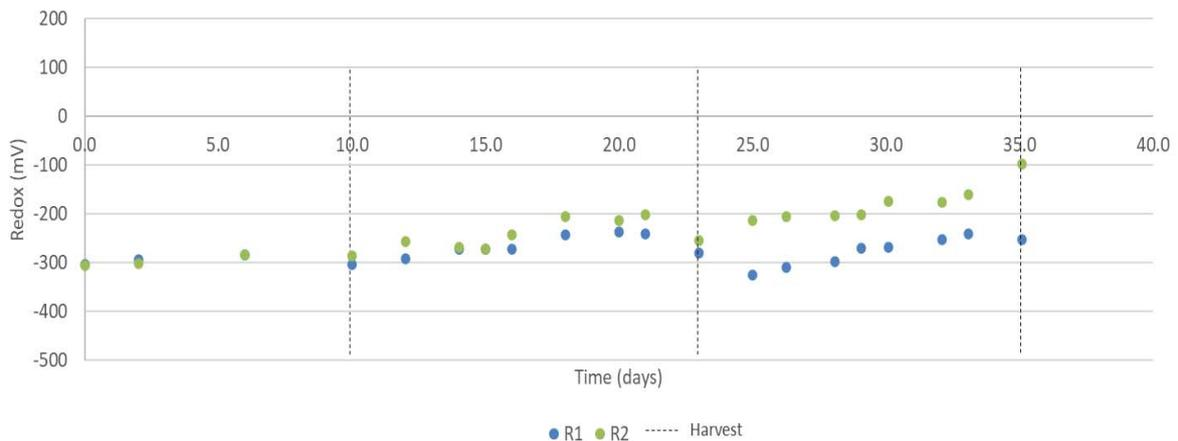
Figure 6-16: LFCR system fed with pretreated AMD with a molasses substrate - redox time trends
