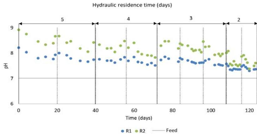
Figure 4-14: Effect of HRT on pH profile within the samples taken from the primary and secondary reactors. Solid and broken vertical lines define the FSB harvesting regime.
