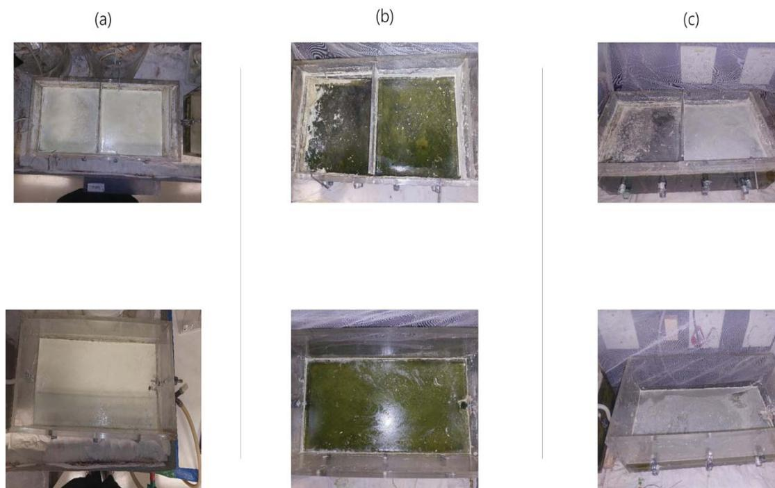
Figure 6-10: Top view of the primary (top) and secondary (bottom) reactor showing (a) FSB formed during a 3-day HRT experiment with a 100% synthetic AMD feed, (b) thin film formed during a 3-day HRT experiment with a 80% AMD and 20% synthetic AMD feed and (c) FSB and thin film mixture formed during a 3-day HRT experiment with a 100% AMD feed
