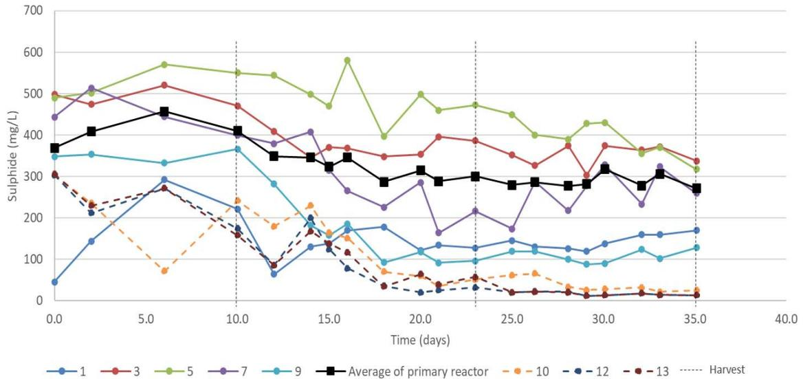
Figure 6-15: Sulphide time trends for 8 L LFCR system fed with pretreated AMD and molasses.
