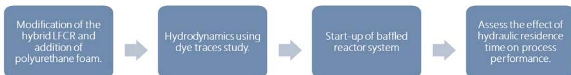
Figure 4-1: Flow chart illustrating the experimental approach for testing the modified hybrid baffled reactor.
