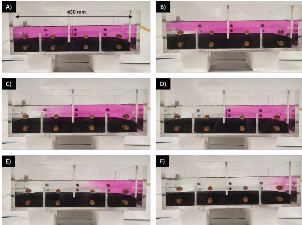
Figure 4-5: Dye tracer study showing photographic images on the progression of mixing over time in the baffled reactor with polyurethane foam operated at a flow rate equivalent to a 12 h HRT, photographs taken at A) 0 min B) 44 min C) 1 h 24 min D) 2 h 7 min E) 2 h 26 min F) 2 h 51 min.
