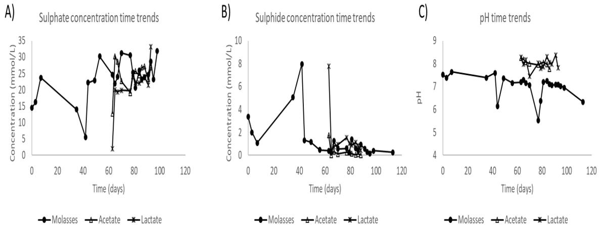
Figure 5-8: Molasses, acetate, and lactate mini-column time trends for A) sulphate concentration B) sulphide concentration C) pH.
