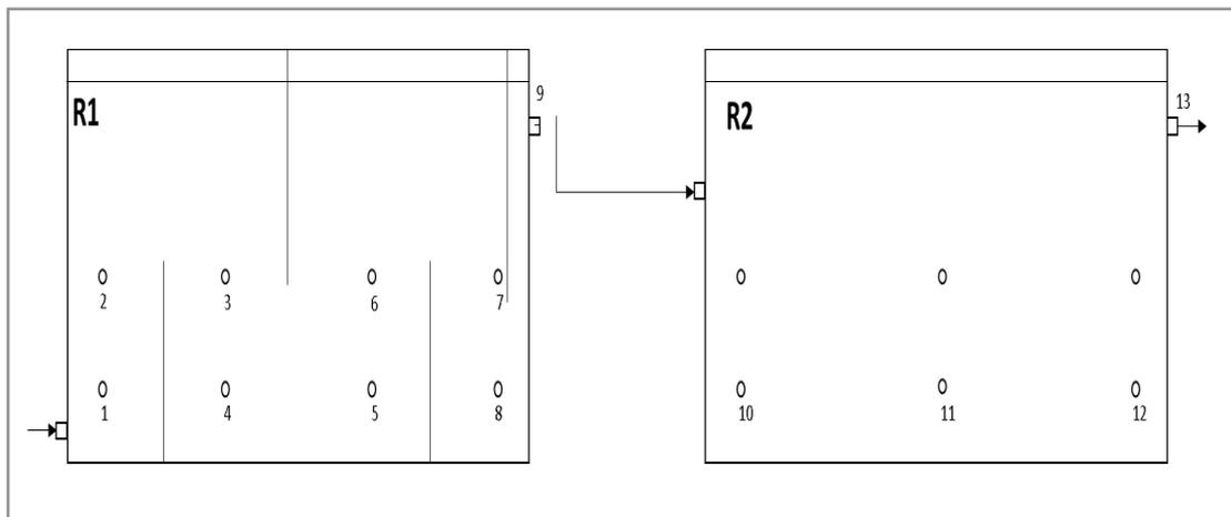
Figure 6-5: Sampling layout of the primary and secondary LFCRs (R1: primary reactor and R2: secondary reactor)
