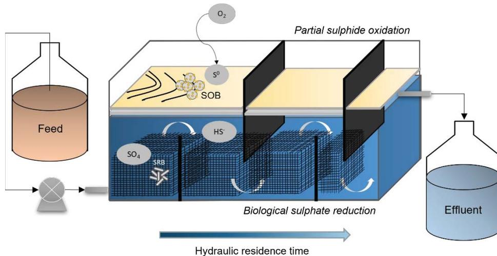
Figure 4-2: Conceptual model of the modified baffled reactor system incorporating sulphate reduction and sulphide oxidation.
