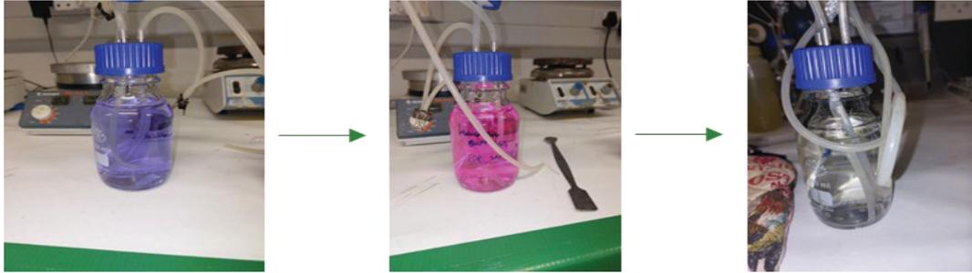
Figure 5-9: Feed (set-up and batch mode) dissolved oxygen test using resazurin.
