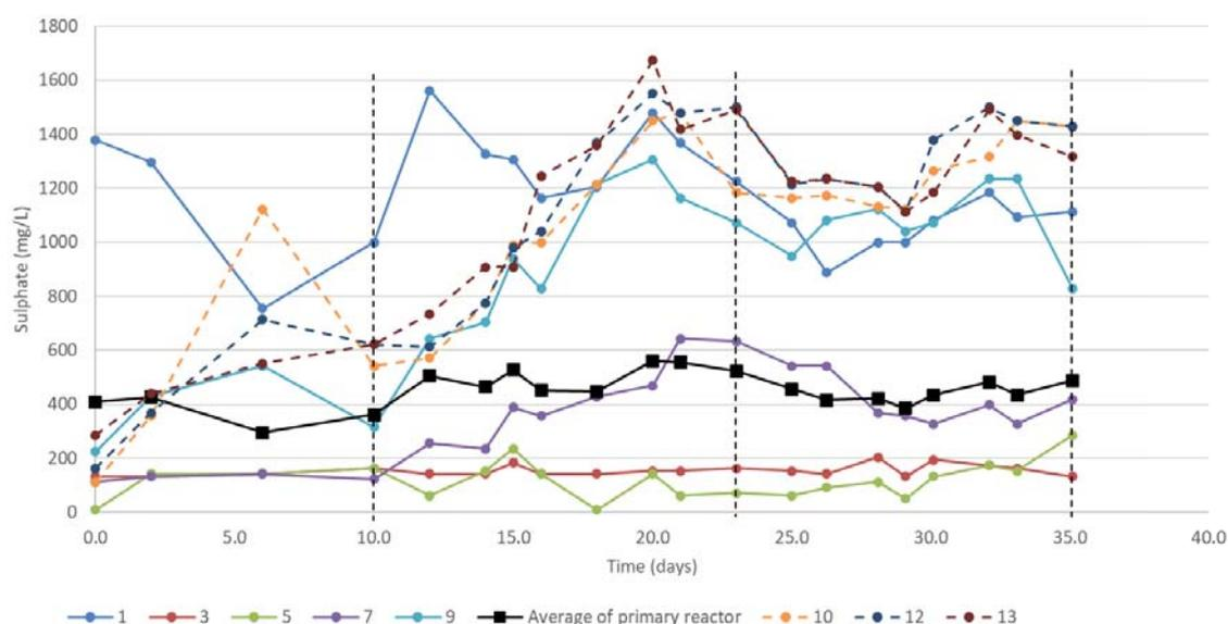
Figure 6-14: Sulphate time trends for 8 L LFCR system fed with pretreated AMD and molasses.
