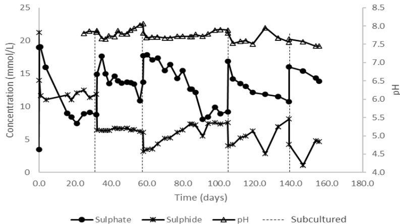
Figure 5-3: Acetate batch reactor sulphate concentration, sulphide concentration and pH time trends.
