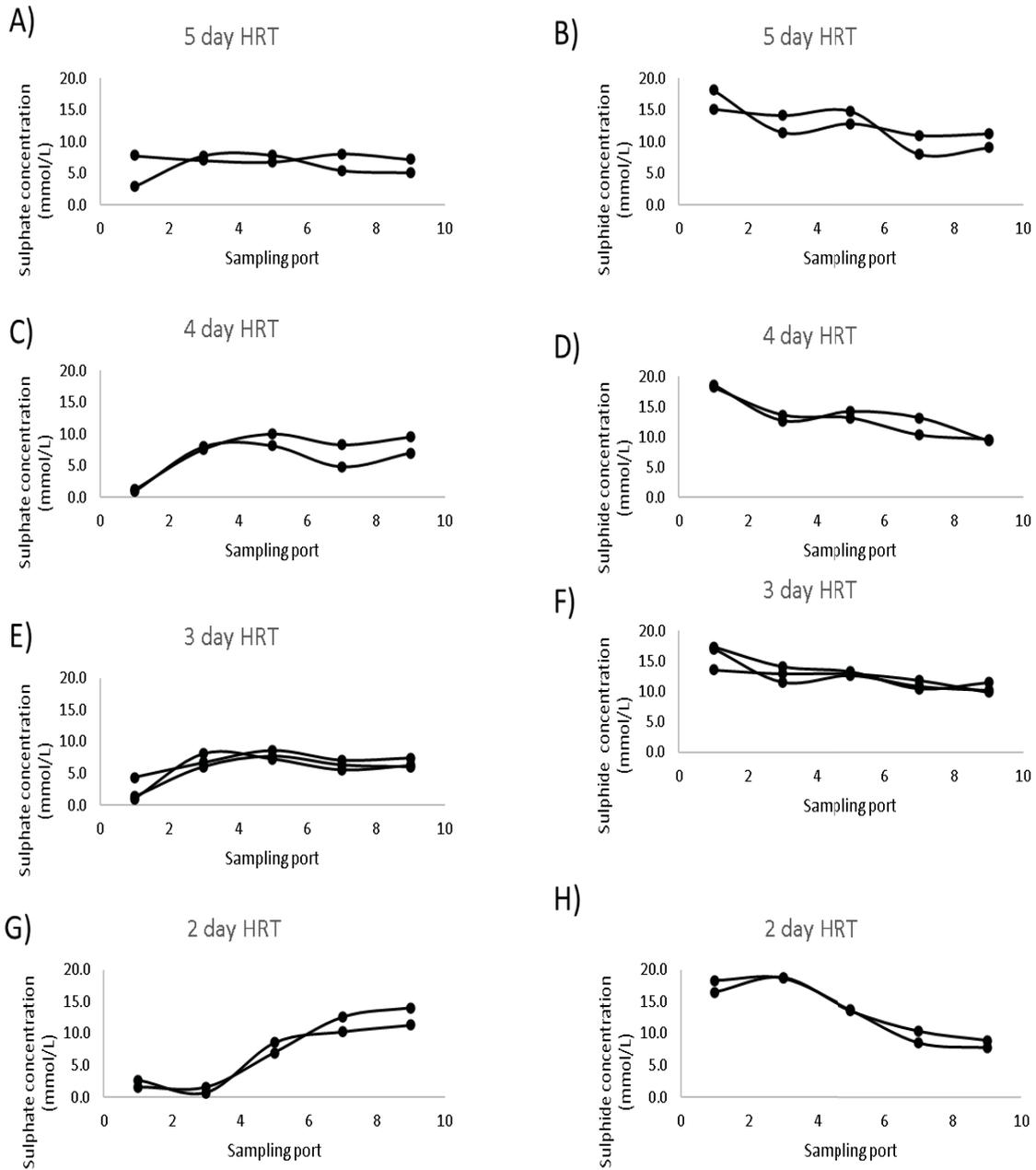
Figure 4-16: Residual sulphate (A, C, E, G) and dissolved sulphide (B, D, F, H) concentration profile across the baffled reactor sampling ports (1-9). Each data series represents a time point (day) of sampling.
