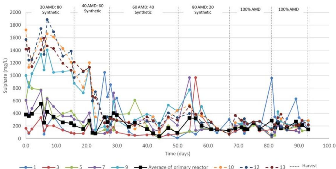
Figure 6-6: Sulphate time trends in the 8 L LFCR system with stepwise increases in real AMD, and lactate as electron donor.
