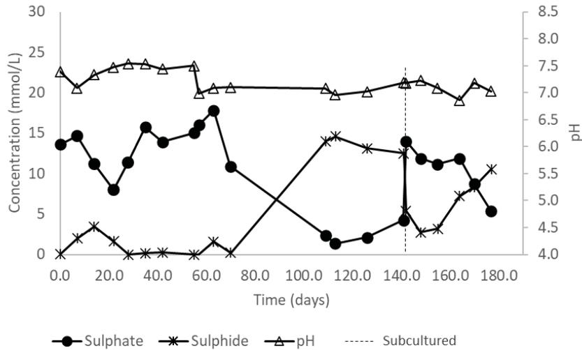
Figure 6-2: Pretreated with lime AMD batch reactor sulphate concentration, sulphide concentration and pH time trends
