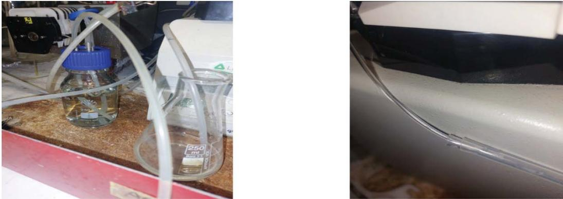
Figure 5-12: Feed and feed tubing dissolved oxygen tests using resazurin during continuous operation.
