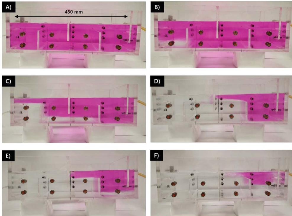
Figure 4-4: Dye tracer study showing photographic images on the progression of mixing over time in the baffled reactor operated at a flow rate equivalent to a 12 h HRT, photographs taken at A) 0 min B) 9 min C) 1 h 15 min D) 2 h 21 min E) 2 h 29 min F) 2 h 57 min.
