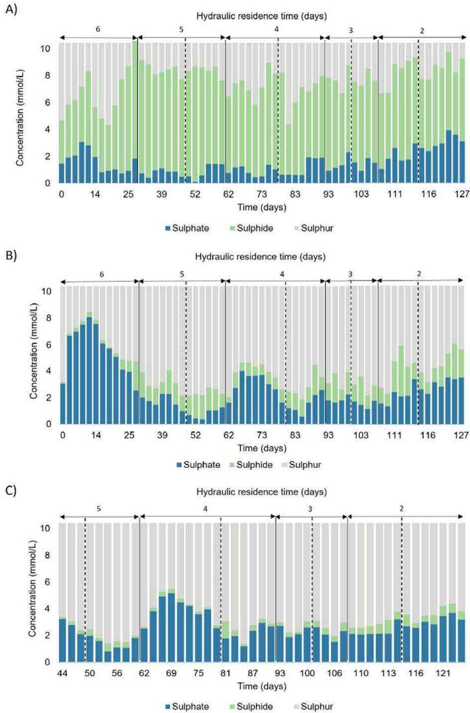
Figure 4-7: Effect of HRT on process performance showing measured residual sulphate and dissolved sulphide concentration over time in the A) primary reactor B) secondary reactor C) clarifier. Elemental sulphur is assumed to be the main product of sulphide oxidation and was determined based on the sulphur mass balance and unaccounted fraction. Solid and vertical lines define the FSB harvesting regime.
