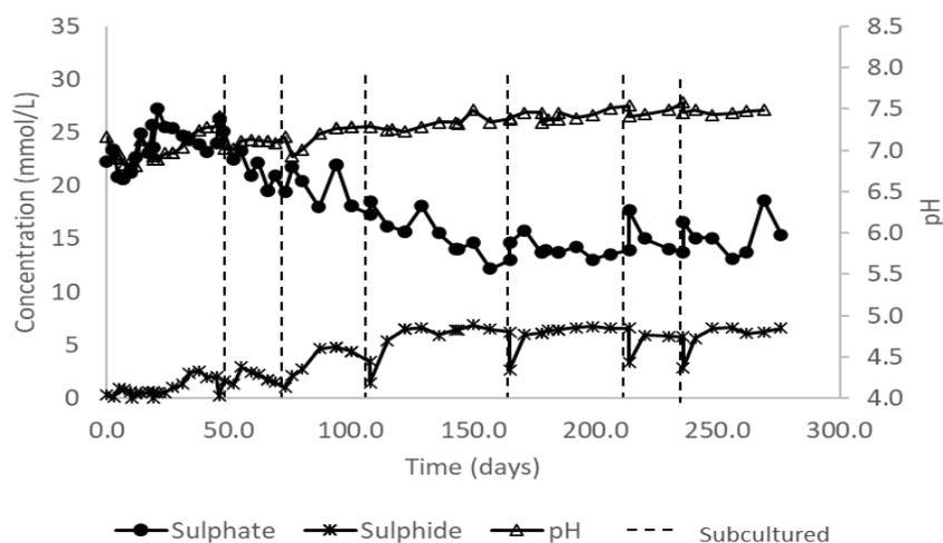
Figure 5-5: Algal lysate reactor sulphate concentration, sulphide concentration and pH time trends.
