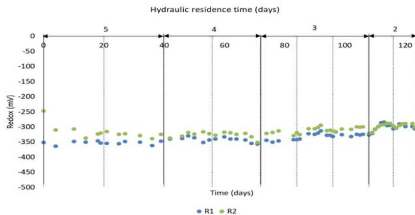
Figure 4-15: Effect of HRT on the redox potential profile within the effluent samples taken from the primary and secondary reactors. Solid and broken vertical lines define the FSB harvesting regime.
