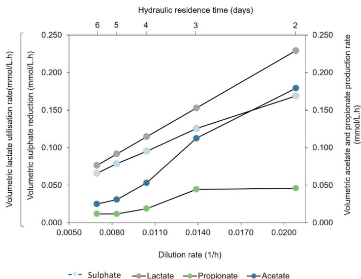
Figure 4-10: Effect of HRT on reaction kinetics showing the volumetric sulphate reduction rate, lactate utilisation rates and acetate/propionate production rates.
