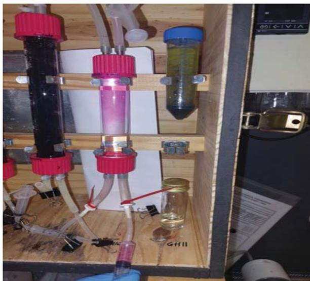
Figure 5-14: Mini-column dissolved oxygen test using resazurin during continuous operation (while mimicking sampling).
