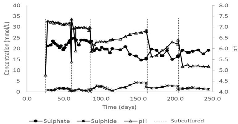
Figure 5-4: Honey batch reactor sulphate concentration, sulphide concentration and pH time trends.
