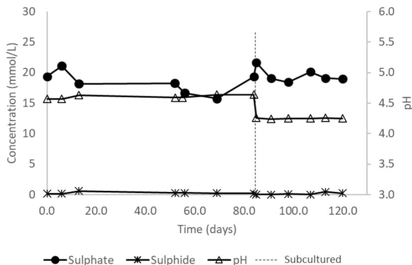
Figure 6-1: Untreated AMD batch reactor sulphate concentration, sulphide concentration and pH time trends
