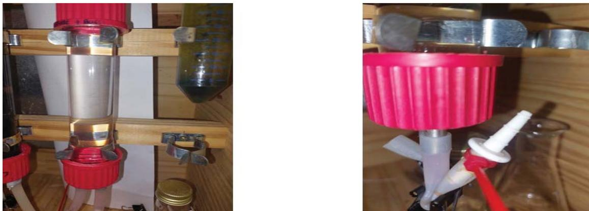
Figure 5-11: Mini-column dissolved oxygen tests using resazurin while on batch mode at room temperature.
