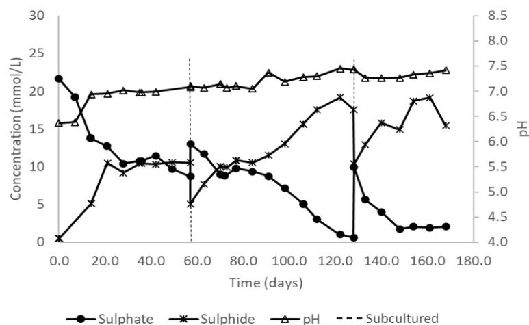
Figure 5-6: Lactate batch reactor sulphate concentration, sulphide concentration and pH time trends.
