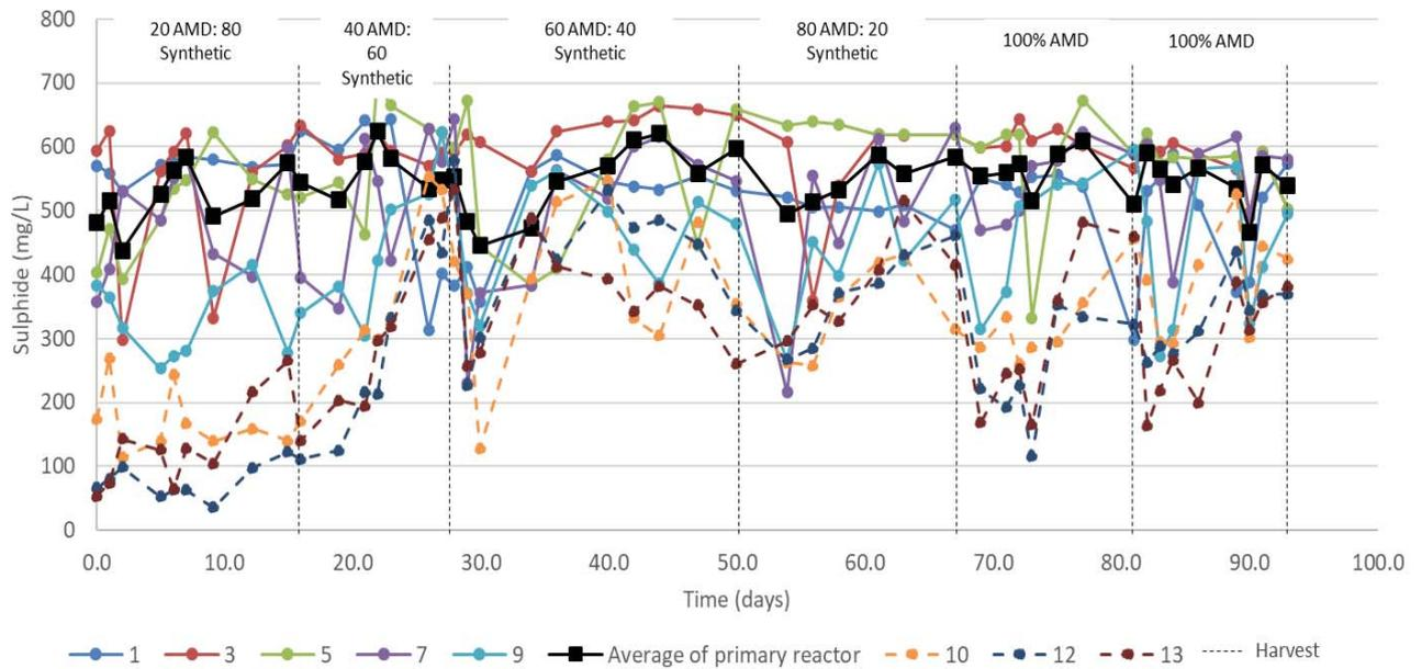
Figure 6-7: Sulphide time trends in the 8 L LFCR system with stepwise increases in real AMD, and lactate as electron donor.
