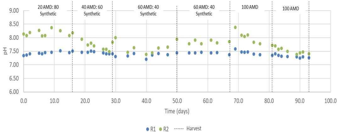
Figure 6-9: pH time trends in 8 L LFCR system with stepwise increases in real AMD, and lactate as electron donor.
