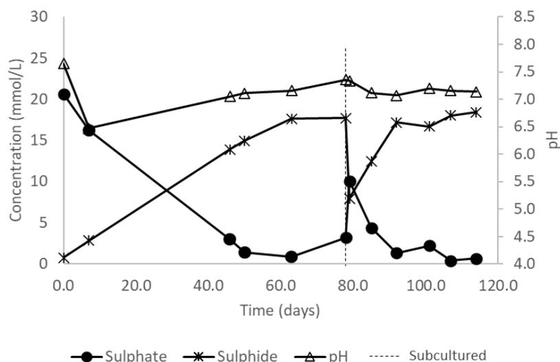
Figure 6-4: Pretreated with lime and sterilised AMD batch reactor sulphate concentration, sulphide concentration and pH time trends
