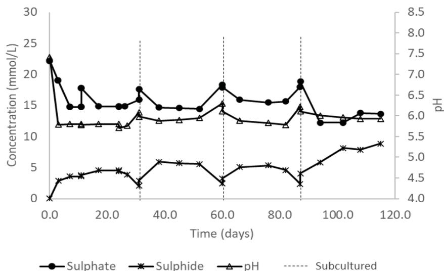
Figure 5-7: Ethanol batch reactor sulphate concentration, sulphide concentration and pH time trends.
