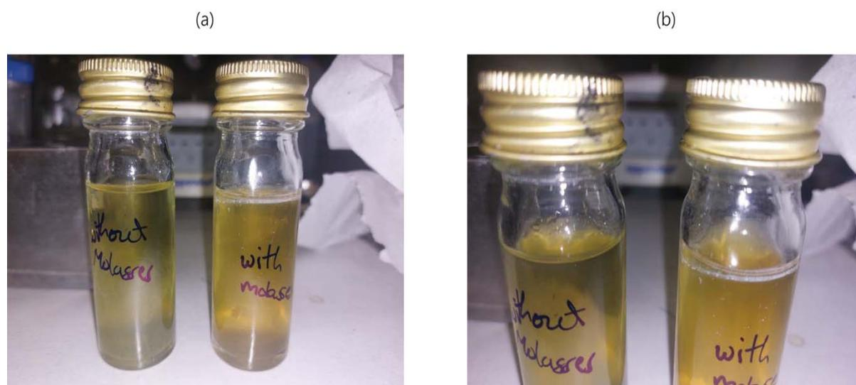
Figure 6-19: Testing for FSB formation when additional carbon source is added to a seemingly carbon depleted SRB system which cannot form an FSB: (a) full view and (b) close-up view
