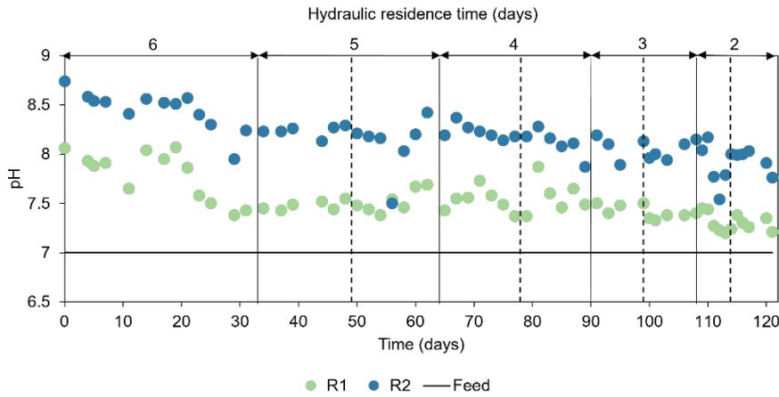
Figure 4-8: Effect of HRT on pH profile within the effluent samples taken from the primary and secondary reactors. Solid and vertical lines define the FSB harvesting regime.
