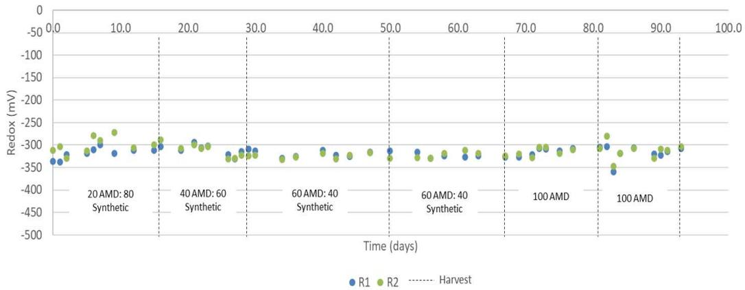
Figure 6-8: Redox time trends in the 8 L LFCR system with stepwise increases in real AMD, and lactate as electron donor.
