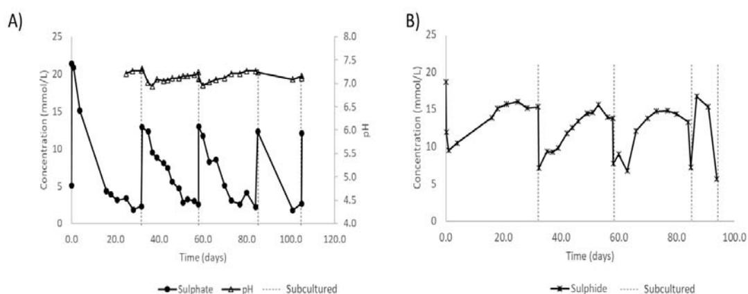
Figure 5-2: Molasses batch reactor A) sulphate concentration and pH time trends B) sulphide concentration time trend.
