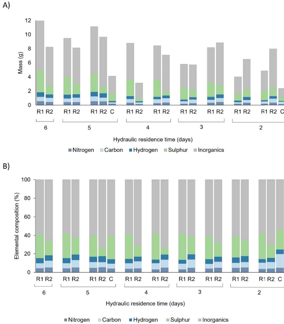
Figure 4-12: Effect of HRT on biofilm harvest and elemental sulphur recovery showing A) total harvested FSB B) elemental composition (%) in the primary and secondary reactors as well as the clarifier.
