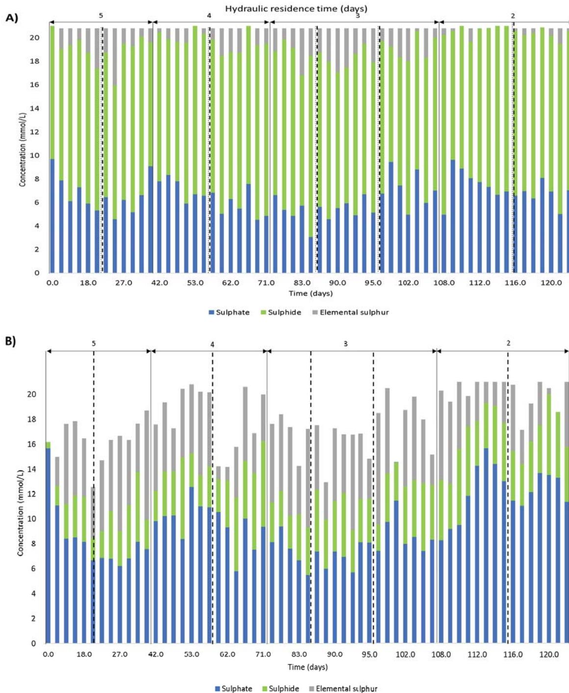
Figure 4-13: Effect of HRT on process performance showing measured residual sulphate and dissolved sulphide concentration over time in the A) primary reactor B) secondary reactor. Elemental sulphur is assumed to be the main product of sulphide oxidation and was determined based on the sulphur mass balance and unaccounted fraction. Solid vertical lines define the FSB harvesting regime.
