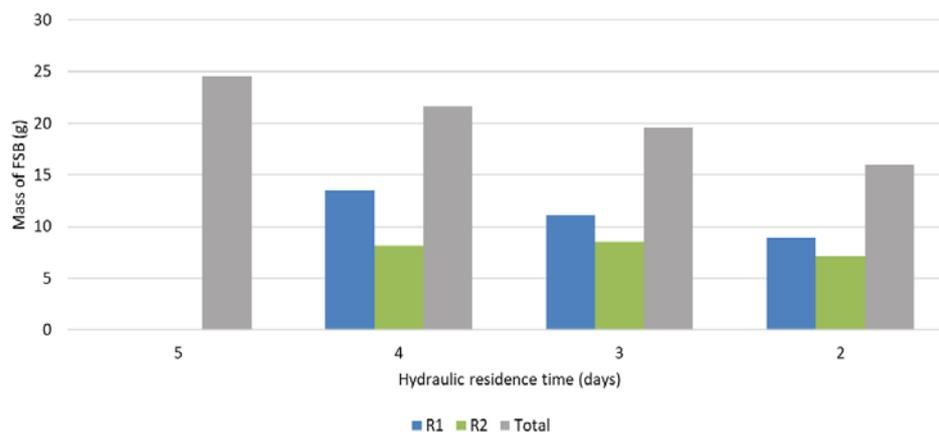
Figure 4-17: Effect of HRT on the biofilm harvest in the primary and secondary reactors.
