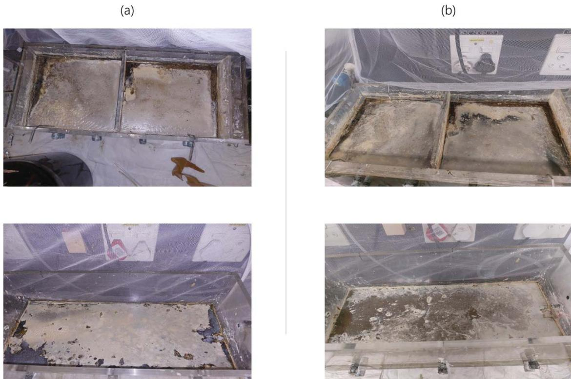
Figure 6-18: Top view of the primary (top) and secondary (bottom) reactor running on pretreated AMD and molasses, showing (a) the first run FSB formation (b) the second run FSB formation.
