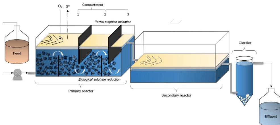
Figure 4-6: Hybrid baffled reactor configuration with the addition of a secondary sulphide oxidation unit and clarifier downstream for enhance sulphur recovery.
