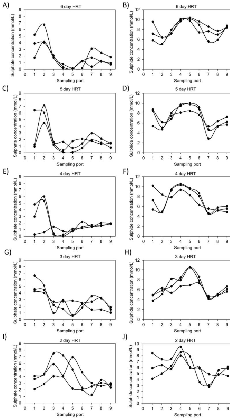
Figure 4-11: Residual sulphate (A, C, E, G, I) and dissolved sulphide (B, D, F, H, J) concentration profile across the baffled reactor sampling ports (1-9). Each data series represents a time point (day) of sampling.
