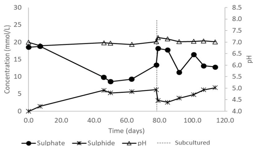
Figure 6-3: Pretreated with lime and sodium sulphide batch reactor sulphate concentration, sulphide concentration and pH time trends
