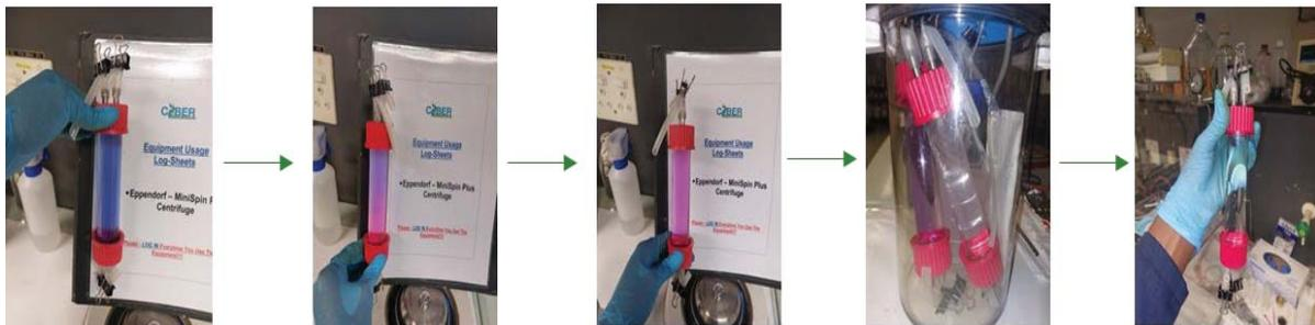
Figure 5-10: Mini-column (set-up and batch mode) dissolved oxygen test using resazurin.
