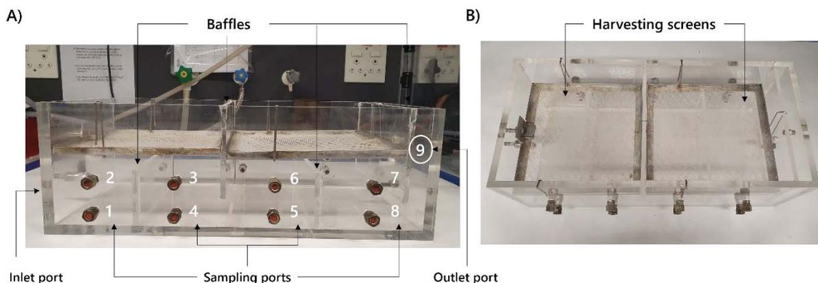
Figure 4-3: Modified hybrid baffled reactor showing A) baffles and sampling ports (1-9) positioned across the length and depth of the reactor as well as the positions of the inlet and outlet ports. B) top view of the reactor fitted with harvesting screens for FSB recovery
