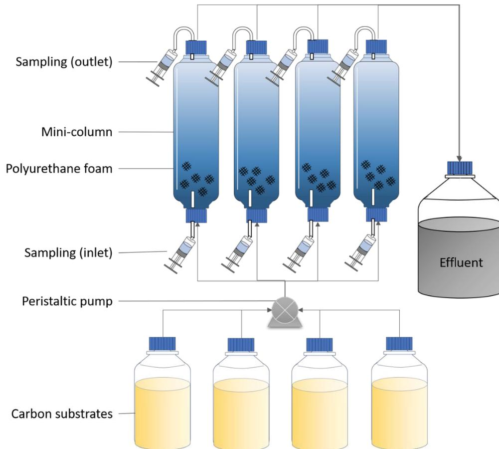
Figure 5-1: Mini-column bioreactor set-up used to evaluate selection of carbon sources (simple and complex).
