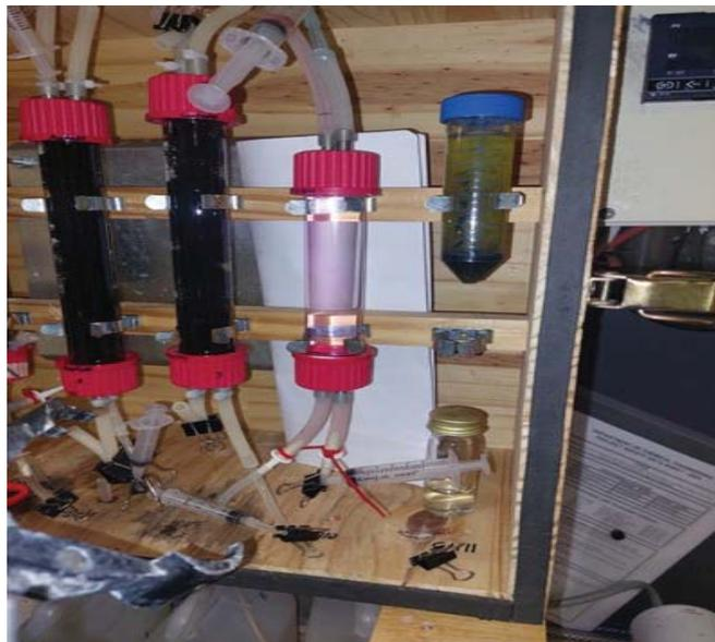
Figure 5-13: Mini-column dissolved oxygen test using resazurin during the startup of continuous operation.
