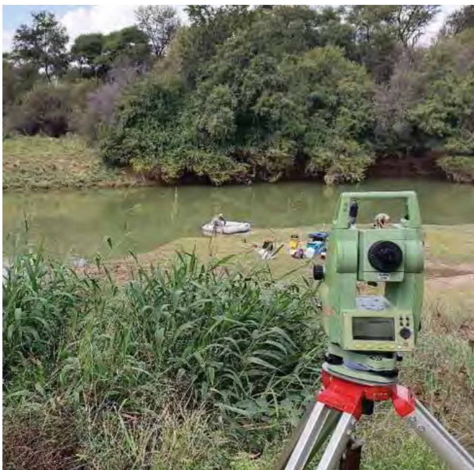
Figure 3-29: Survey setup – Leica Tcr403 power total station on tripod.
