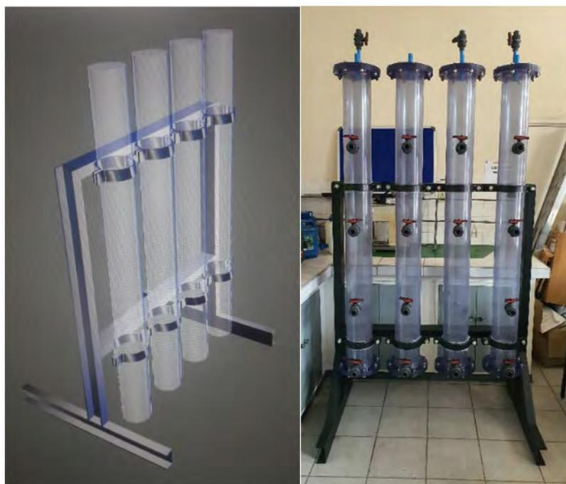
Figure 4-1: Pilot Scale Adsorption Column Rig before Installation at BNR Activated Sludge Case Study Plant
