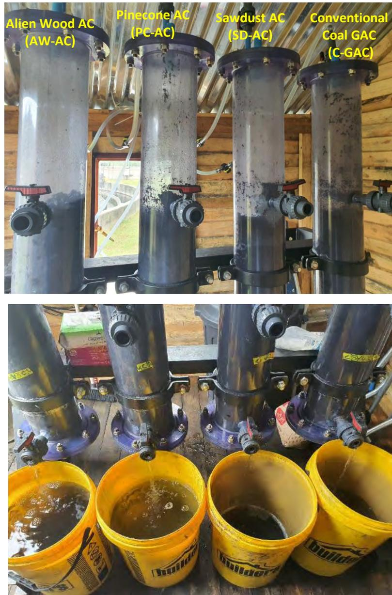
Figure 5-20: Pilot Scale Column Test Calibration for the Various ACs. After washing off fines, soaking and removing floating particles, the AW-AC and PC-AC column beds remained intact similar to GAC.
