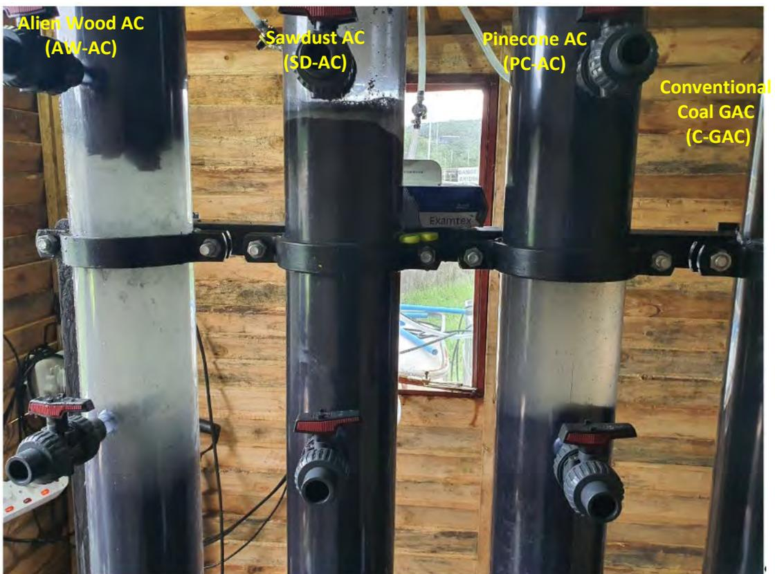
Figure 5-19: Pilot Scale Column Test Calibration for the Various ACs. AW-AC and PC-AC had broken beds with some particles floating to the surface while wastewater could not flow through SD-AC causing pooling in the column. C-GAC had a normal bed.
