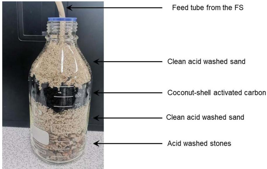
**Figure 3.2:** Pre-treatment with sand filtration and coconut-shell activated carbon.
